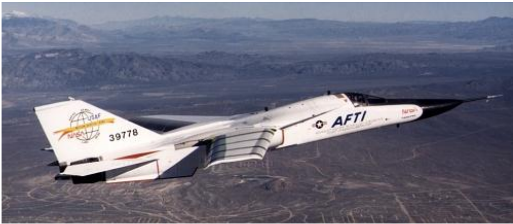
Figure 4: AFTI F-111 Mission Adaptive Wing (MAW) in flight [19].
