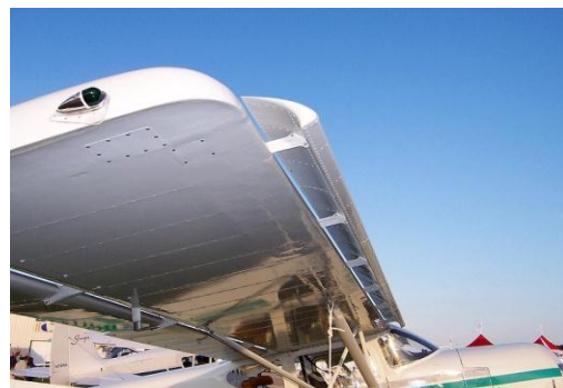
Figure 6: STOL aircraft with a fix slot [11].
