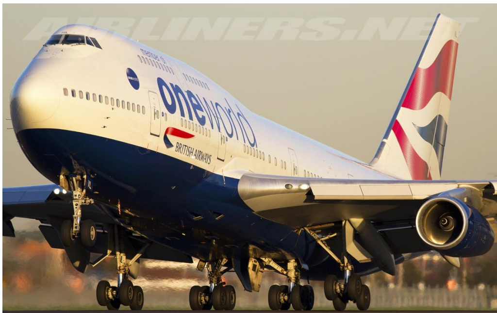
Figure 10: Boeing 747 equipped with bull nose Krueger flaps in the inboard section and variable camber Krueger flaps on the outboard section [20].
