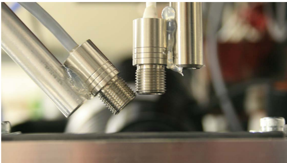
Figure 4.11: Side-on image of an example pyrometer configuration, in this case on a SiC square substrate. The pyrometers observed are both imaging the laser incidence zone, with one 45° angled pyrometer and the other at 15mm standoff perpendicular to the substrate surface.
