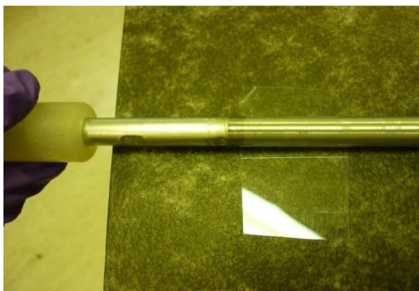
Figure 3.6 Meyer rod coating setup for Ag NW coating on plastic substrate
