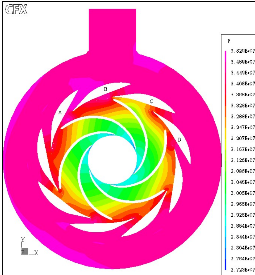
Figure 3.13: Delivery model pressure plot - impeller blade aligned with diffuser C ( N/m^2 )
