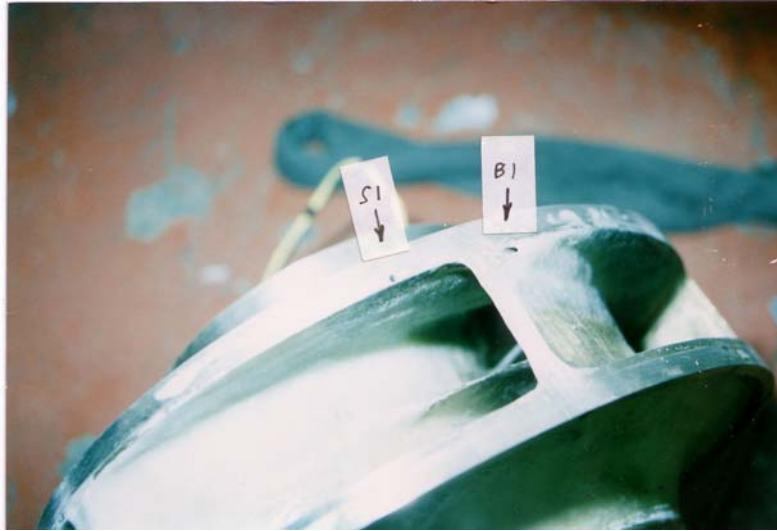
Figure 4.5a: Photograph of an inline impeller (blade B1 and shroud S1 transducer positions labelled)
