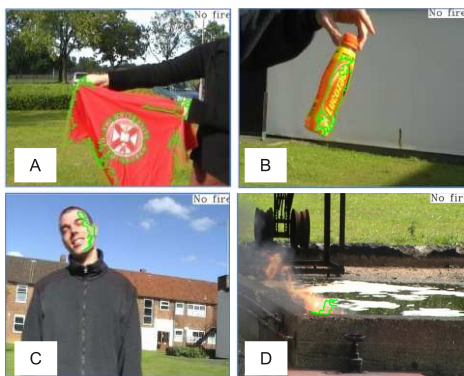
Fig. 7. Successful non-fire detection (A-C) and false negative example (D)
