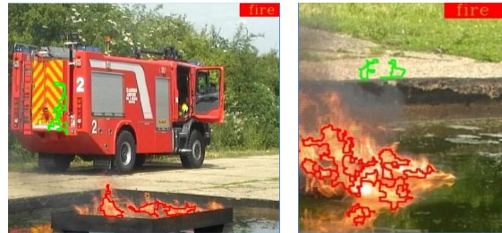
Fig. 4. Fire pixels regions detected using 2-stage colour spectroscopy and decision tree classification (red), single-stage colour spectroscopy only (green)
