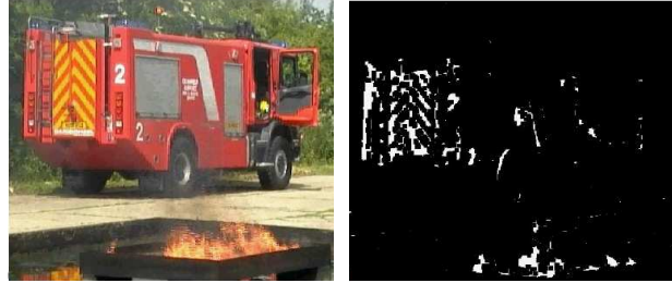
Fig. 3. Original image (left) and corresponding fire pixels regions detected using colour spectroscopy (right).
