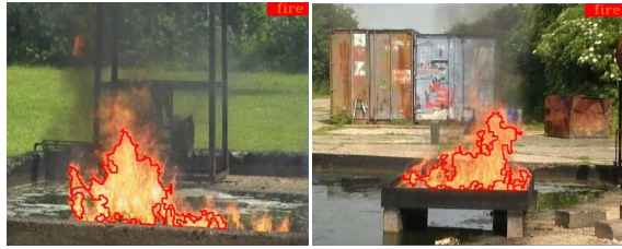
Fig. 5. Fire pixels regions detected using neural network classification (red)
