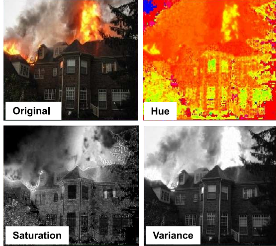
Fig. 1. Example of fire image separated into HSV colour channels (H with false colour added)
