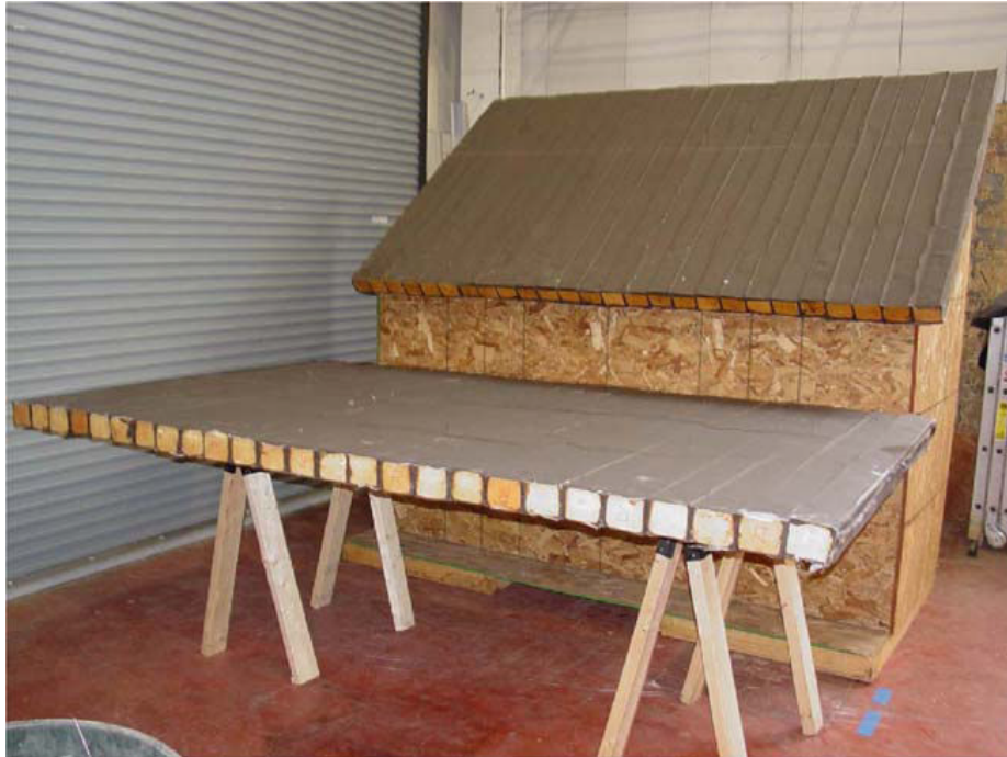
Fig. 14 Bio-based composite roof panels; one of them is mounted on a demonstration house made of timber [183]
