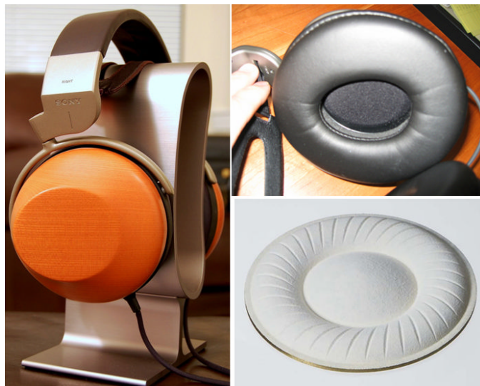
Fig. 17 Nanocellulose diaphragm used in SONY® headphones
