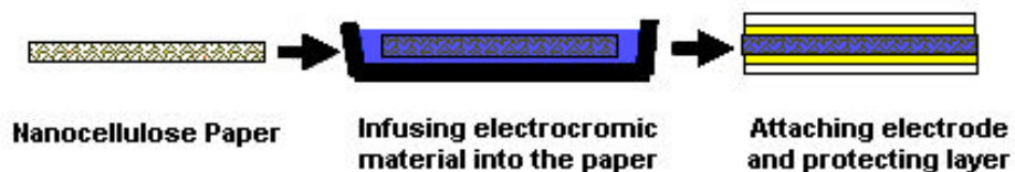
Fig. 18 Fabrication process of the display using nanocellulose
