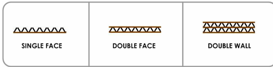
Figure 4.2: Cardboard Sheet Configuration
