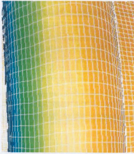
Figure 6.18: Static Pressure Distribution around the Bellmouth Lip
