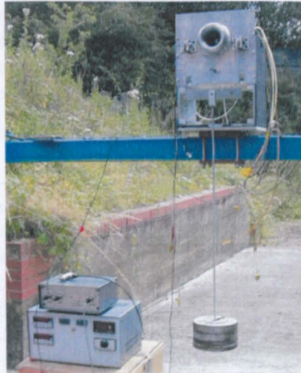
Figure B.7: Outdoor Load Cell Calibration
