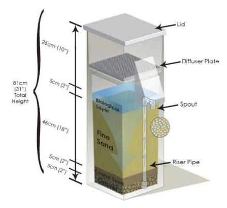
Figure 9: Measurements for media and specification of parts.
