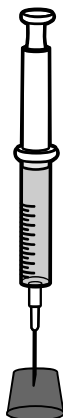
Scheme 6-4: Syringe, needle, cork and plunger used to measure the swelling of the polymers
