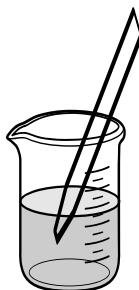
Scheme 6-1: Immersion of a Pasteur pipette into the solution to degas it with an inert gas
