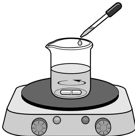
Scheme 6-2: Stirring the solvent to create a vortex and precipitate the polymer by dropping in the solution of the polymer
