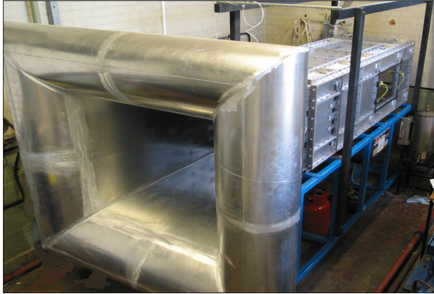
Figure 3.3 Bellmouth on test facility
