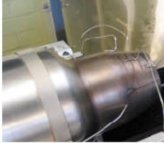
Figure 4.23 Static pressure probes on the exhaust nozzle
