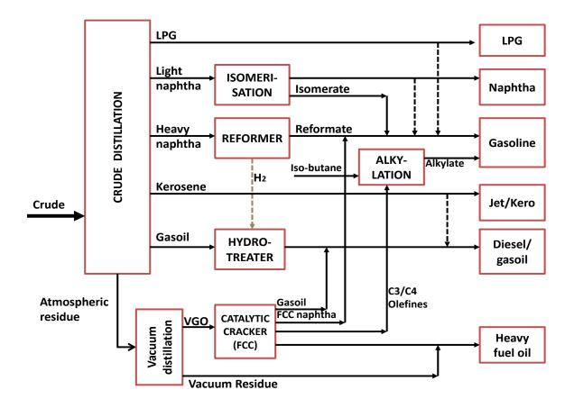
Figure 2.5 A Catalytic Cracking Refinery (Speight, 2011)
