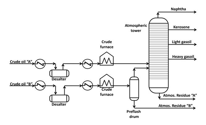
Figure 5.5 Most effective refinery scheme (Dual Drum Scheme: Hori, 2000)
