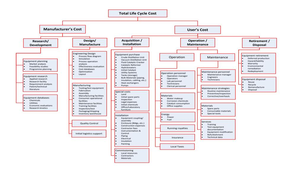
Figure 4.26 Proposed Life Cycle Cost Breakdown Structure for Oil Refineries
