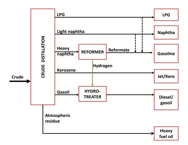
Figure 2.4 A Hydroskimming Refinery (Speight, 2011)
