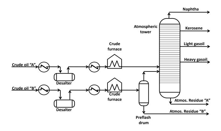
Figure 5.3 Dual Drum Scheme (Hori, 2000)
