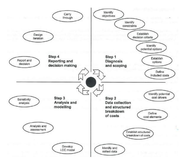
Figure 2.22 LCC Methodology for Petroleum & Natural Gas Industries (ISO 15663)
