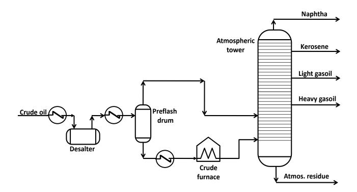
Figure 5.1 Preflash Drum Scheme (Hori, 2000)
