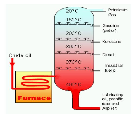
Figure 2.2 Simple Fractional Distillation (Pighadshy, 2008)
