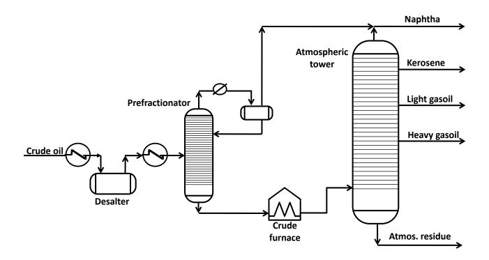
Figure 5.2 Prefractionator Scheme (Hori, 2000)
