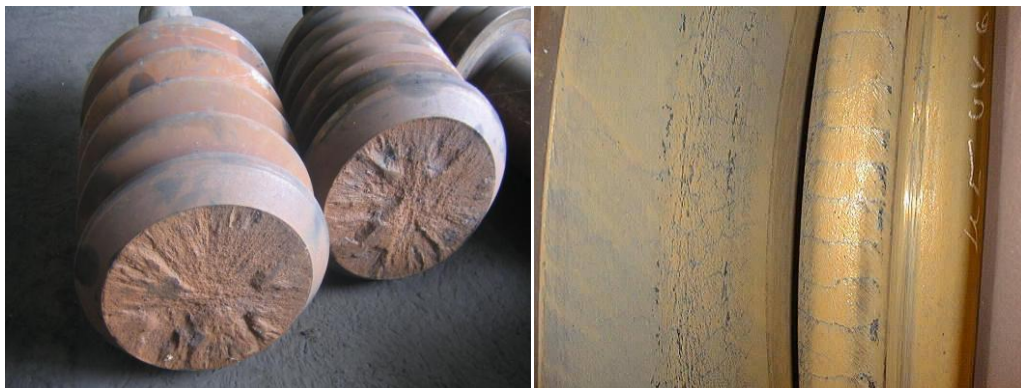
Figure 1.2. Left to right: Roll breakage due to too high temperature gradient/high residual stresses and fire cracks rolling rails (Schroeder, 2005).
