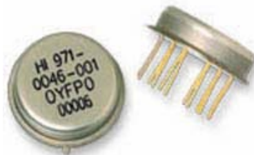
Figure 1 – The ASA7000 microaccelerometer by Colibrys
