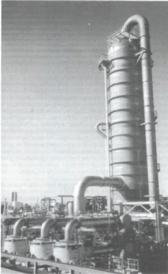
Figure 8 Three very small size RPBs equivalent to one large packed column (photo courtesy of The Dow Chemical Company)
