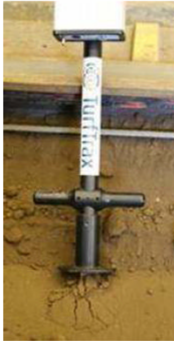
Figure 3.3: Going Stick with data logger and showing failure of soil (photograph in soil bin at Cranfield University, Silsoe courtesy of Godwin, 2006).
