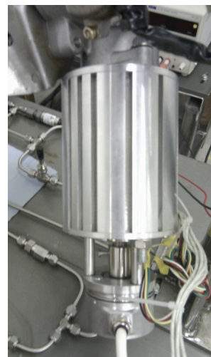
Figure A8.3 Three-phase, permanent magnet synchronous motor (right)
