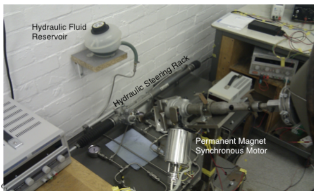
Figure A8.2 EPAS experimental apparatus (left)
