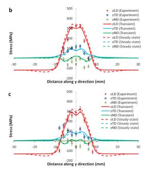
Fig. 9: Stresses in the longitudinal (LD), transverse (TD) and normal (ND) directions along a transverse line in the base-plate indicated in Fig. 2 for (a) single, (b) two, and (c) three layers.
