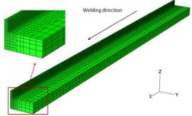
Fig. 3: Mesh of transient thermal model.
