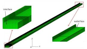
Fig. 4: Mesh of the steady state thermal model.
