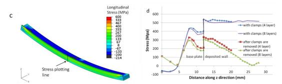
Fig. 7: Longitudinal residual stress predictions from: (a) transient thermal and mechanical models; (b) steady state thermal and mapped mechanical models; (c) steady state thermal and mapped mechanical models after clamps were removed (a scaling factor of 5 is used for the distorted shape); and (d) the stress plotted along the lines shown in of (b) and (c).
