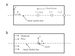
Fig. 1: Model with different reference frames. (a) Lagrangian reference frame (b) Eulerian reference frame.
