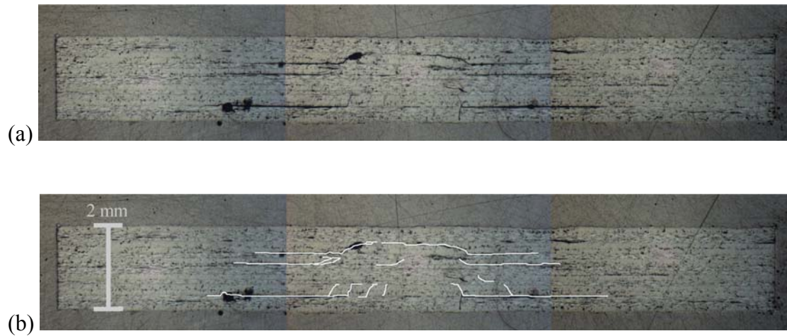
Figure B.10 Micrographs of the 5-Joule impact onto the panel DT03 with 100MPa pre-stress. (a) shows the micrograph without the delaminations highlighted and (b) shows the micrograph with the delaminations highlighted.
