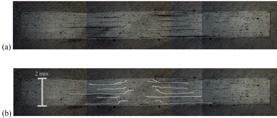
Figure B.6 Micrographs of the 5-Joule impact onto the panel DT04 with 0MPa pre-stress. (a) shows the micrograph without the delaminations highlighted and (b) shows the micrograph with the delaminations highlighted.
