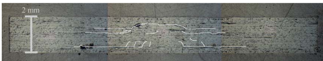
Figure 7.10 Micrograph of the damage state in a laminate pre-stressed to 100 MPa and impacted at 5 Joules in the instrumented falling weight impact tester
