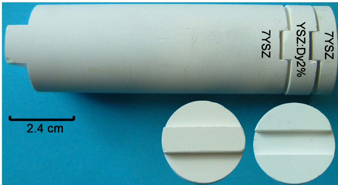
Figure 57: Multistage rod used for the multilayer coating deposition.
