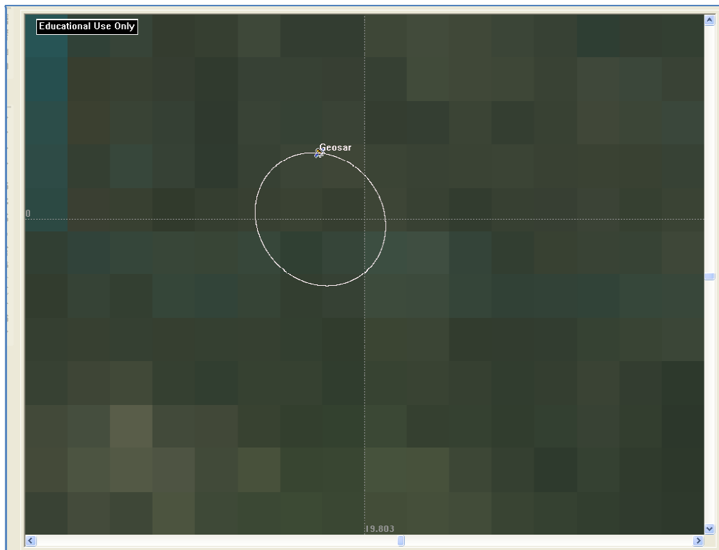
Figure 3-3. Trajectory of the satellite for a geosynchronous nearly circular orbit with non-zero inclination and non-zero eccentricity.
