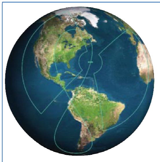
Figure 3-5. 60° geosynchronous orbit, ground track and instantaneous field of view (NASA JPL, 2003).
