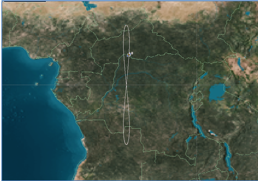
Figure 3-1. Trajectory of the satellite for a geosynchronous orbit with zero eccentricity and 5° inclination.
