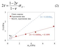
Figure 4. Variation of shear strength with impact stress.
