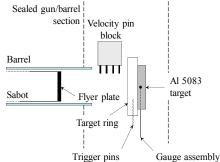
Figure 1. Lateral gauge plate-impact experimental setup.
