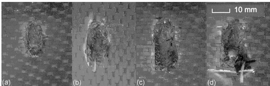
Figure 3: Penetration cavity formed after impacting the target with (a) 126 J (187 m/s), (b) 239 J (259 m/s), (c) 365 J (319 m/s), (d) 484 J (367 m/s).
