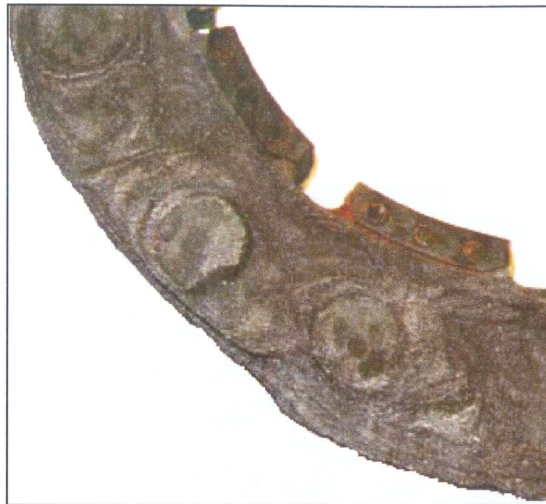
Figure 18 Catalytic Oxidation Damage (Dunlop)
