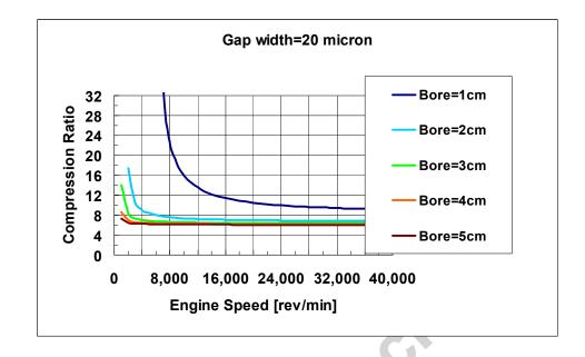
Figure 4a: Minimum compression ratio that is required to ensure ignition vs. engine speed and engine bore for a gap width of 20µm.
