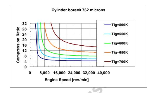
Figure 7: The effect of the fuel ignition temperature on the minimum compression ratio and minimum engine speed for a small size cylinder of 0.762cm and gap width of 5µm.
