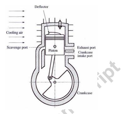
Figure 1: A schematic sketch of a simple SI crankcase-scavenged (Schnurle type) two-stroke engine<sup>18</sup>.
