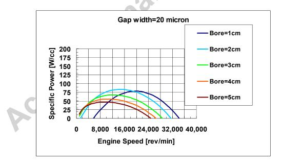
Figure 4b: The corresponding specific brake engine power.
