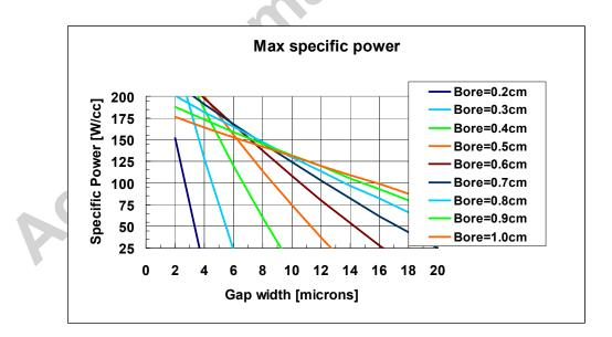
Figure 8: Maximum specific brake power vs. gap width and cylinder bore. The corresponding engine speeds are shown in Fig. 5.
