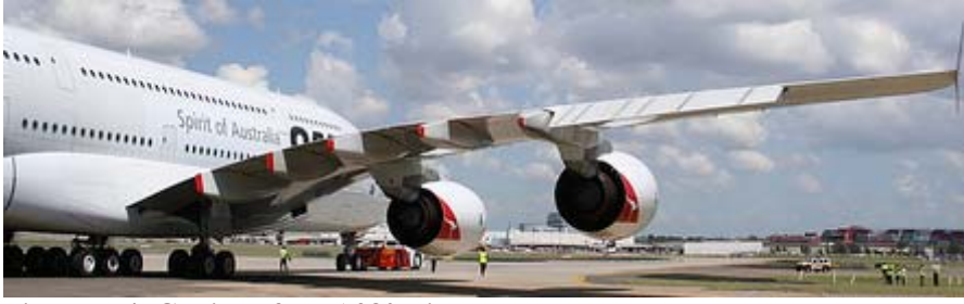
Figure D-4: Gulling of the A380 wing
