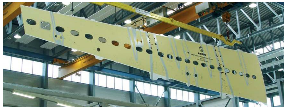
Figure 7-7: Manhole row positioned mid-chord on A400M CFRP lower cover
