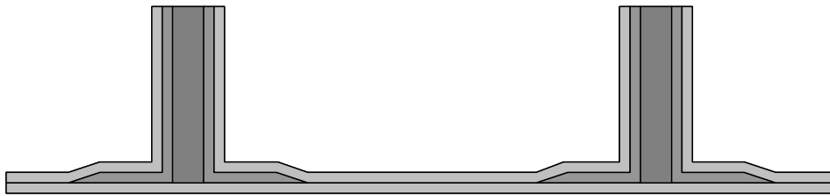
Figure 7-48: U-profile stringer concept
