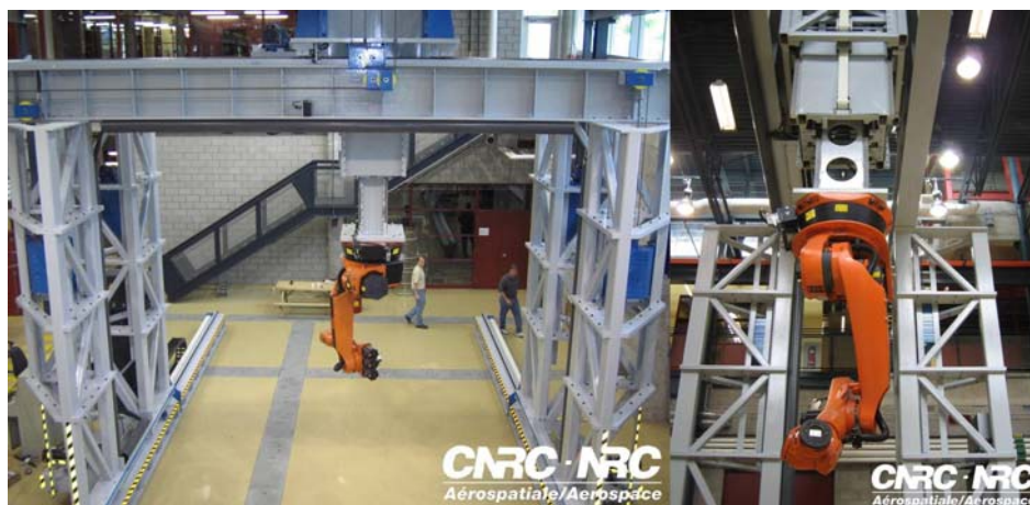
Figure 3-13: Gantry system and robotic arm
