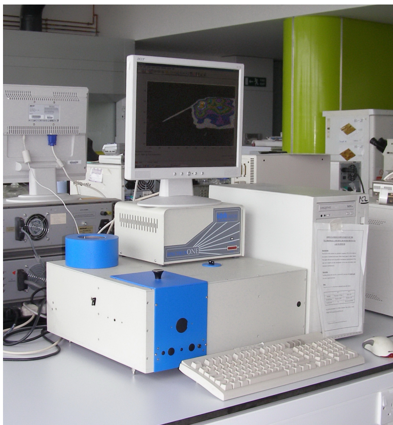
Figure 3.1: The spectrofluorometer capable of acquiring three-dimensional excitation–emission matrix (EEM) fluorescence spectra.
