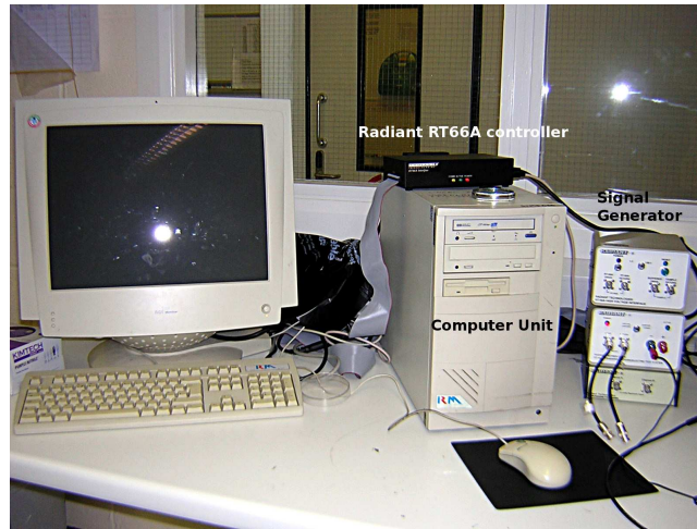
Figure 2.33: Radiant RT66A set up for ferroelectric characterization.
