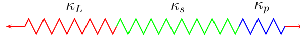
Figure 2.4: Equivalent spring constant of the load cell, the tested sample and the piezo element. The force from the extension/ contraction of the piezo is applied on the load cell and the sample.
