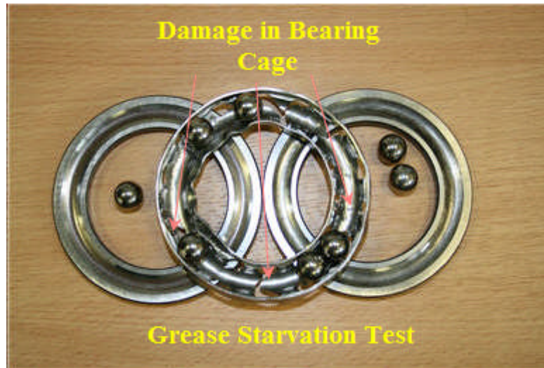
Figure 4—43 Damage on the bearing cage
