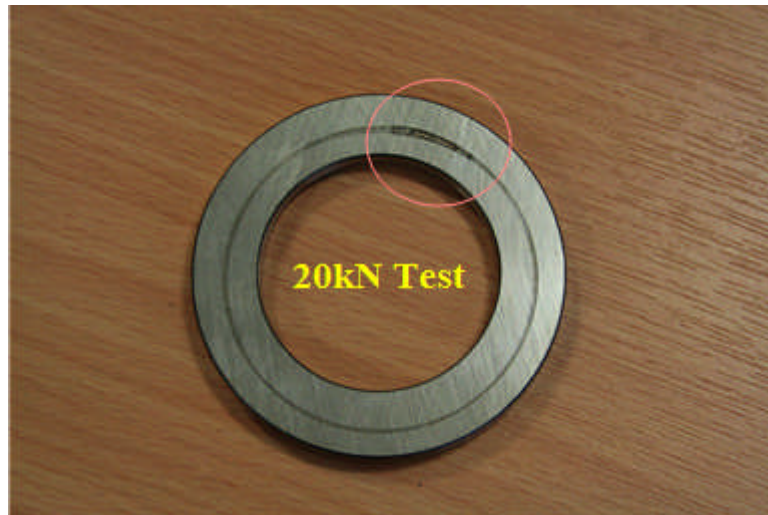
Figure 4—30 Crack zone on flat ring
