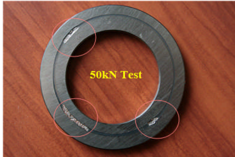
Figure 4—14 Crack zones on flat ring
