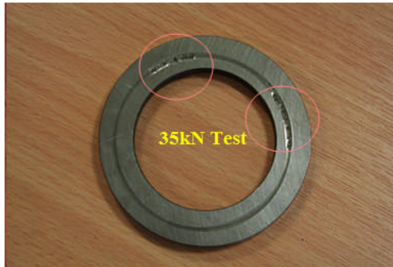
Figure 4—22 Crack zones on flat ring
