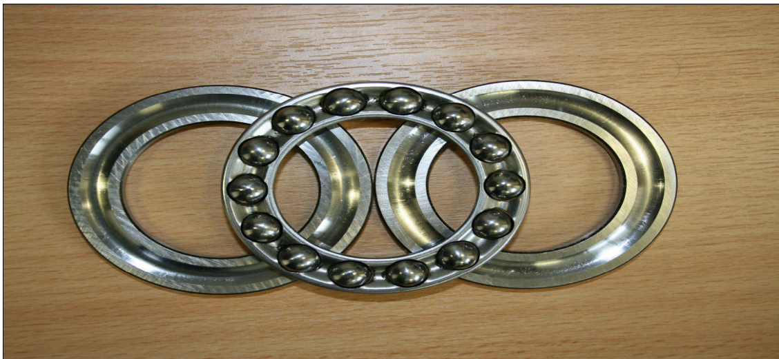
Figure 4—3 Test bearing run under starvation of grease
