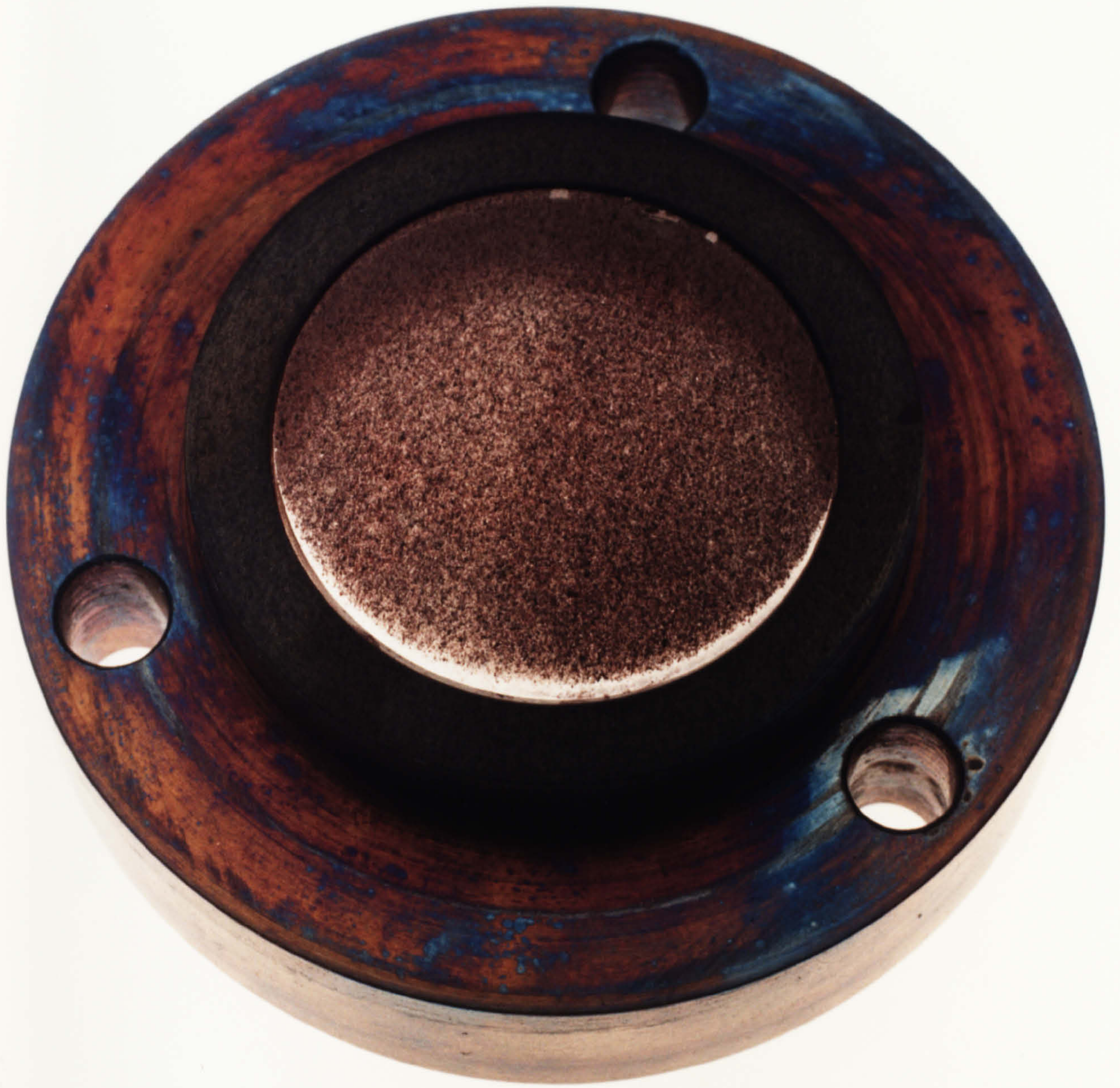
Fig. (7.2) The Quartz Window After The Test
