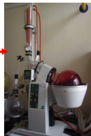
Plate 3.12. Solvent evaporation unit (Büchi Rotavapor R-200)
