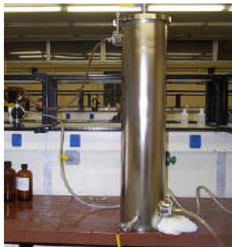
Plate 3.6. Pall bagfilter with 25 \mu\text{m} pore sizes
