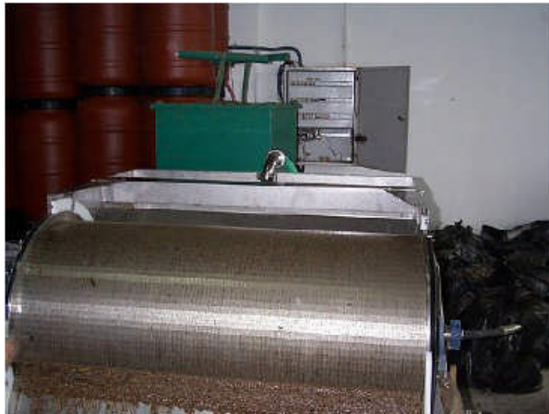
Plate 3.5. Stainless steel waterscreen rotating screen
