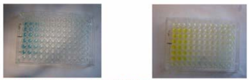
Figure 4. Microtitre plate during an ELISA assay. These images are various steps of an ELISA assay, the "blue" is the observed colour change and the "yellow" indicated the end of the reaction when stopped.
