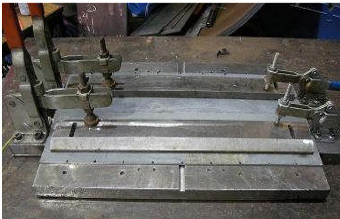
Fig. 2 Clamping arrangement for plates.
