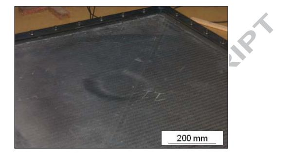
Figure 1. Slamming impact, core crushing after medicine ball impact
