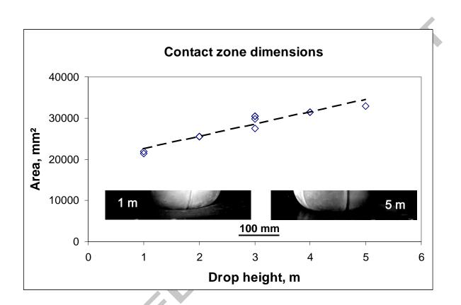
Figure 12. Influence of drop height on contact zone area. Images show ball form and correspond to maximum ball compaction for two drop heights onto pinned foam core sandwich.
