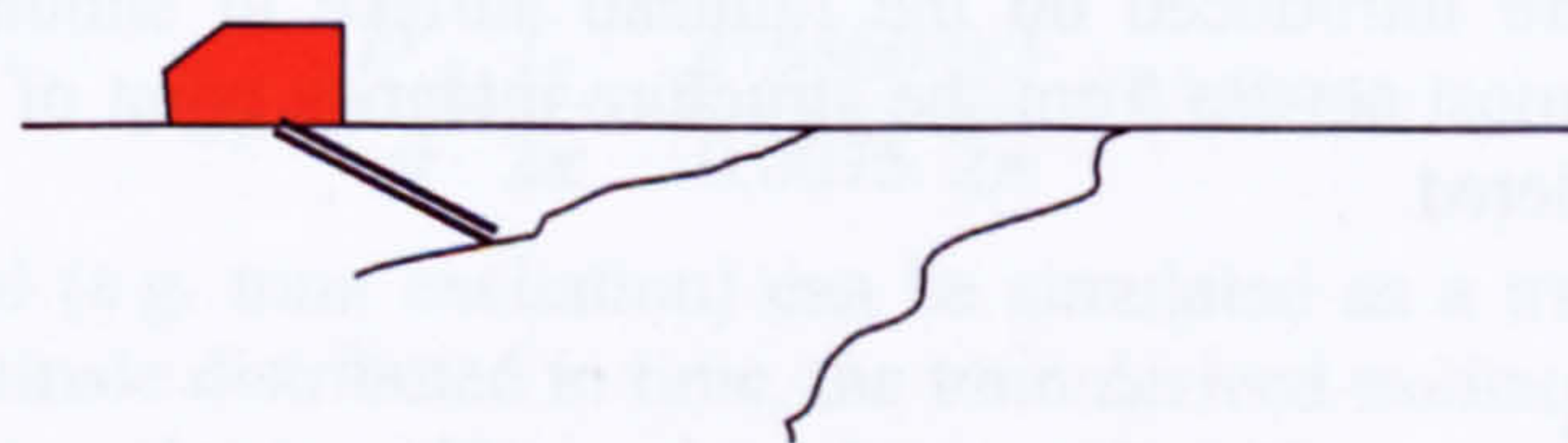
Figure 74 - Shallow crack shadowing
