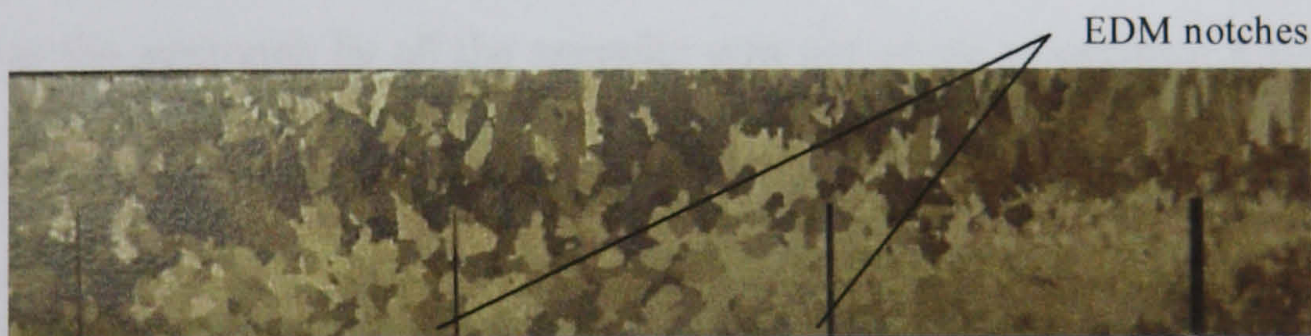
Figure 37 - Anisotropic grain structure (X 1)
