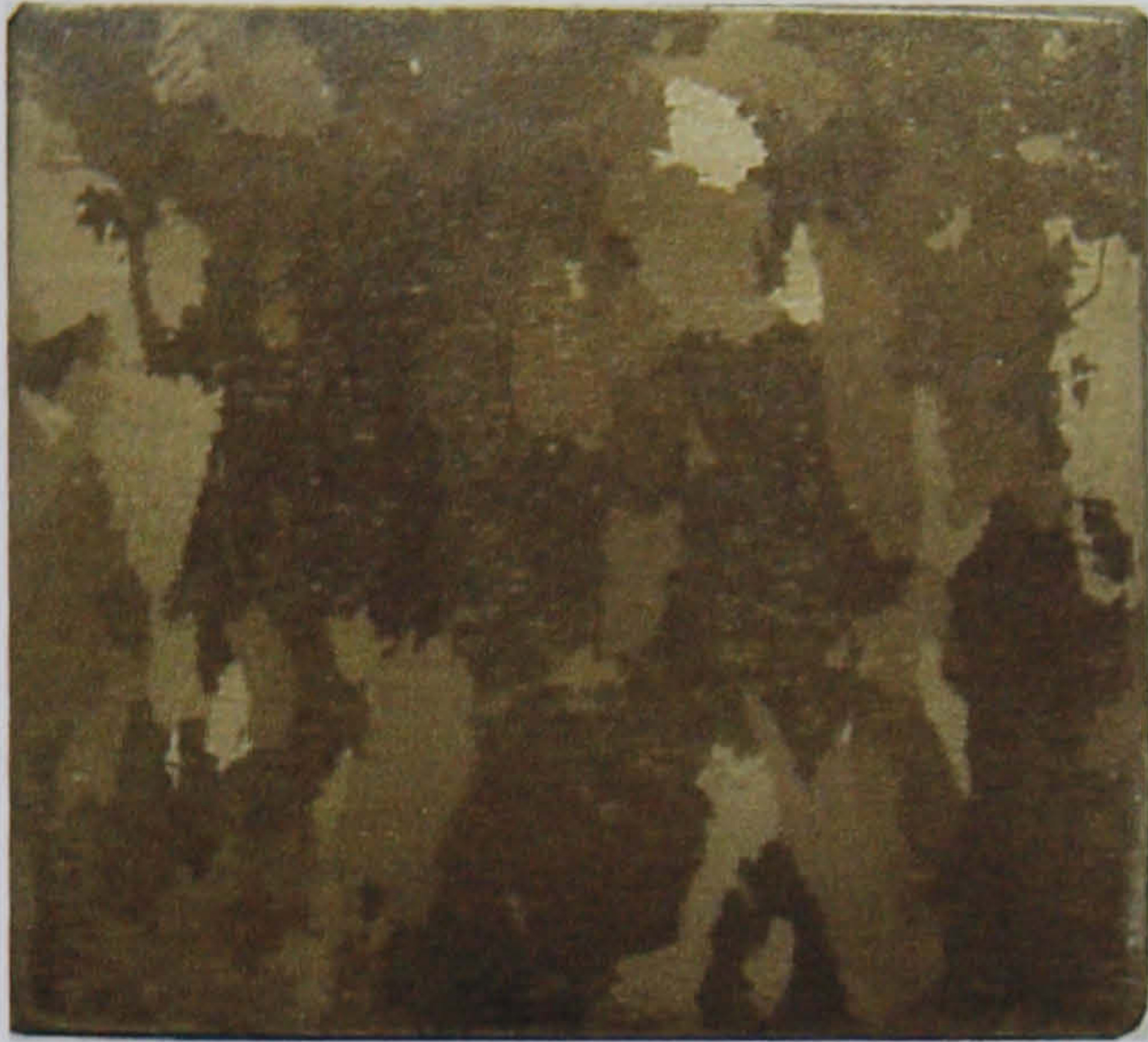
Figure 35 - Coarse grain structure - section of adapter plate.( X1.5)
