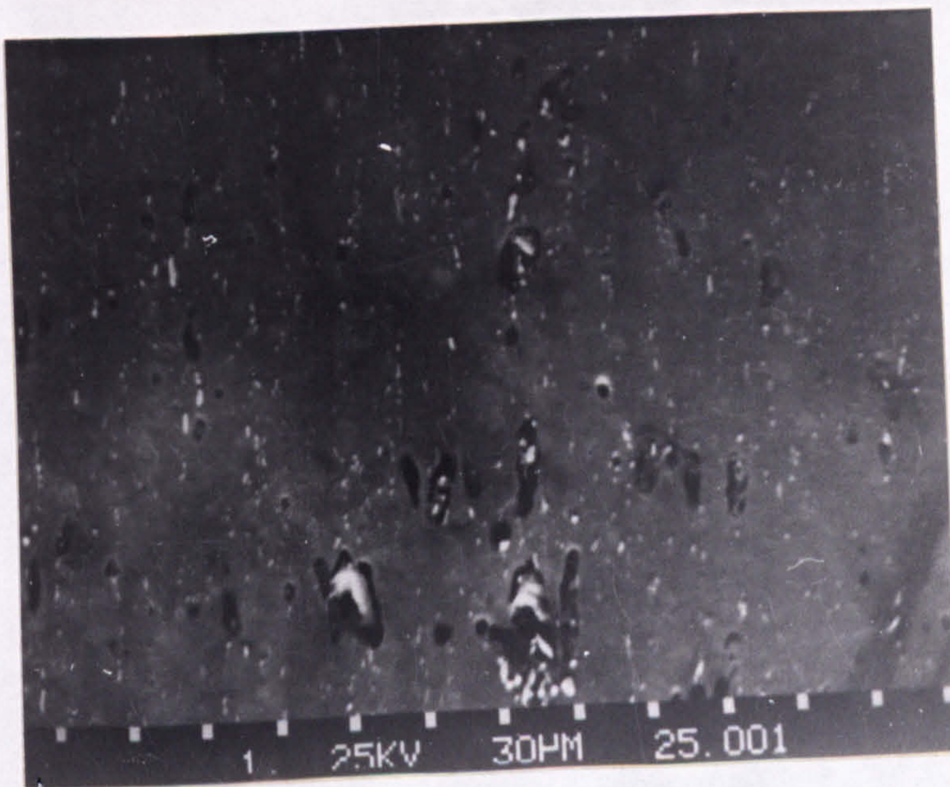
Figure 88(a)- SEM micrograph showing the nature of cavitation and distribution of precipitates in SPF and heat treated Supral 150.
