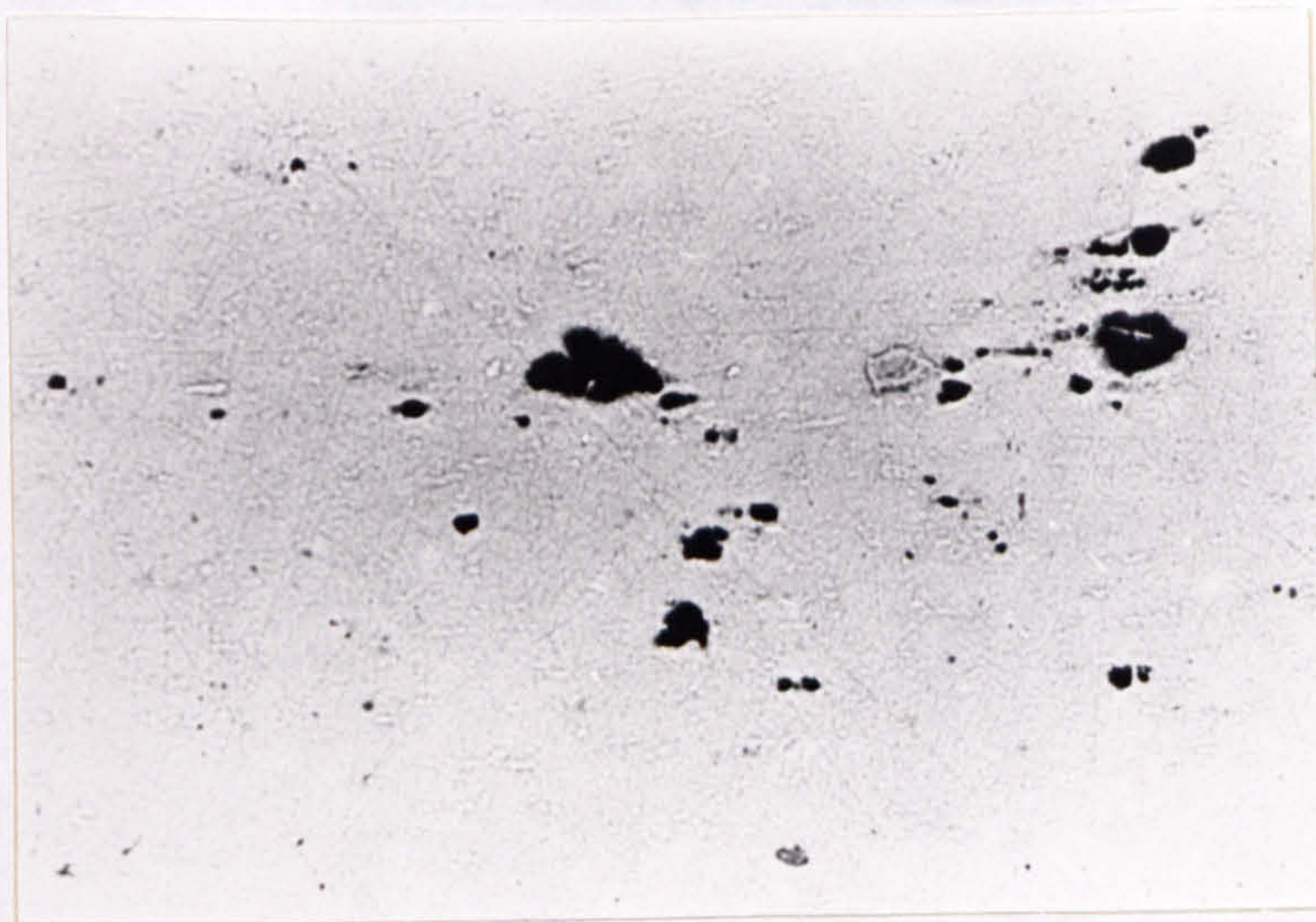
Figure 47 - Micrographs of SPF Supral 150 edge sections showing as-received SPF cavity morphology (x 75).
