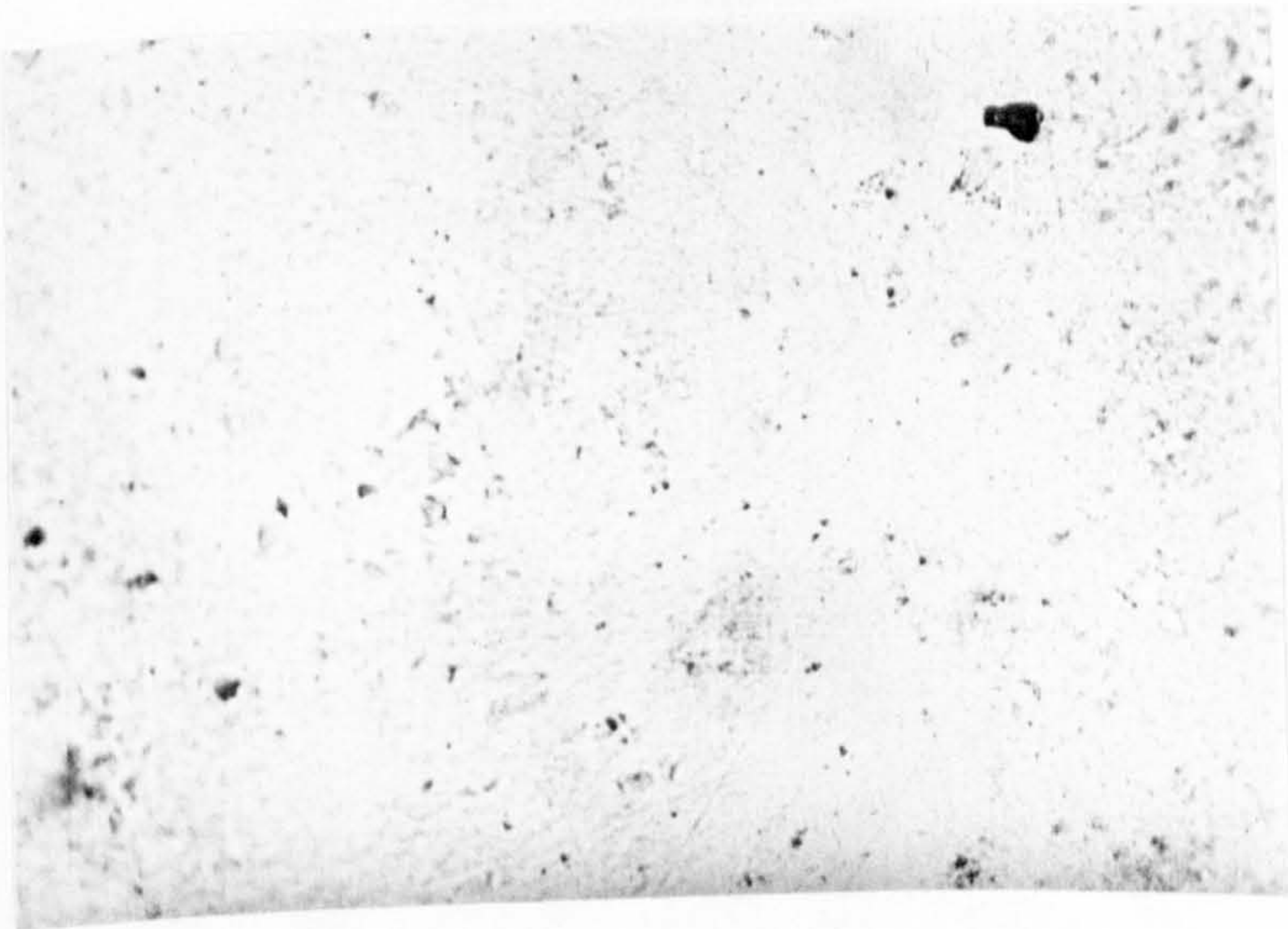
Figure 95 - Optical hot stage micrograph of SPF Supral 150 at 530°C under a vacuum at start (x 200).
