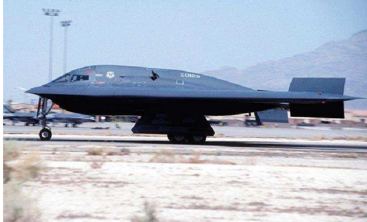
Figure 2.11: B-2 split flap rudders deployed on ground [20]
