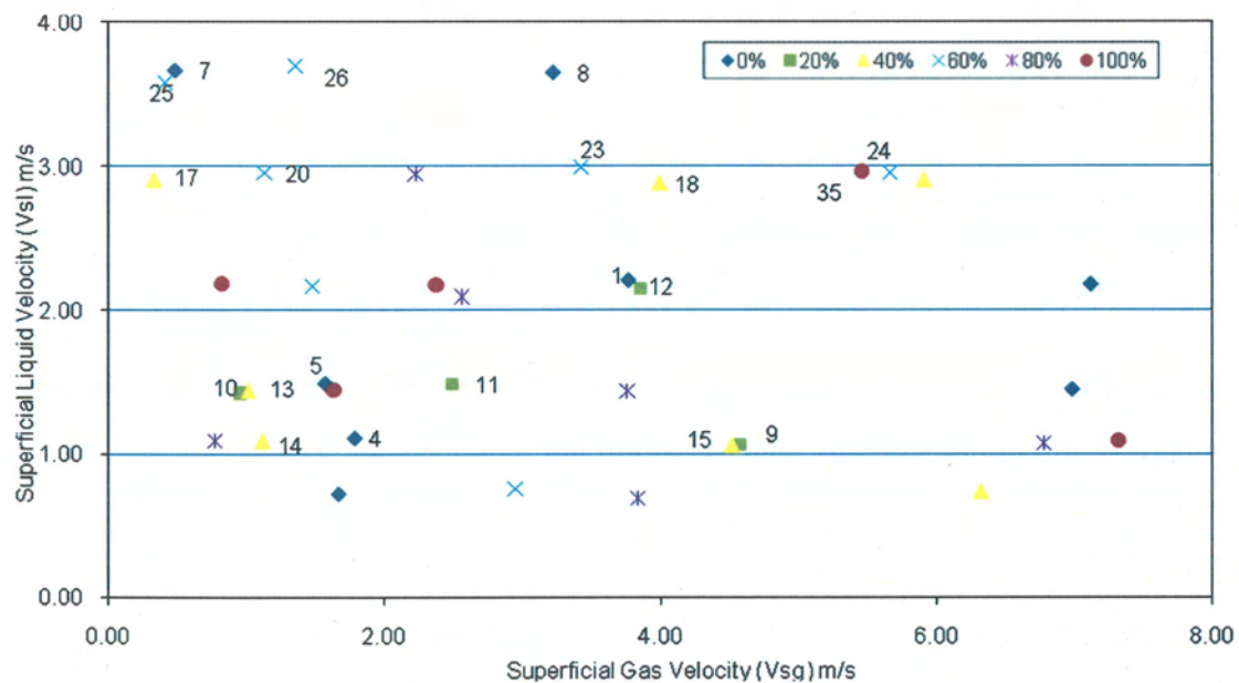
Figure 4.31 – Outlying Test Point Matrix Location for Feature Fusion Errors – Conductance 1 (Vsl Prediction)
