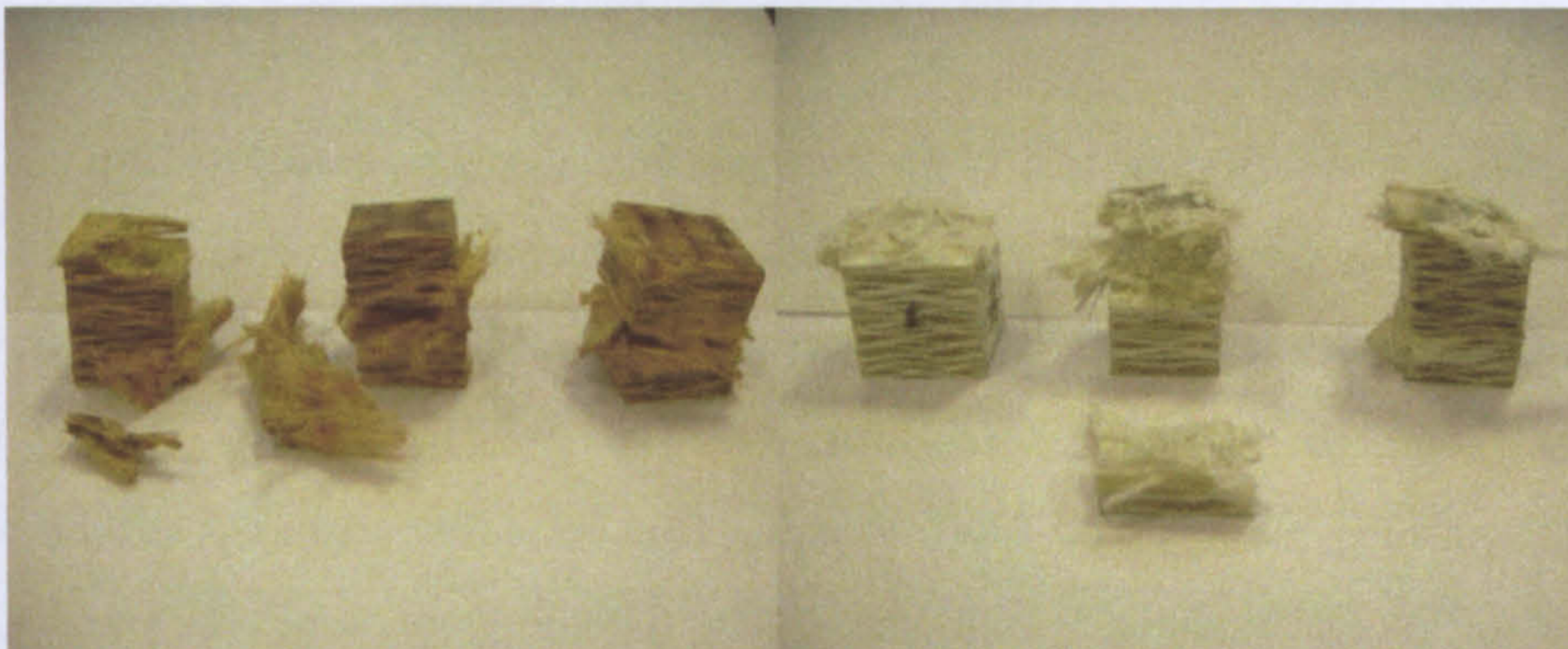
Image 4.2: Failed heavy weave samples force applied perpendicular to laminate (L – Phenolic, R – VE)
