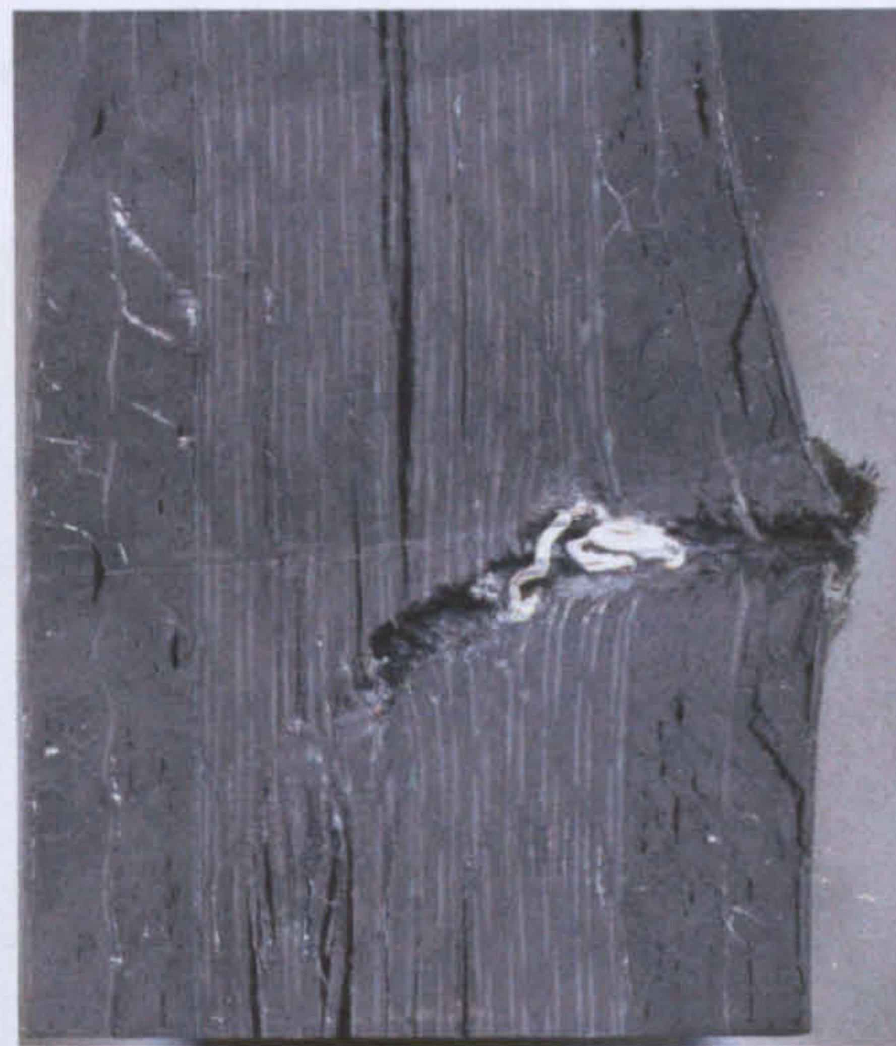
Image 6: Yaw in impacted carbon
