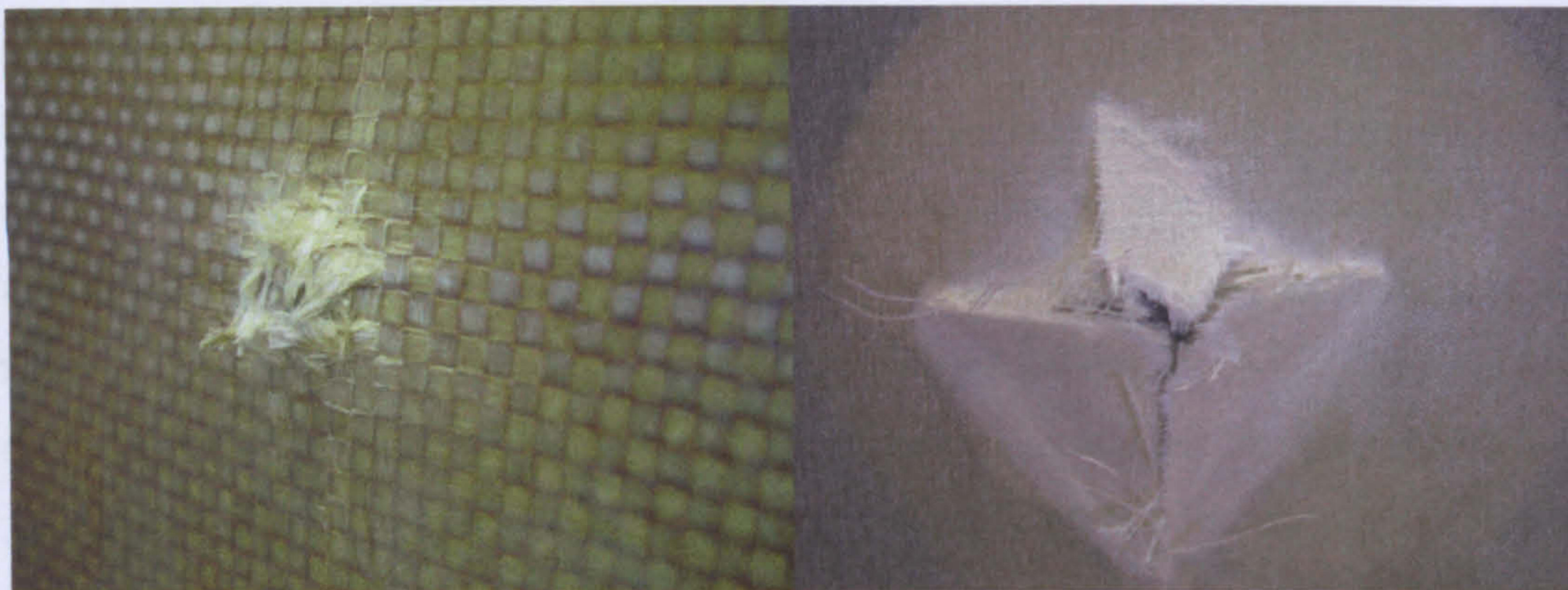
Image 6.2: Rear surface damage of heavy (left) and light (right) weave materials (different magnifications)
