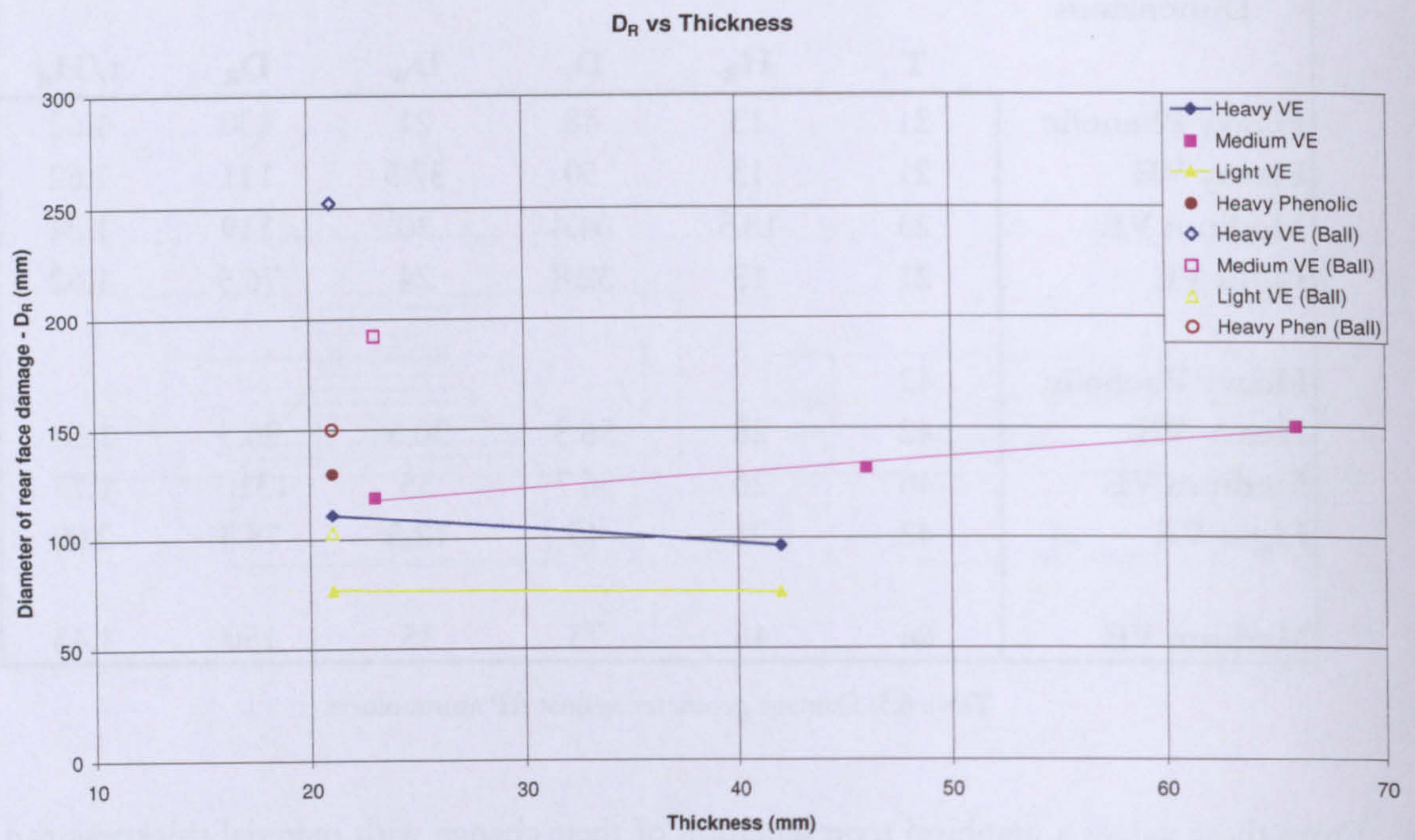
Graphs 6.12: D R vs target thickness for all materials, Ball and AP ammunition
