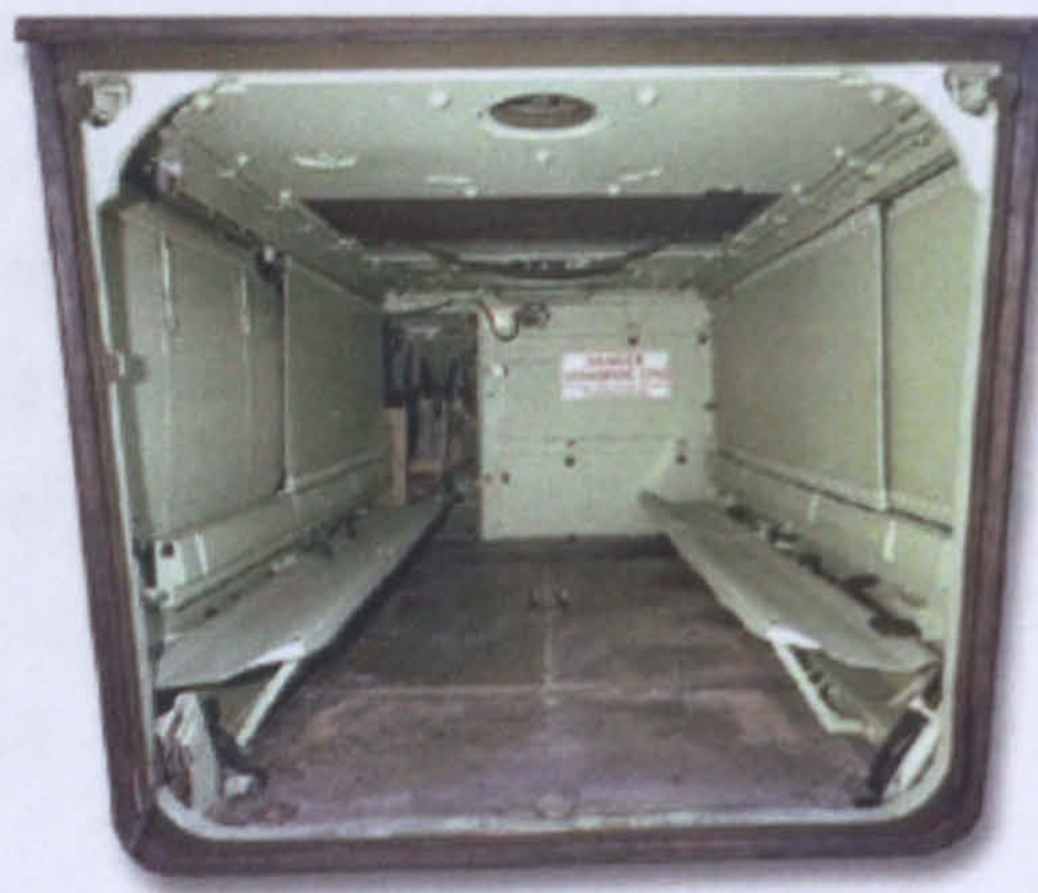
Image 2.5: A Kevlar spall liner in an M113 APC vehicle
