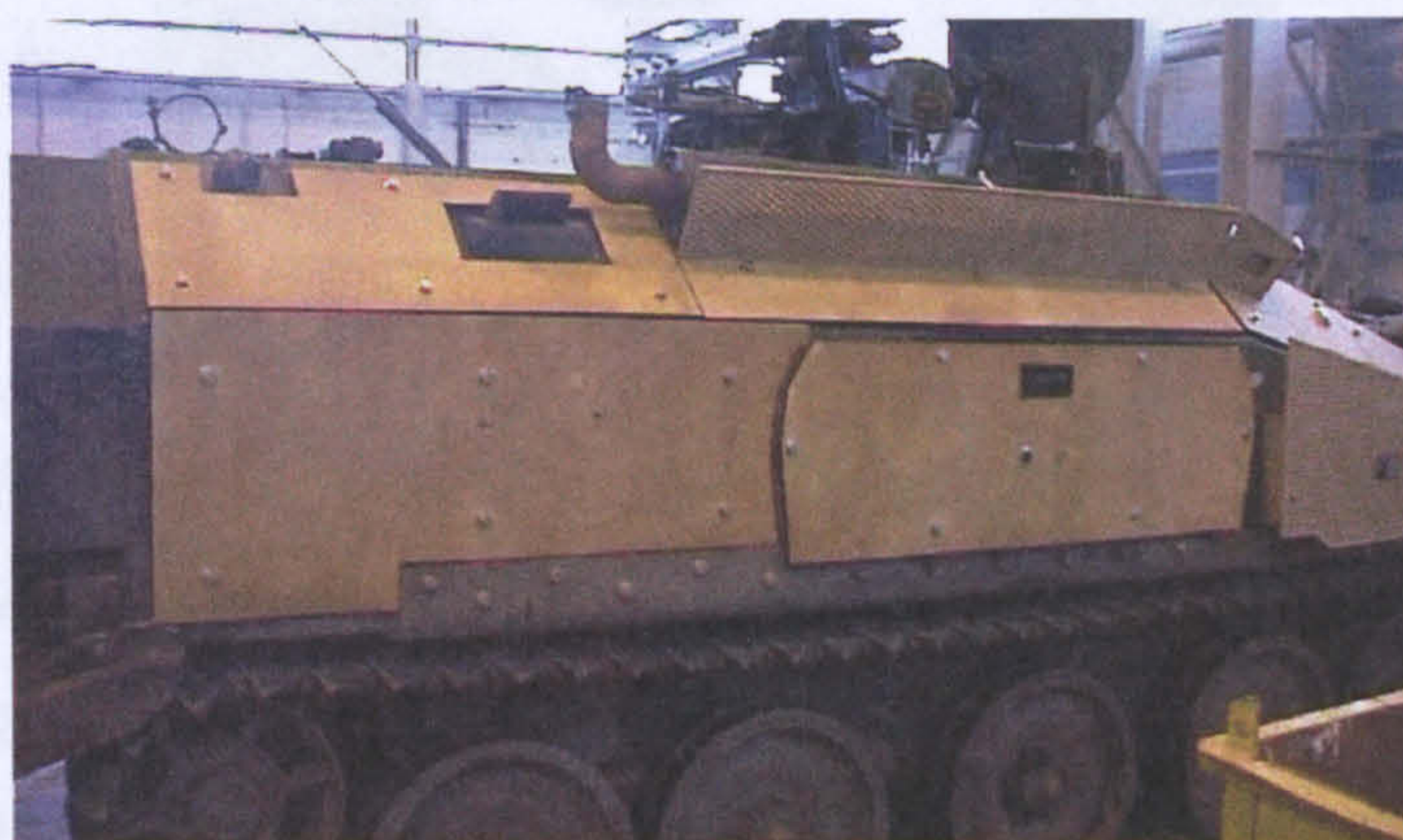
Image 2.6: Ceramic appliqué panels on a CVRT vehicle (Photo Courtesy of Lt Col A Roxburgh)
