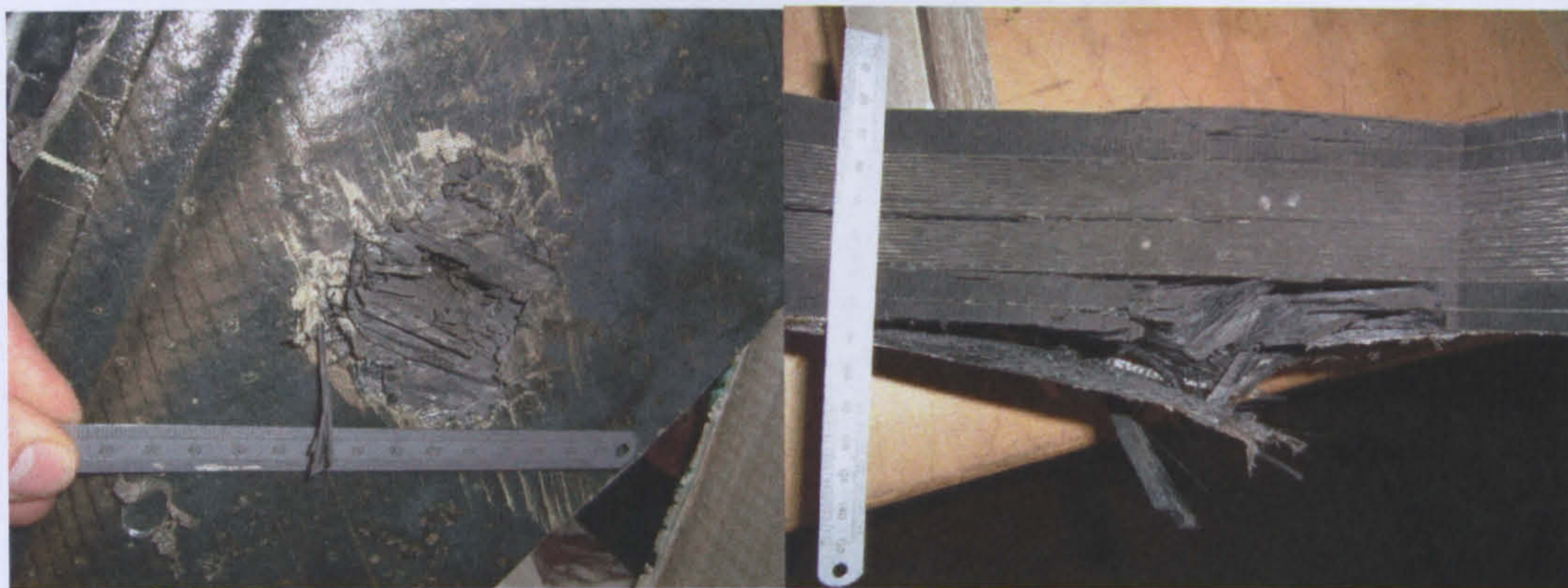
Image 8: Failure against STANAG level IV
