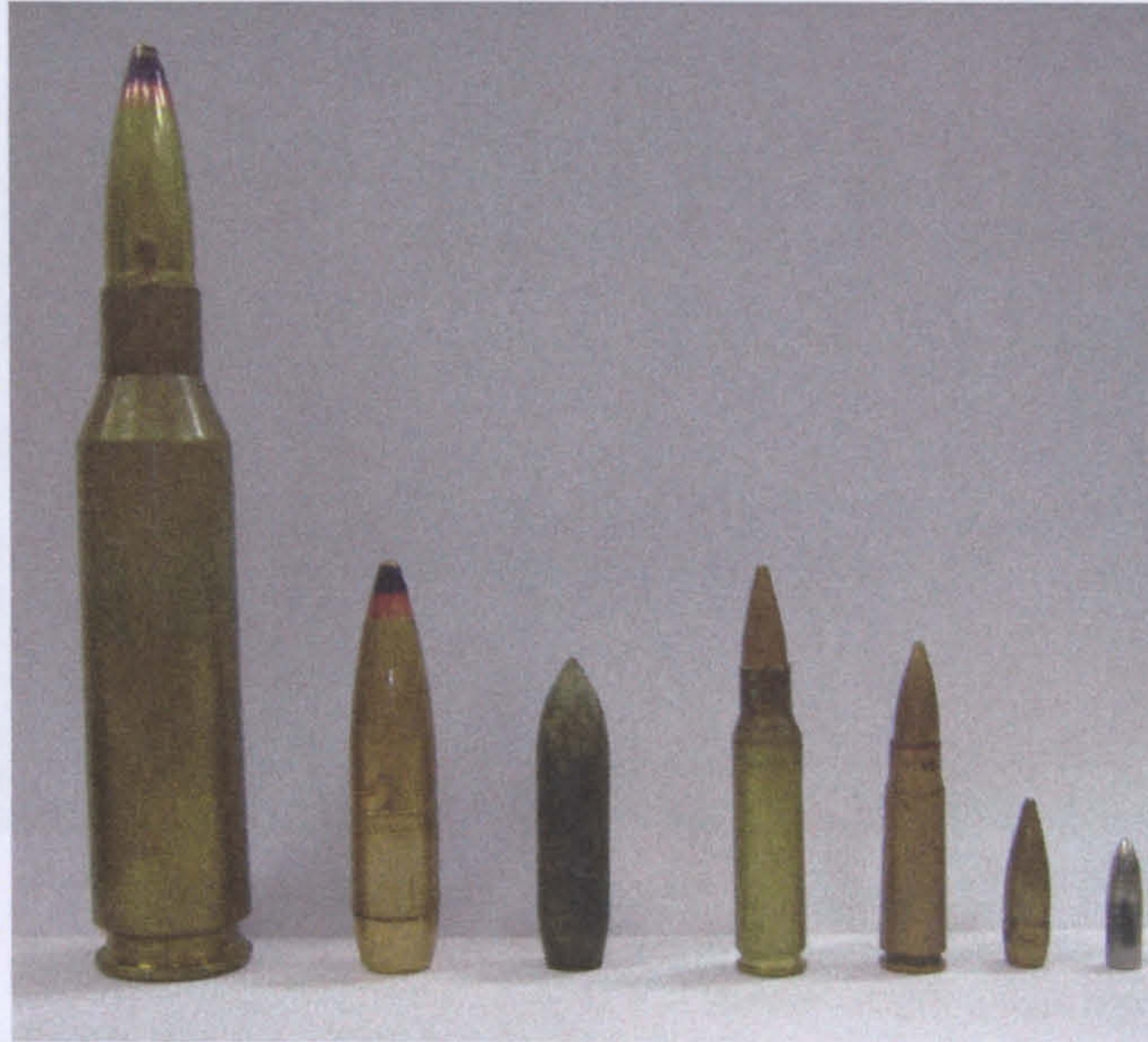
Image 1: Ammunition L-R: 14.5mm AP Complete, Bullet, Core, 7.62x51, 7.62x39 complete, Bullet, core
