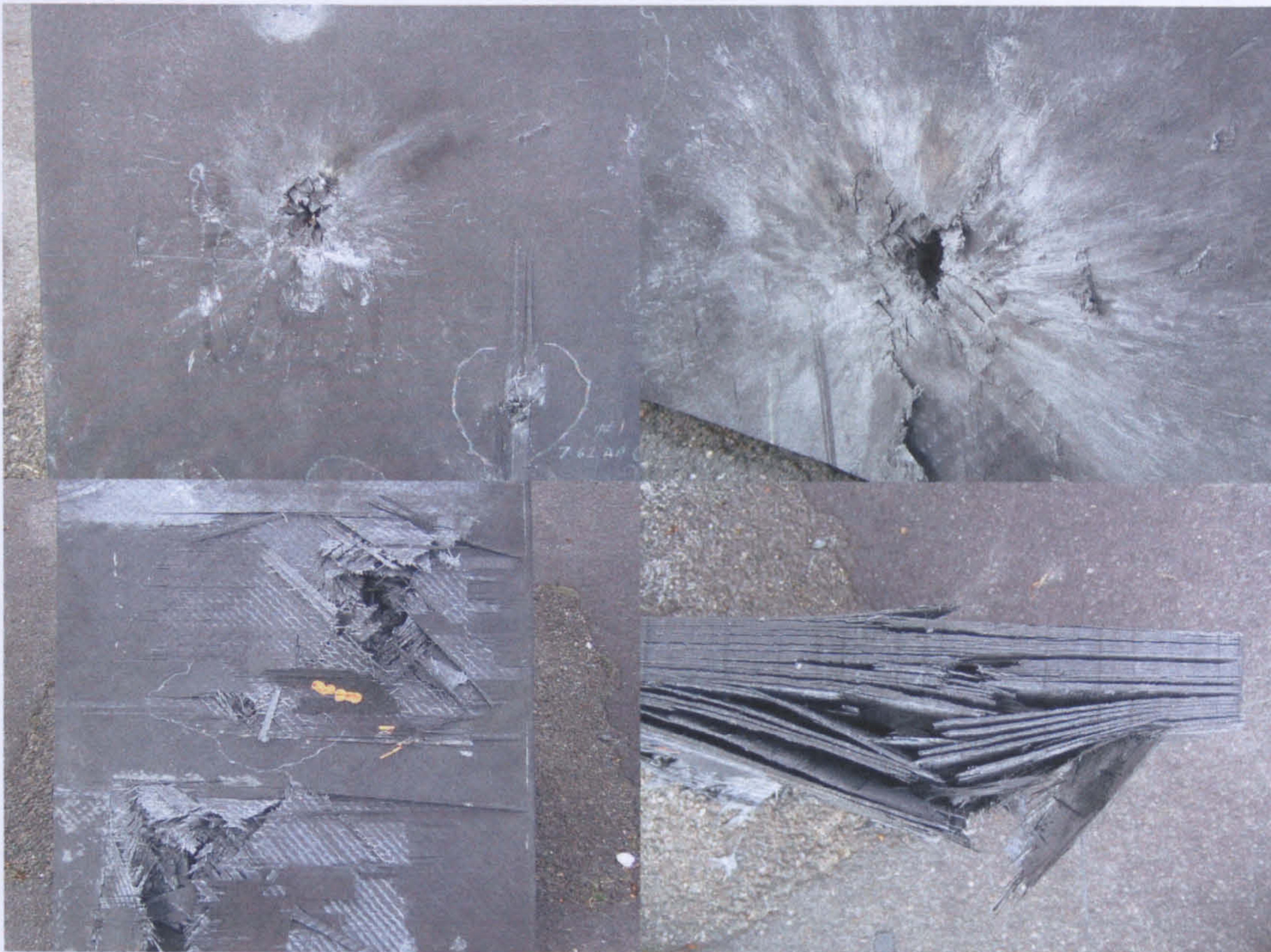
Image 5: 14.5 B32 (STANAG IV) vs Carbon panel + 20mm alumina tile 126\text{kgm}^{-2}
