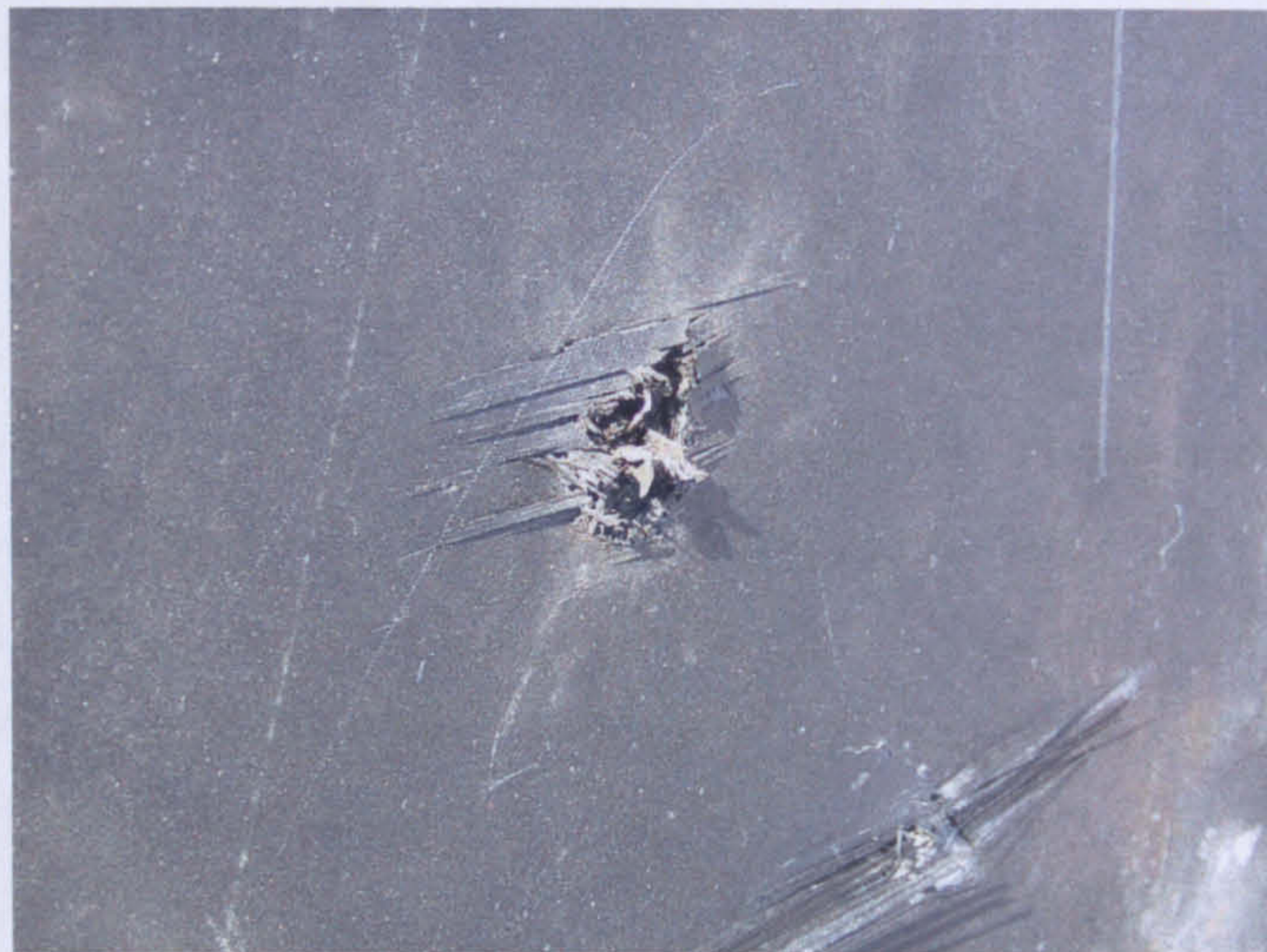
Image 3: 7.62 AP vs Carbon panel + 3mm mild steel spaced and inclined 66kgm -2
