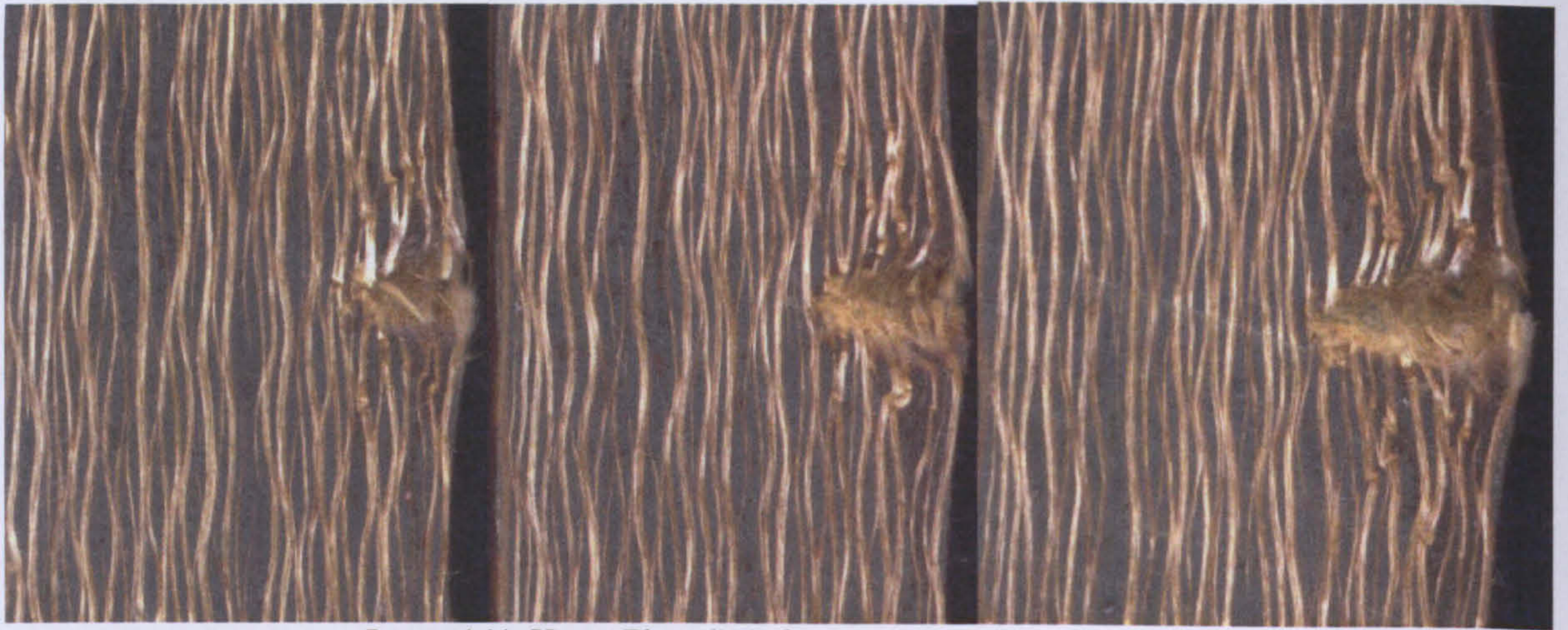
Image 4.11: Heavy Phenolic indentations(L-R; 50J, 75J, 100J)
