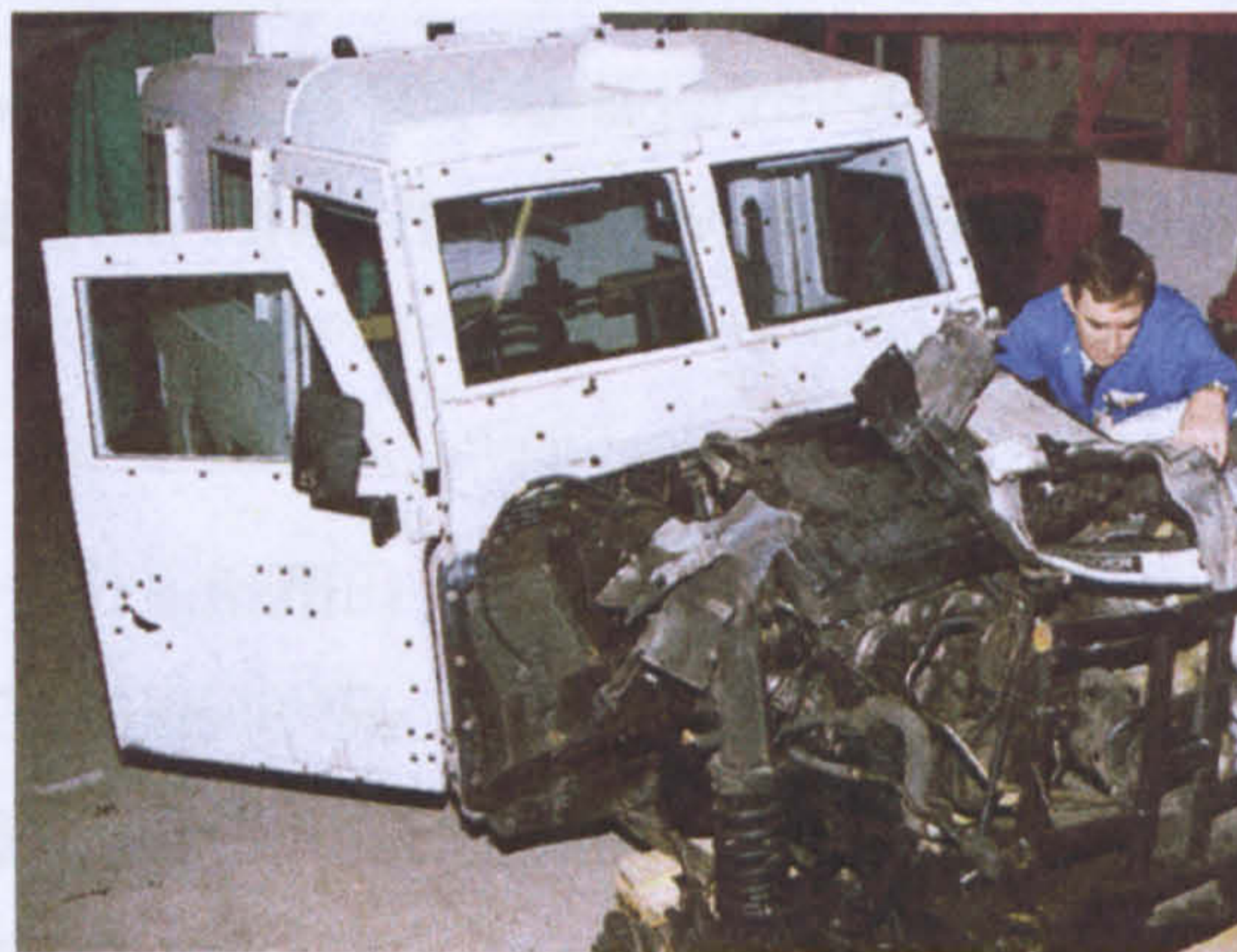
Image 2.9: Successful crew protection after mine detonation
