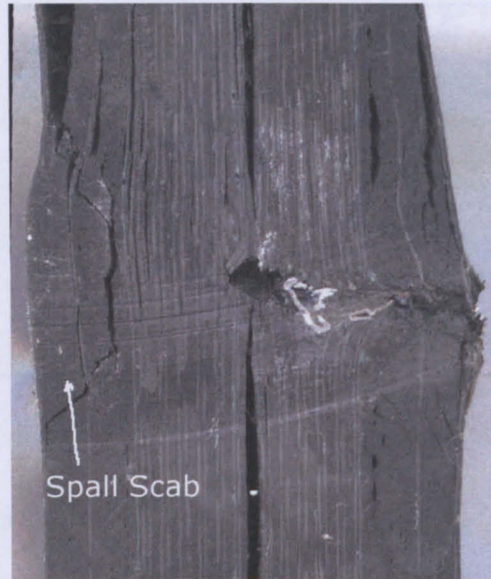
Image 7: Spall scab in impacted carbon
