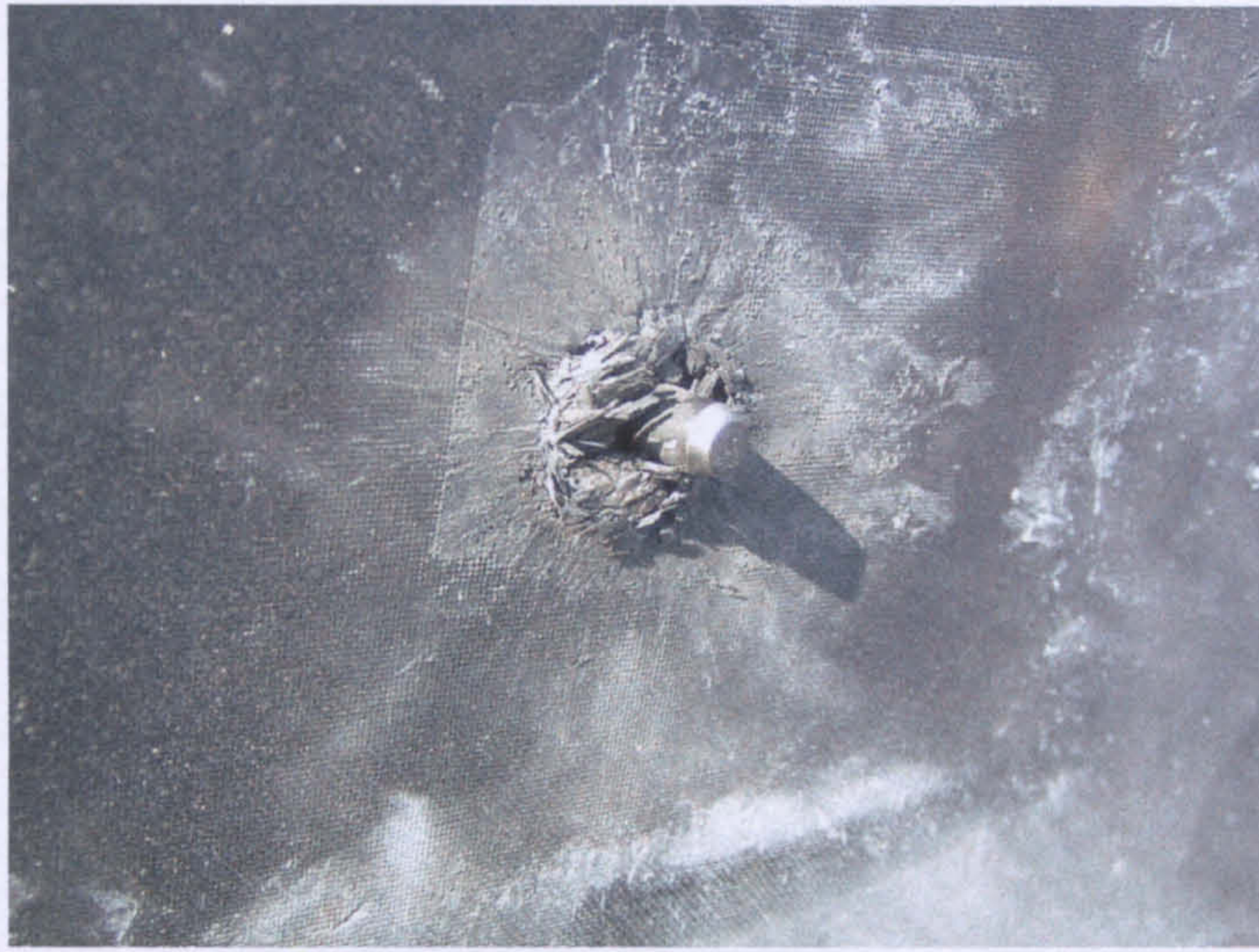
Image 4: 7.62 AP vs Carbon panel + 8mm alumina tile 78\text{kgm}^{-2}
