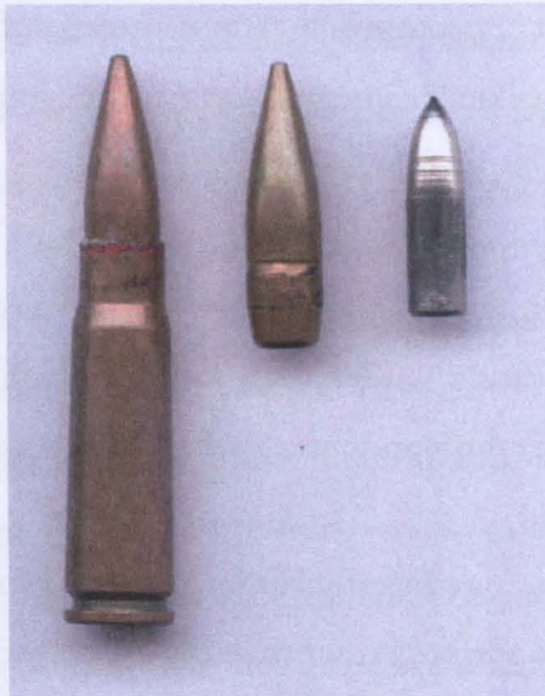
Image 2.12: 7.62x39 AP STANAG level II ammunition. L-R Complete round, Bullet, Core
