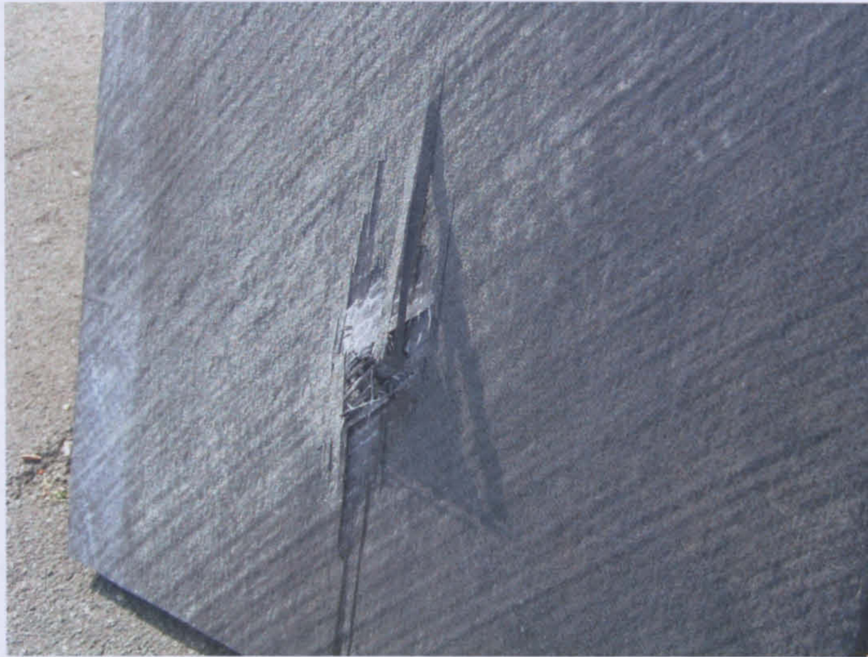
Image 2: 7.62 AP vs Carbon panel alone 44kgm -2
