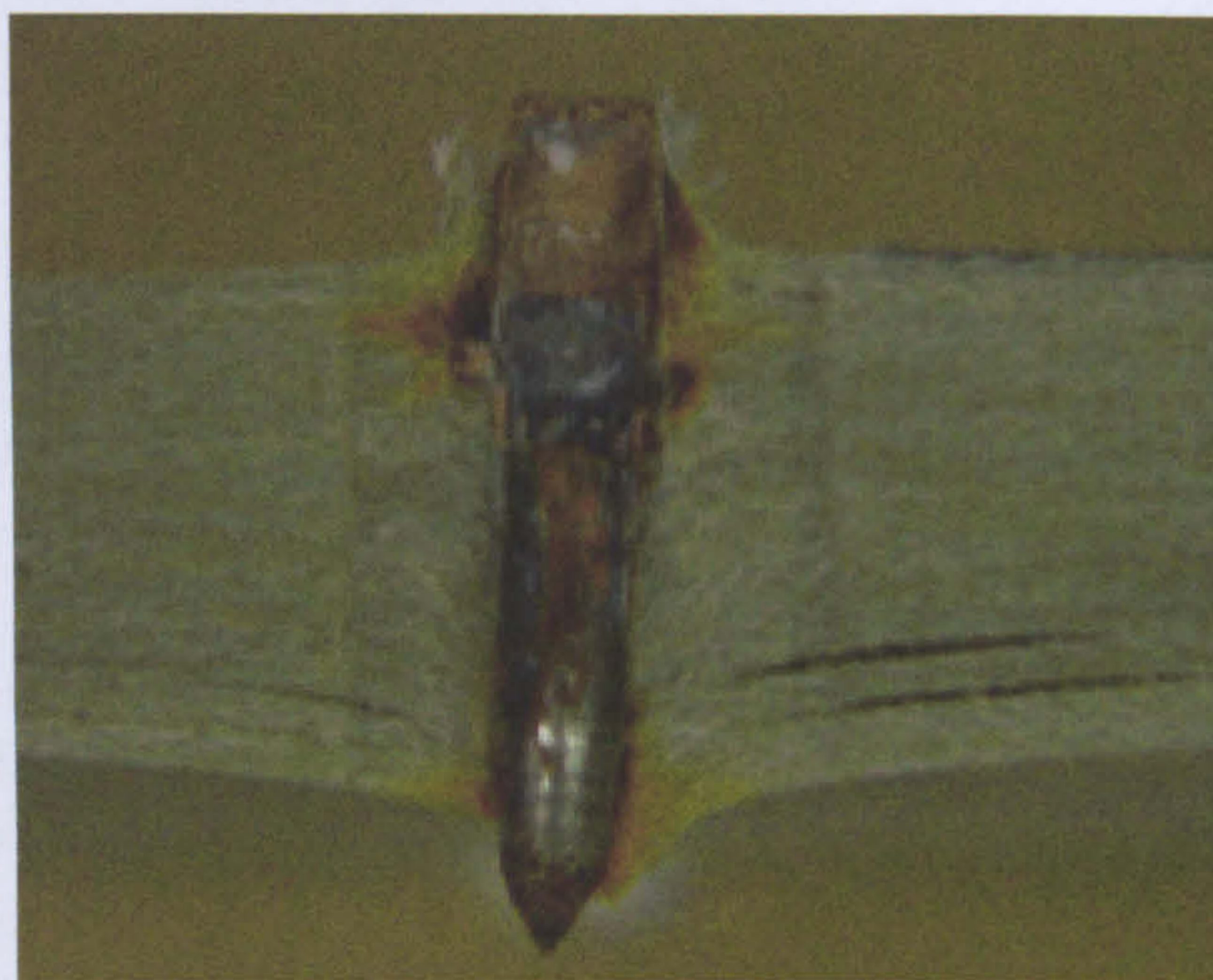
Image 4.7: Bullet embedded in armour showing plastic deformation through thickness from front face
