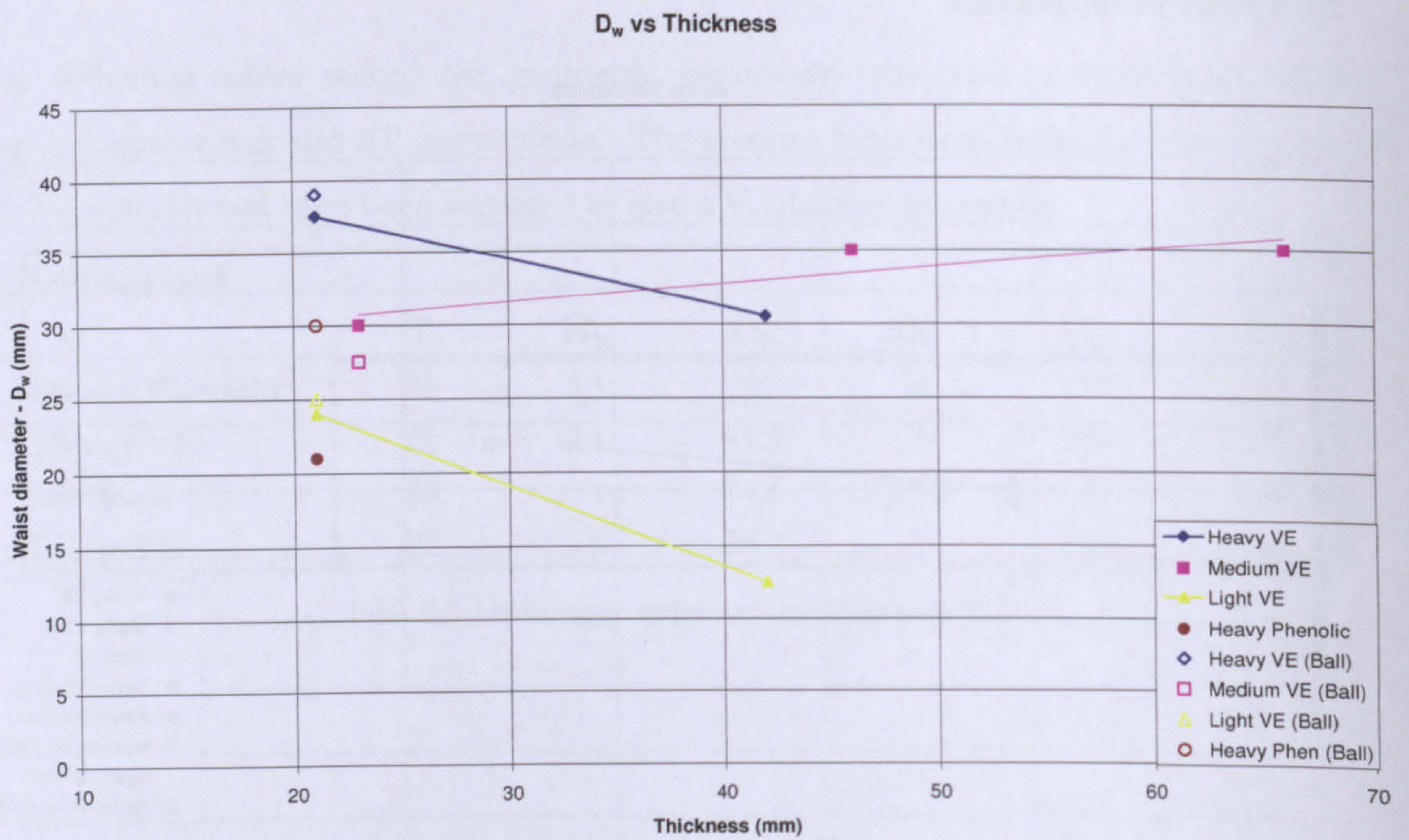
Graphs 6.13 D w vs target thickness for all materials, Ball and AP ammunition
