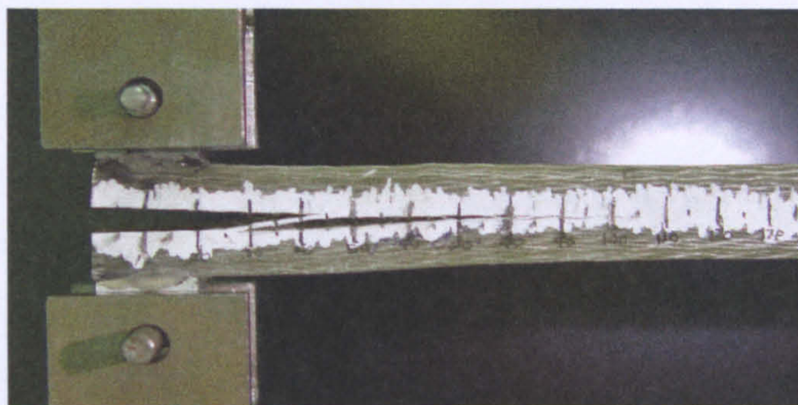
Image 5.1: Ply skipping invalidating test
