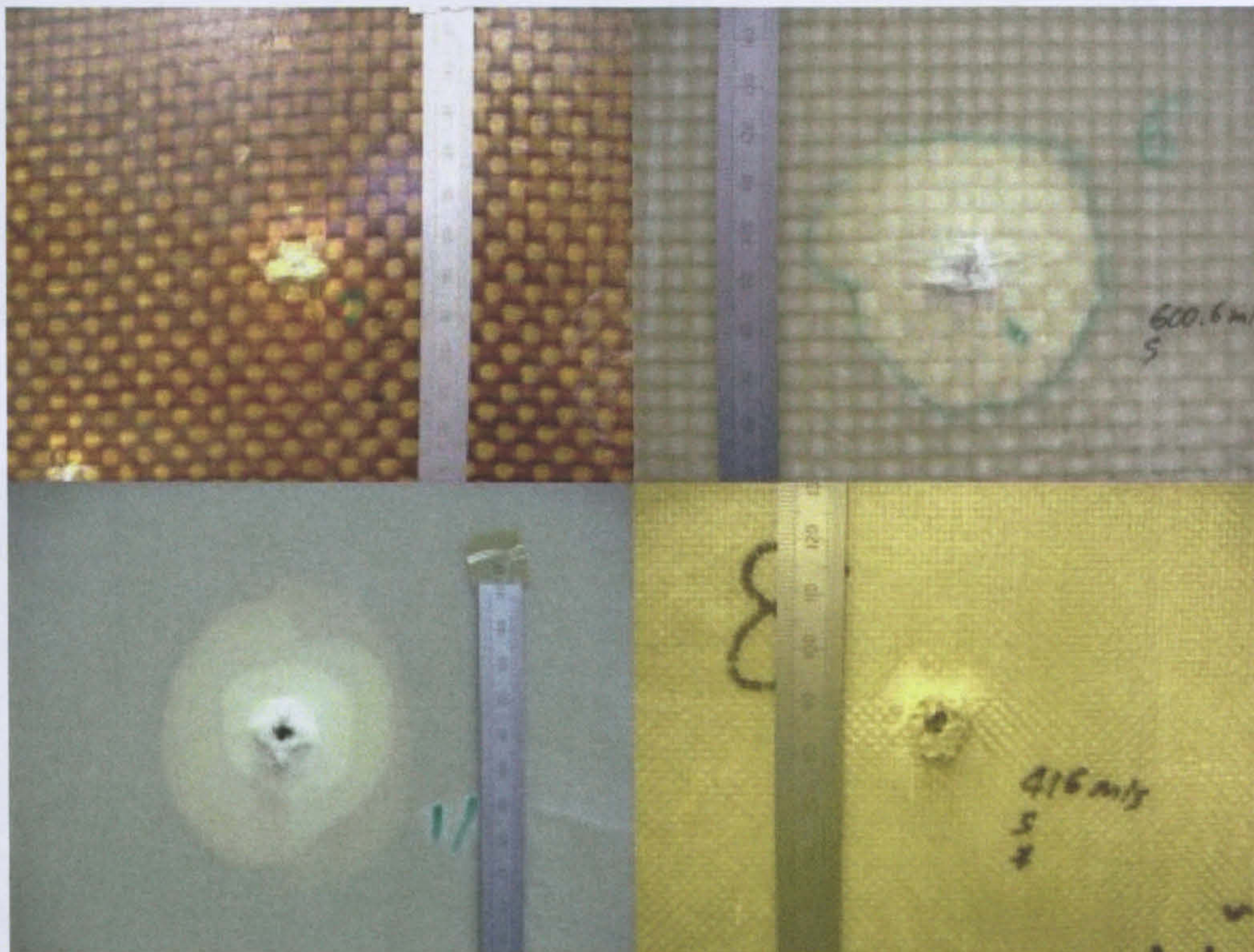
Image 3.8: Successful stops, front surface: CW from Top Left; Heavy Phenolic, Heavy VE, Light VE, Medium VE
