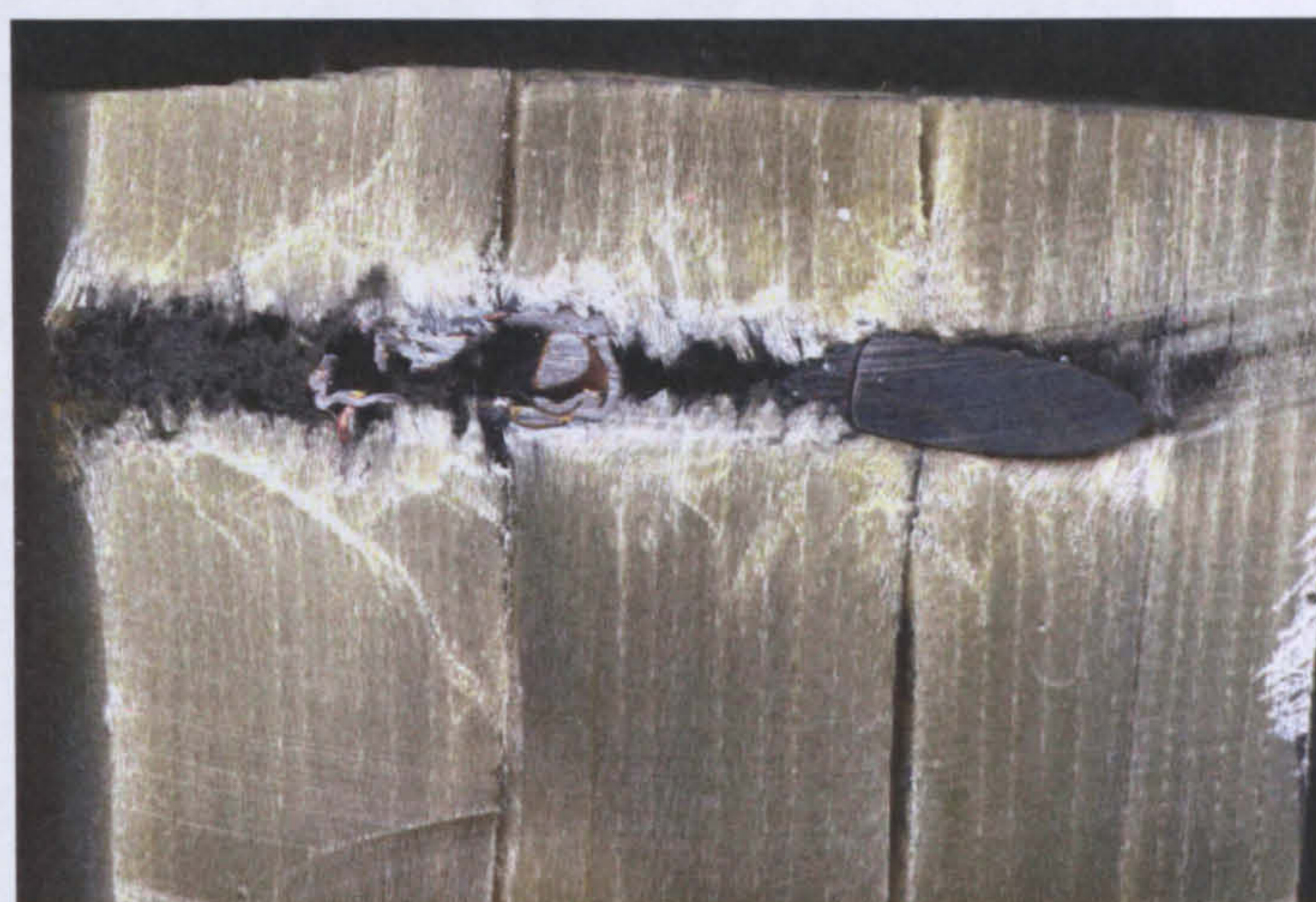
Image 3.27: Sections of treble thickness, medium weave Vinylester panel
