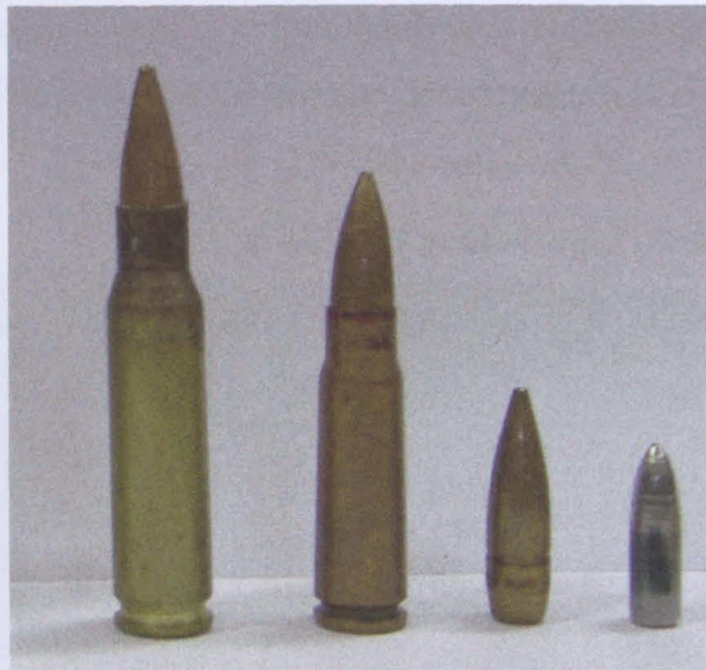
Image 3.7: Ammunition: Left – Right 7.62x51 Ball (FMJ), 7.62x39 AP (Steel Core), 7.62 bullet, 7.62 AP core
