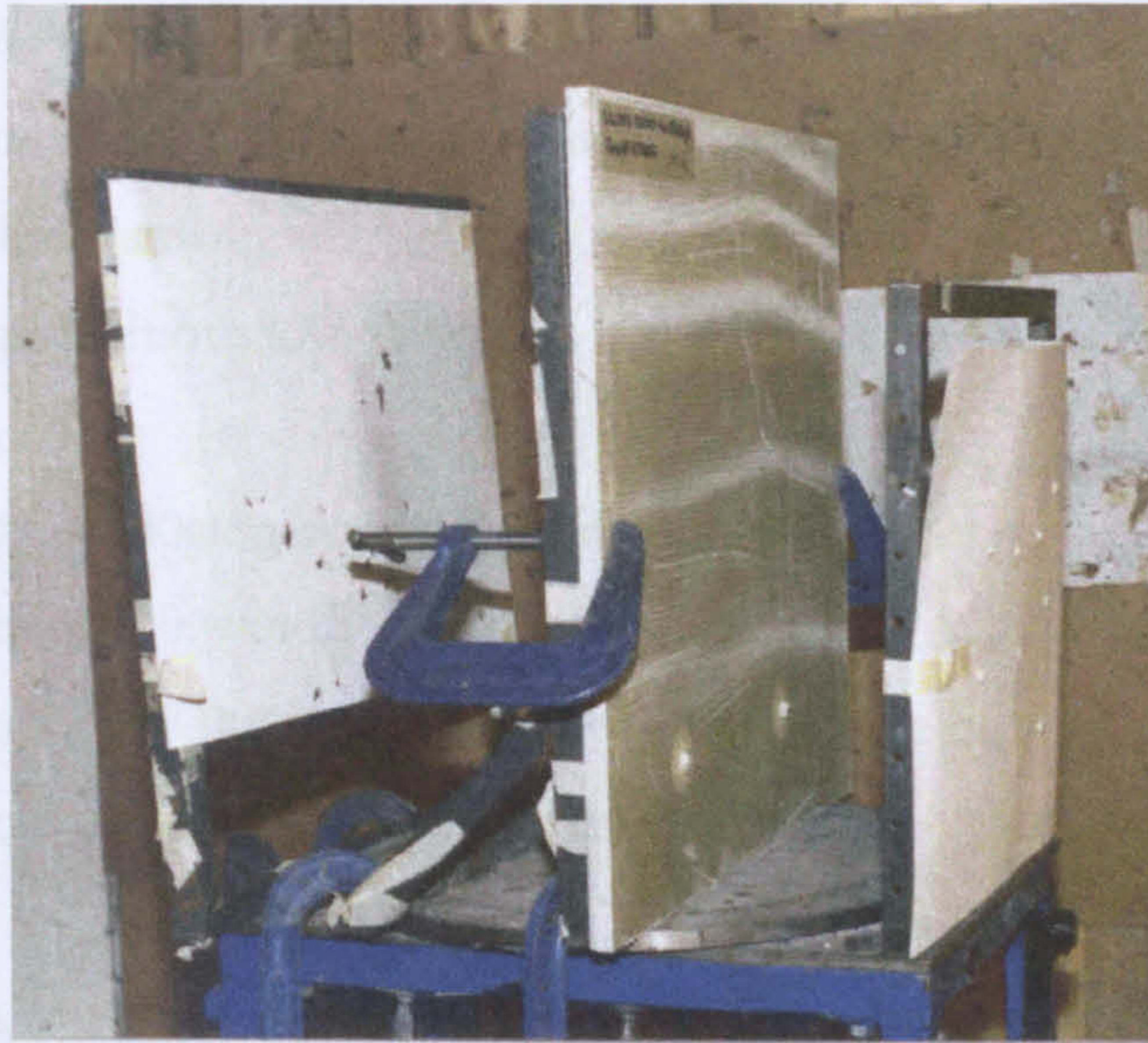
Image 3.2: Target arrangement with front and rear witness screens
