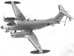
RC-12 K, Modified Beechcraft King Air ( www.fas.org/irp/program/collect/guardrail.htm ) Federation of American Scientists, Intelligence Resource Program
