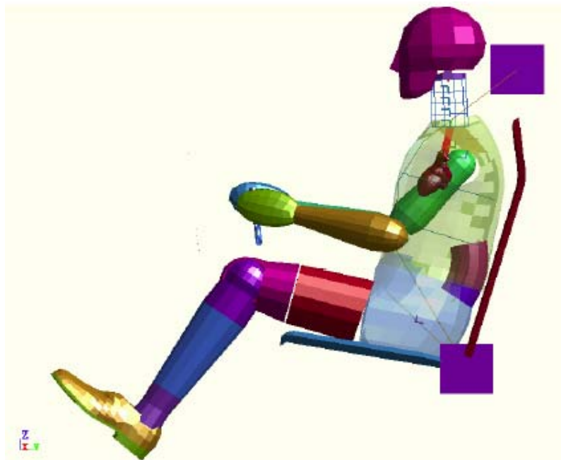
Figure 3-2. Simple Heart and Aortic Model in the Hybrid II ATD
