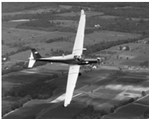
Condor Schweizer RG-8A / SA2-37B Length 8.79m, Height NA, Empty Weight 1,156kg, Gross Weight 1,950kg ( www.globalsecurity.org/intell/systems/rg-8.htm )
