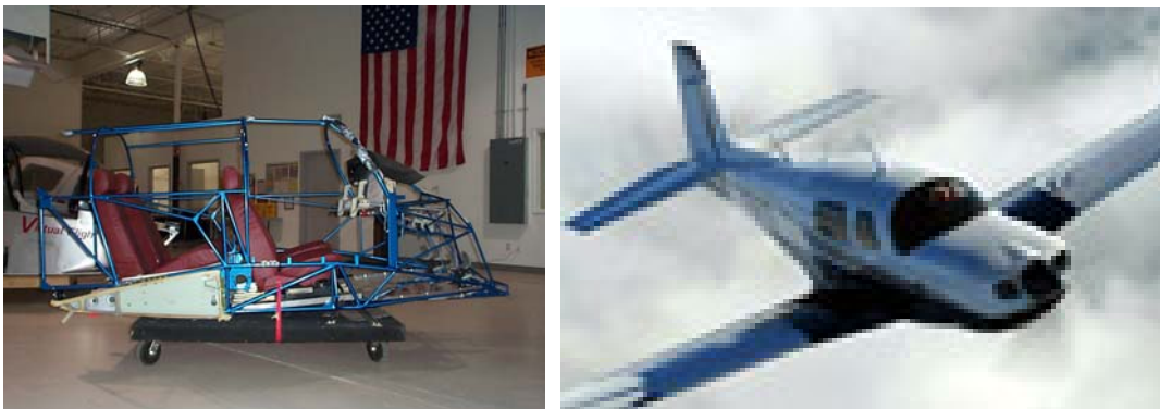
Figure 3-6 Mooney M20 Aircraft Fuselage Used for Interior Dimensions and an Image of a Complete Mooney M20 Aircraft
