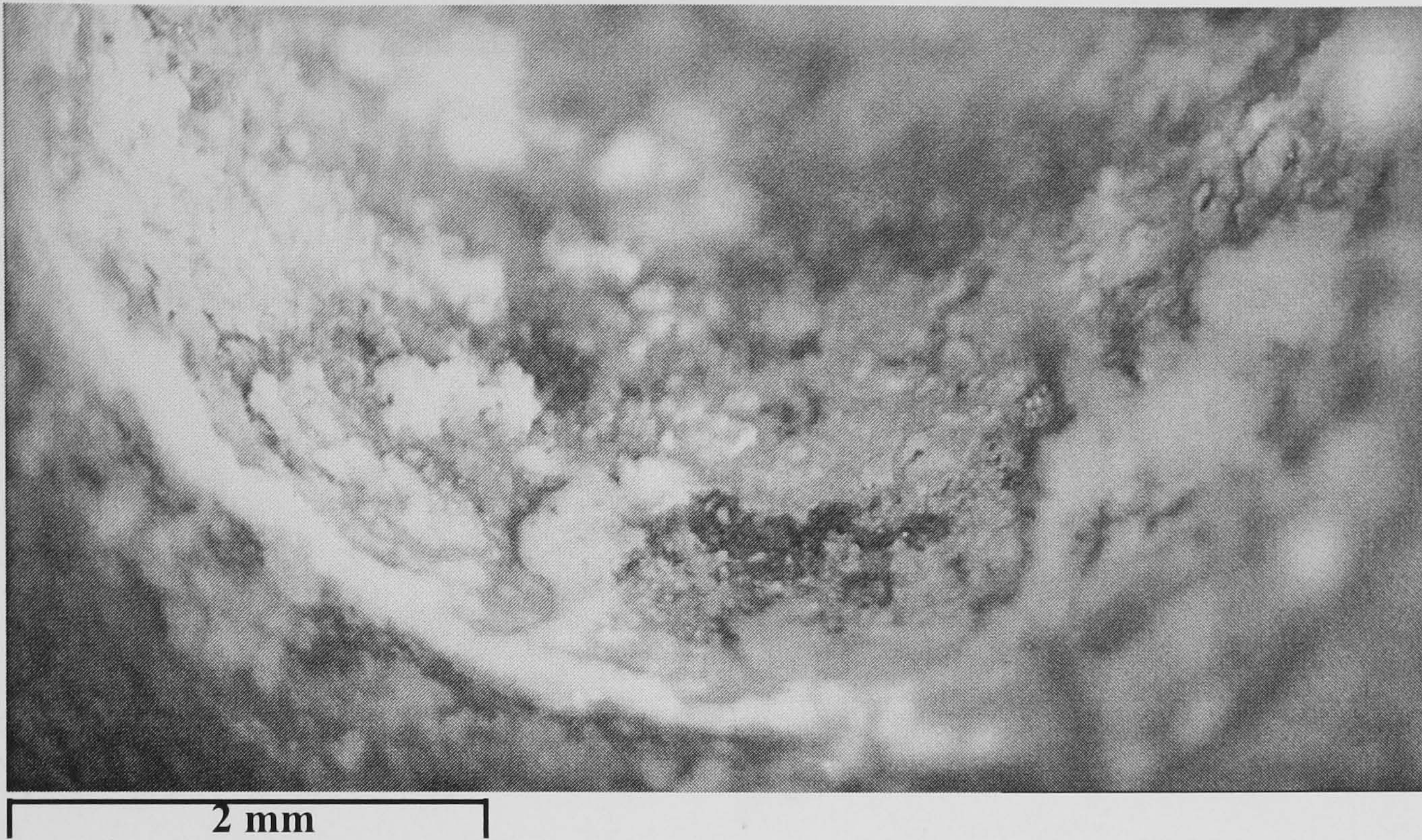
Figure 98 Optical micrograph showing the corrosion product inside the hole surface after 8 weeks.
