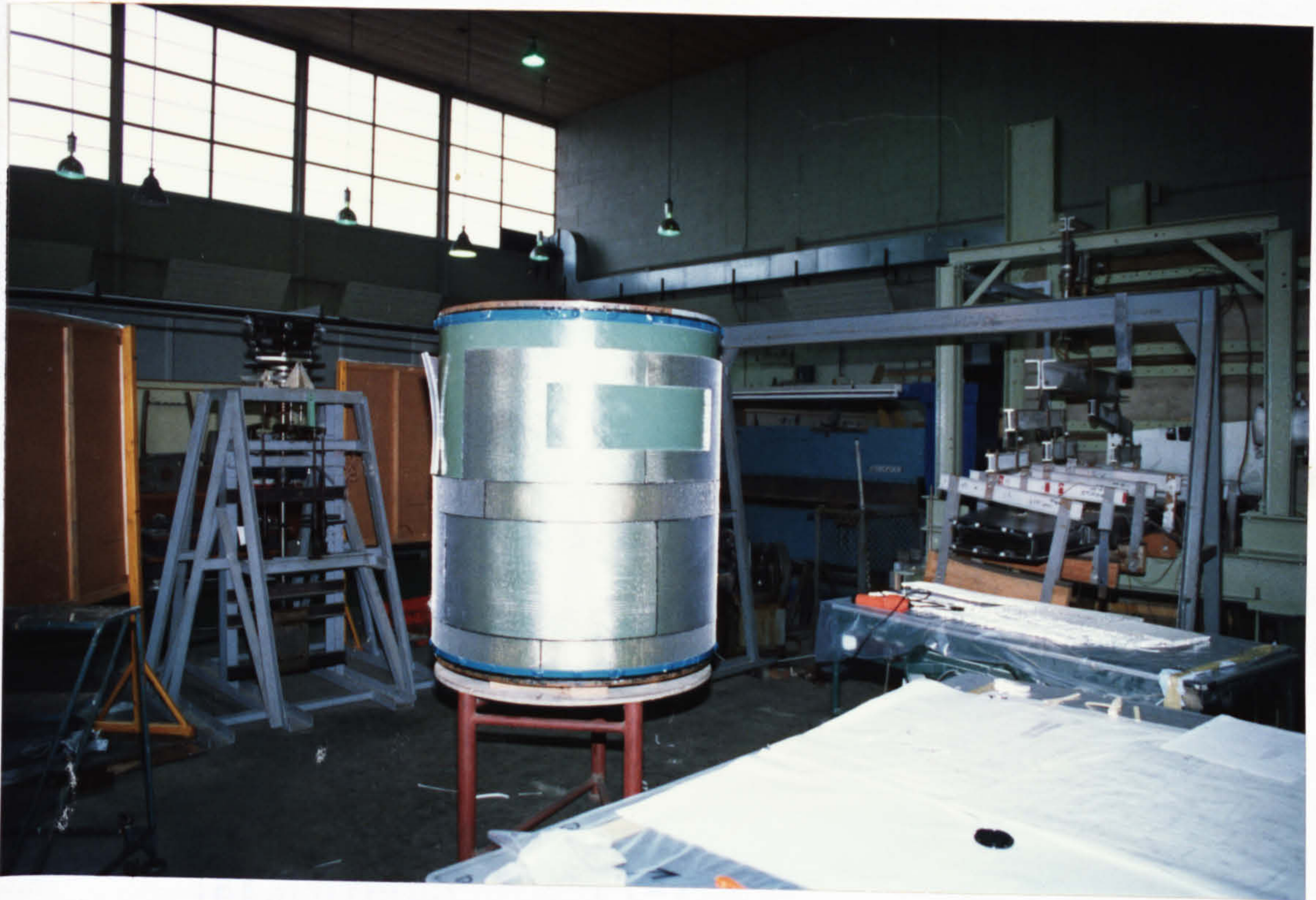
Fig. 9.6 HONEYCOMB LAY-UP ALMOST COMPLETED
