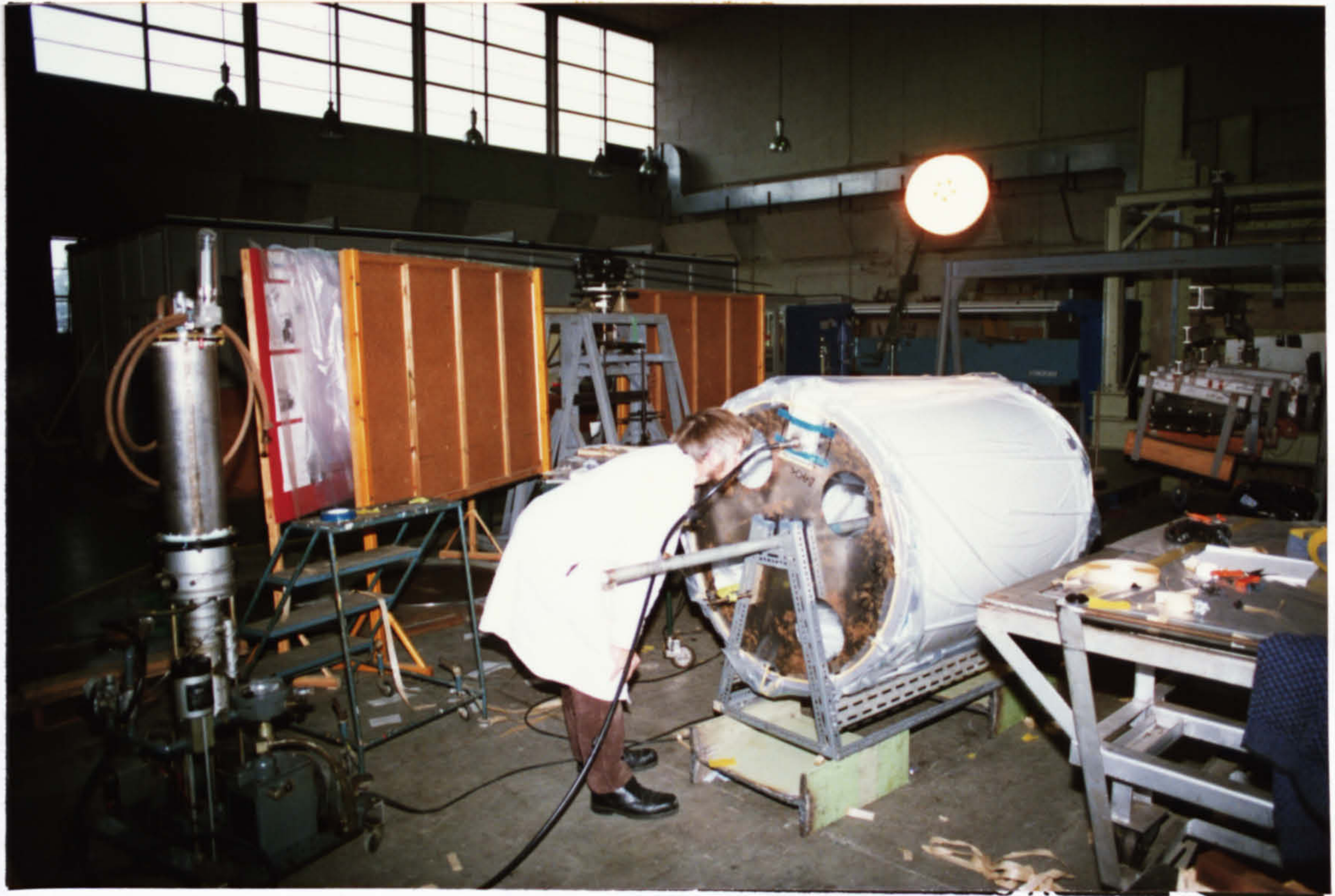
Fig. 9.13 APPLYING A VACUUM
