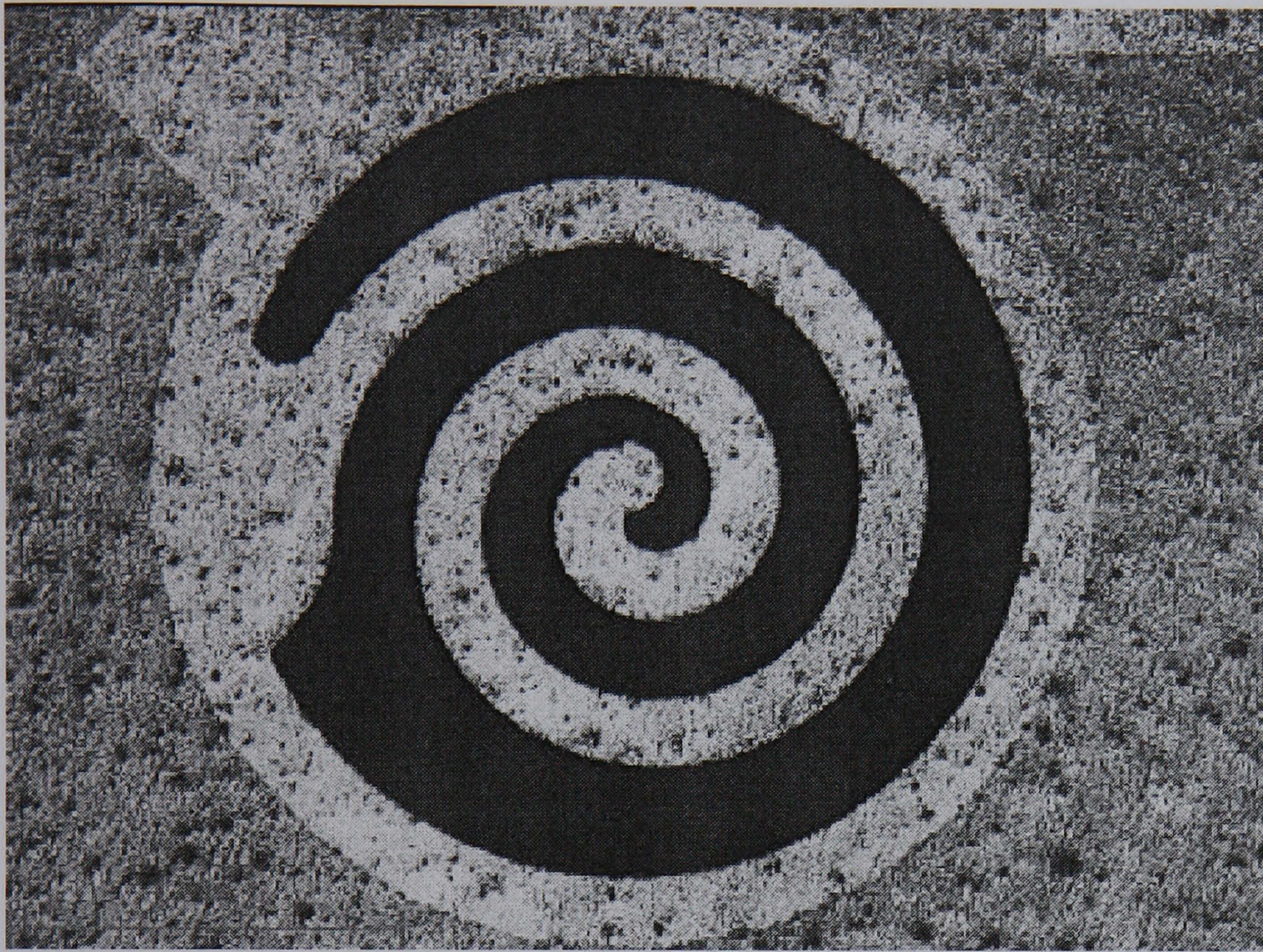
Fig 7.15 A 2mm diameter spiral actuator
