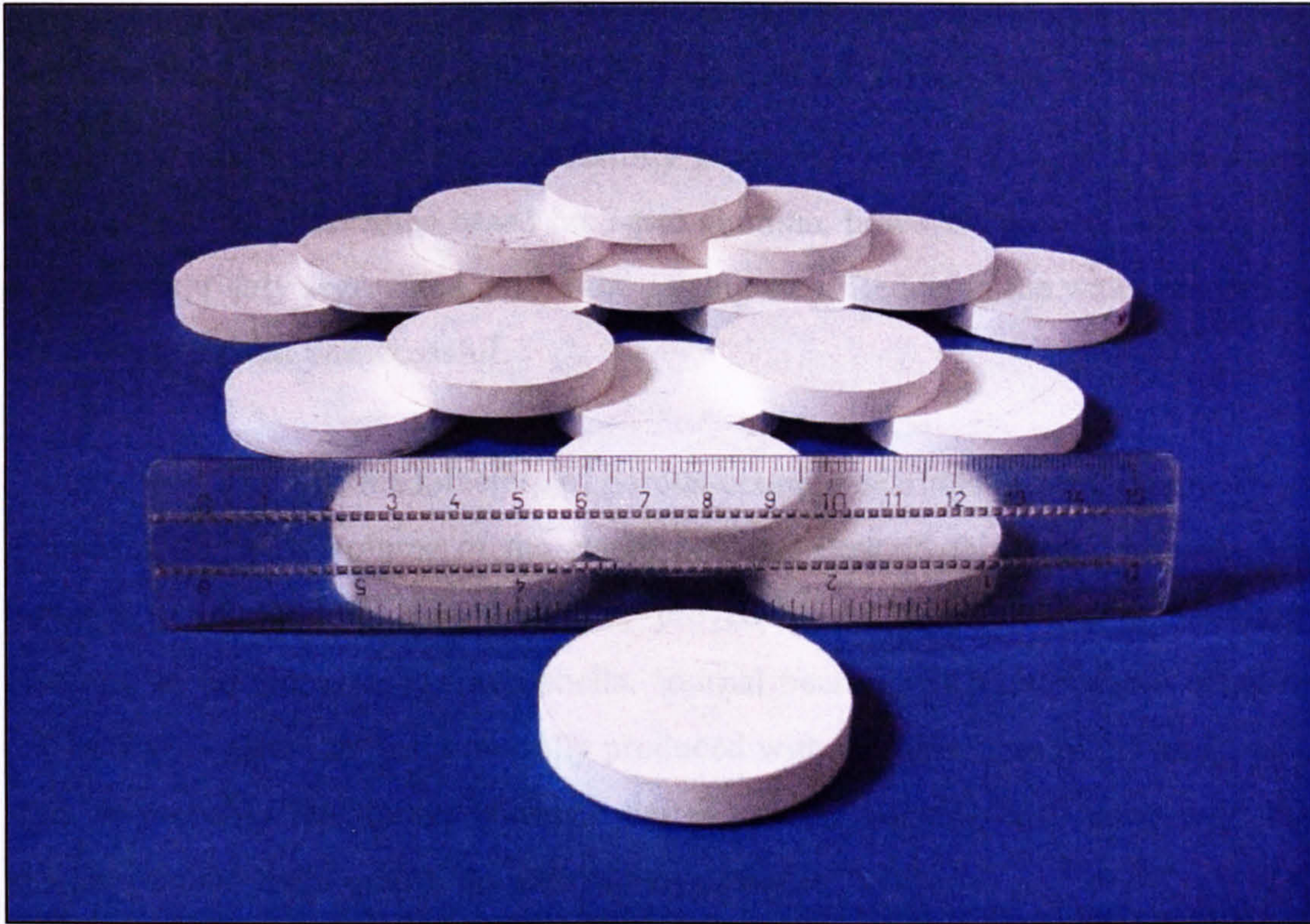
Figure 35-Porous-ceramic thrust bearings manufactured by the SC technique, \text{\O} 46\text{mm} \times 7\text{mm} thick.
