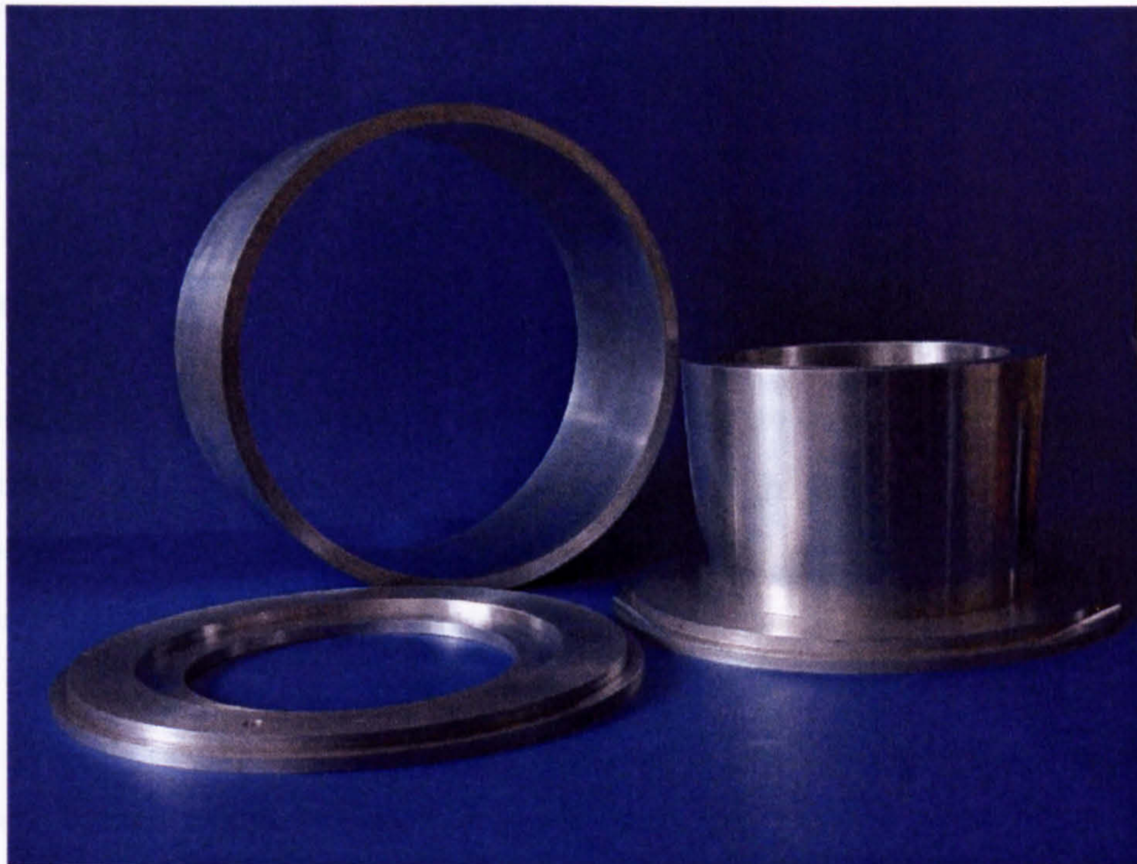
Figure 15-Typical 4-part aluminium mould for the manufacture of journal bearings.
