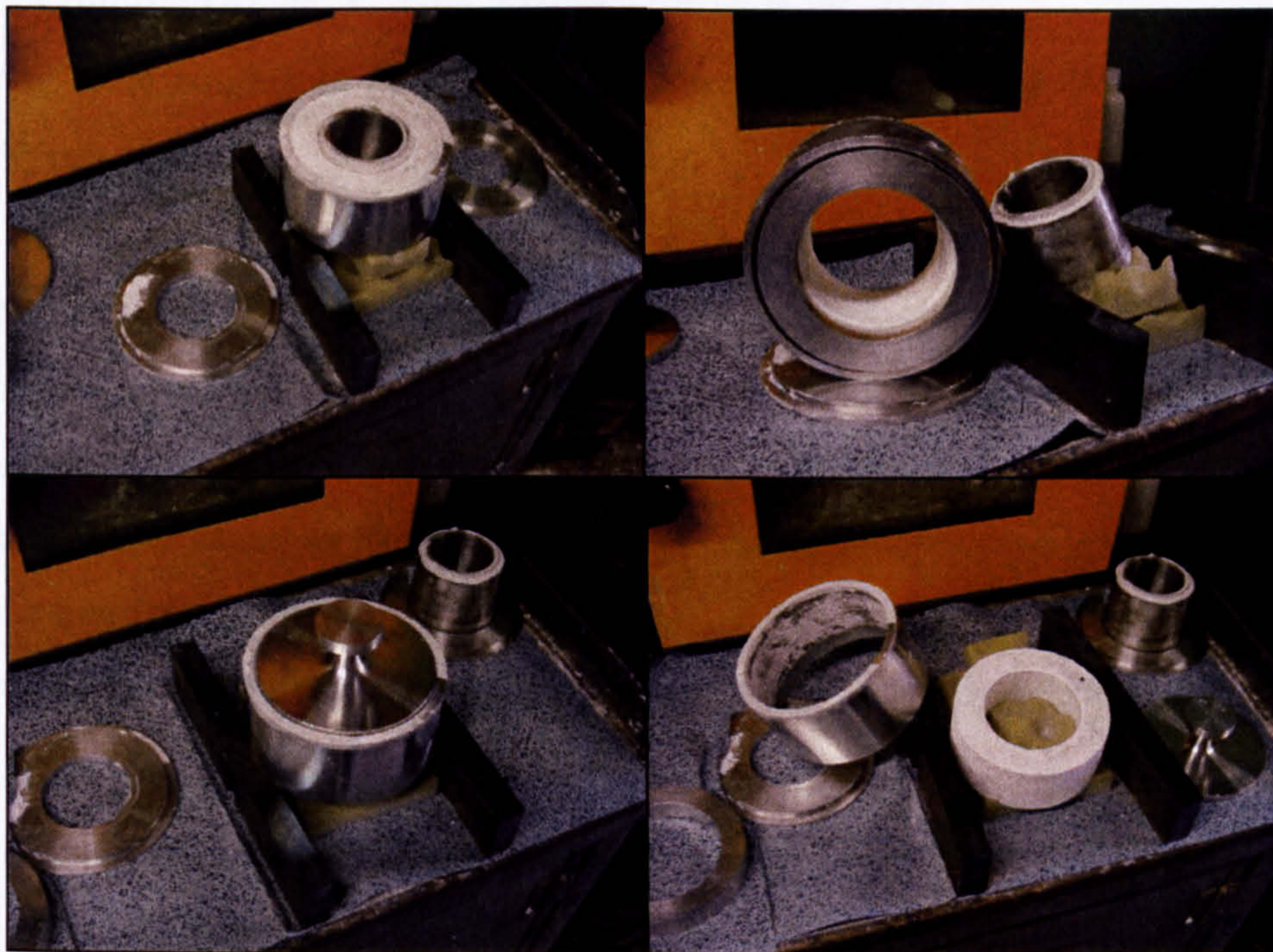
Figure 16- De-moulding procedure sequence. From left to right: 1-lid and base removal, 2-core removal, 3-casting ejection, 4-completed procedure.
