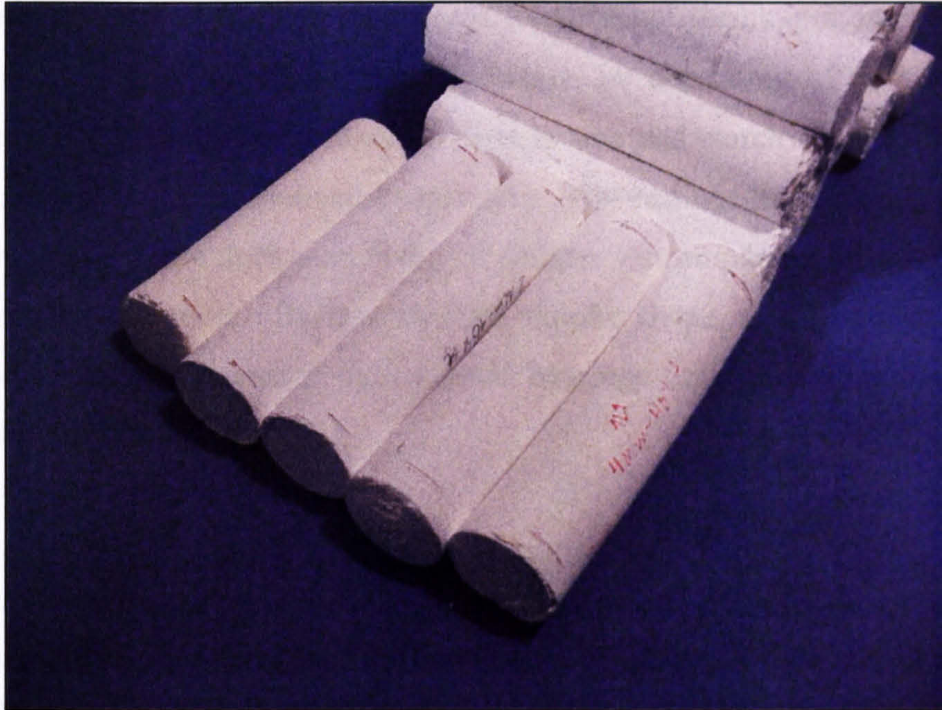
Figure 39-Shrinkage test cylinders after sintering. From left to right 0.5, 1, 2, 3 and 4 \mu\text{m} alumina at a fixed starch content of 40%. The further shrinkage of the 0.5 \mu\text{m} alumina is clearly noticeable.
