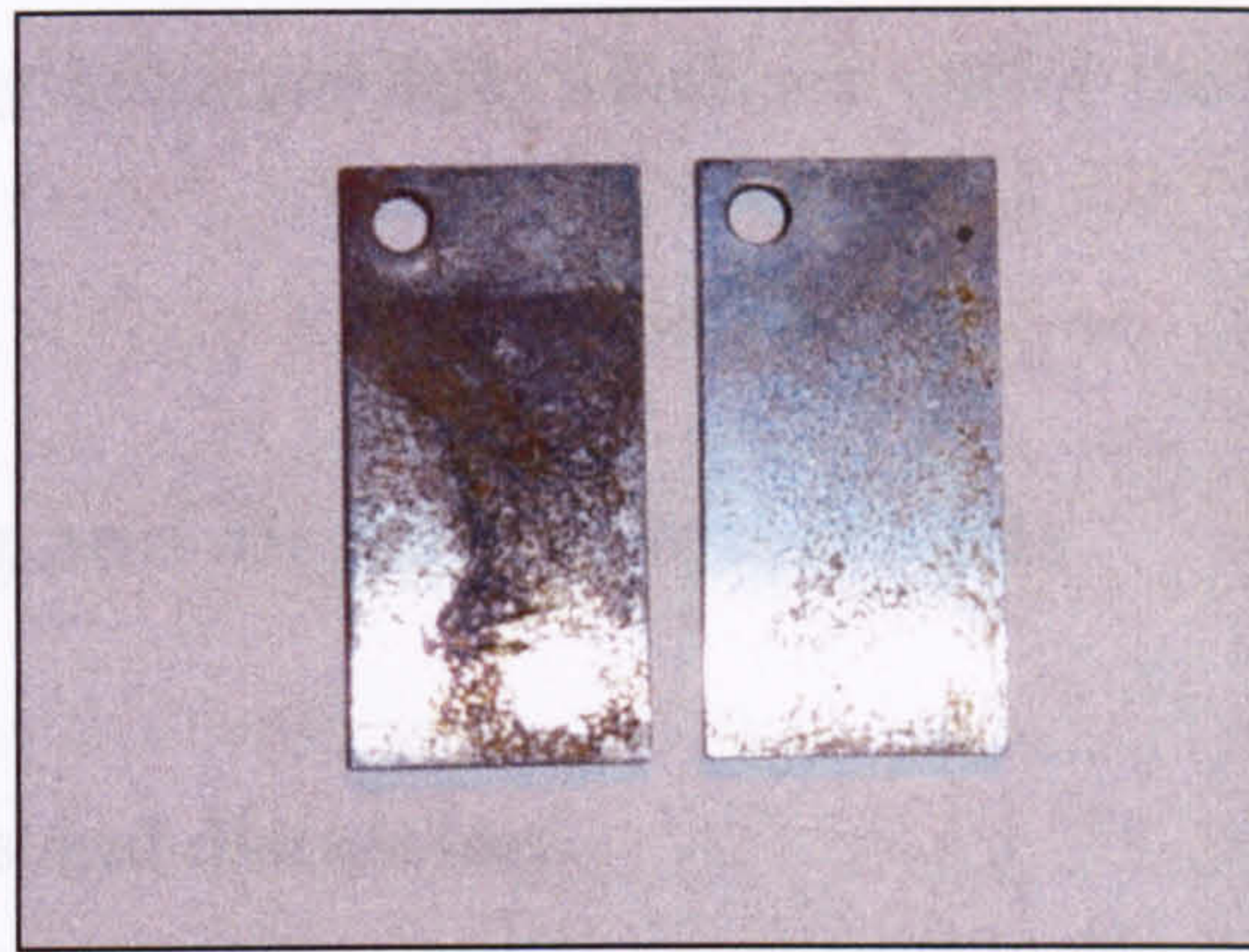
Figure 103- Cast iron corrosion test coupons rusted from an aborted inhibitor run (intermittent exposure).
