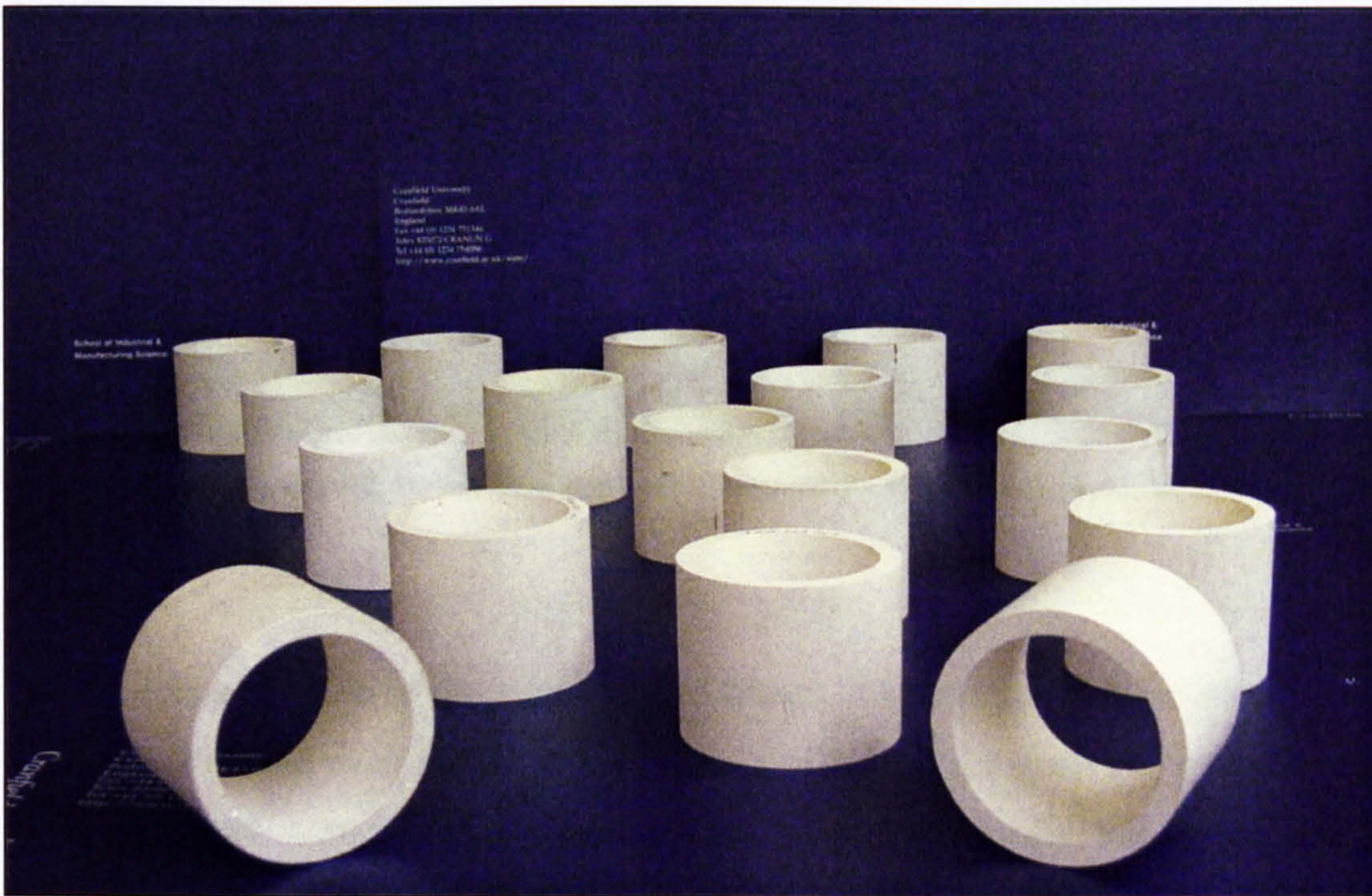
Figure 34-Porous ceramic journals bearings manufactured by SC technique, 50 mm ID, 62 mm OD and 50mm long.
