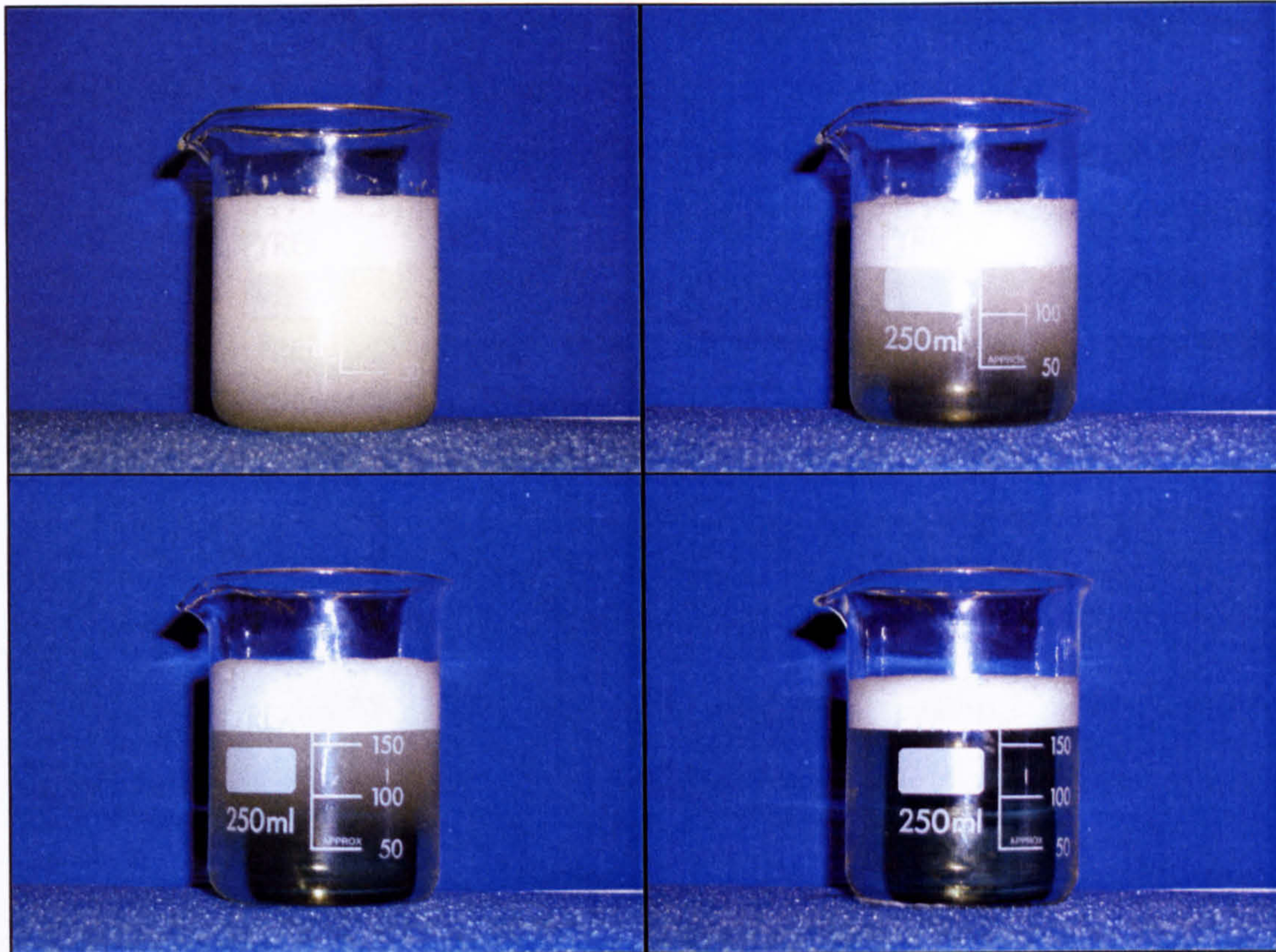
Figure 108- Dowell's sample, foaming and air release characteristics observed in porous-ceramic hydrostatic journal bearing test rig at 8000 rpm, 2.0 MPa lubricant supply pressure and an air supply pressure of 2PSI. In order from top-left to bottom-right: sample after 2 s, after 30s, after 1 min and sample after 2 min.
