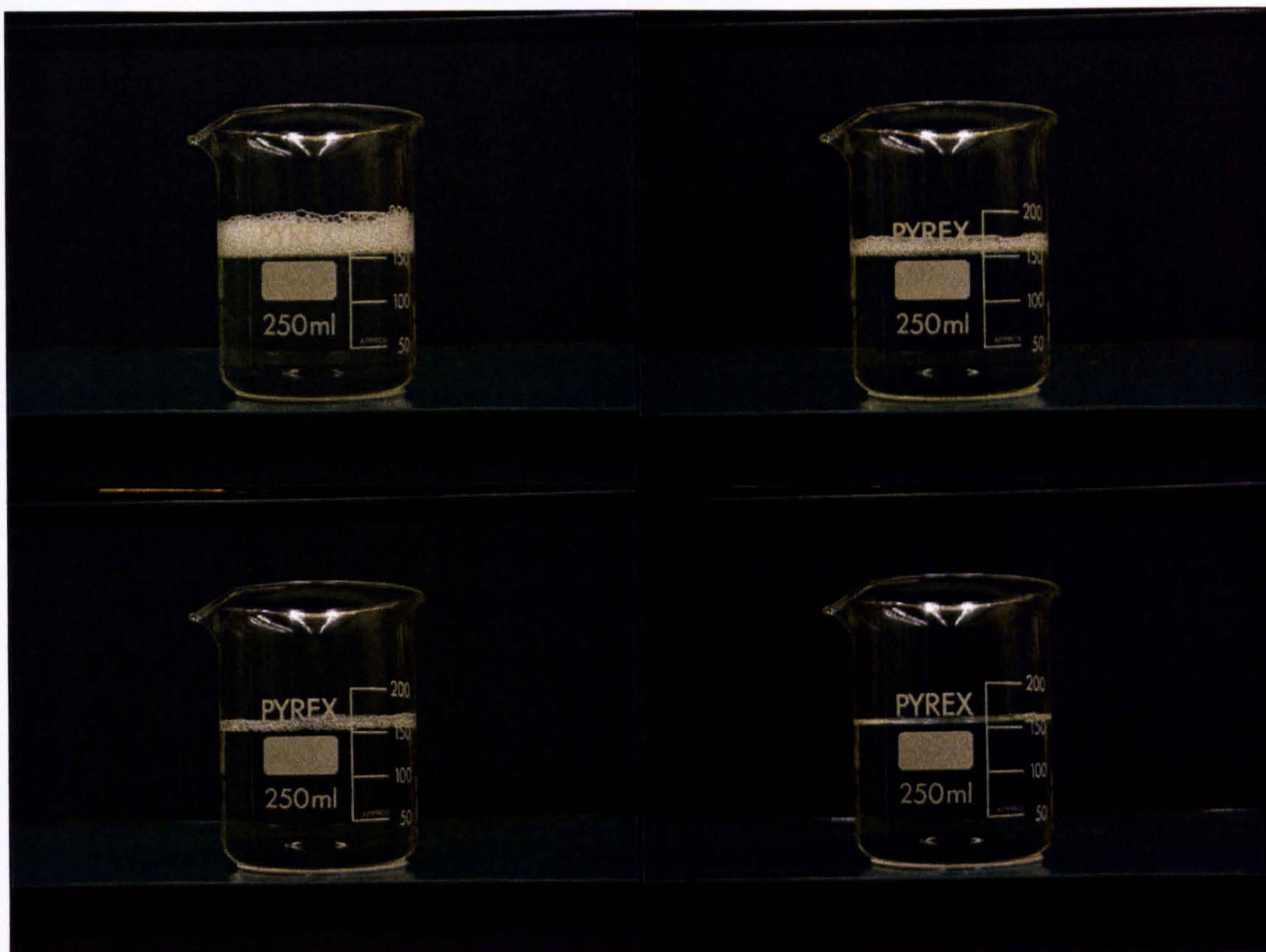
Figure 109- Oil DIE-180 foaming test sample. Foaming and air release characteristics observed in the porous-ceramic hydrostatic journal bearing test rig at 6000 rpm, 1.0 MPa lubricant supply pressure and an air supply pressure of 2PSI. In order from top-left to bottom-right: sample after 2 s, after 30s, after 1 min and sample after 2 min.
