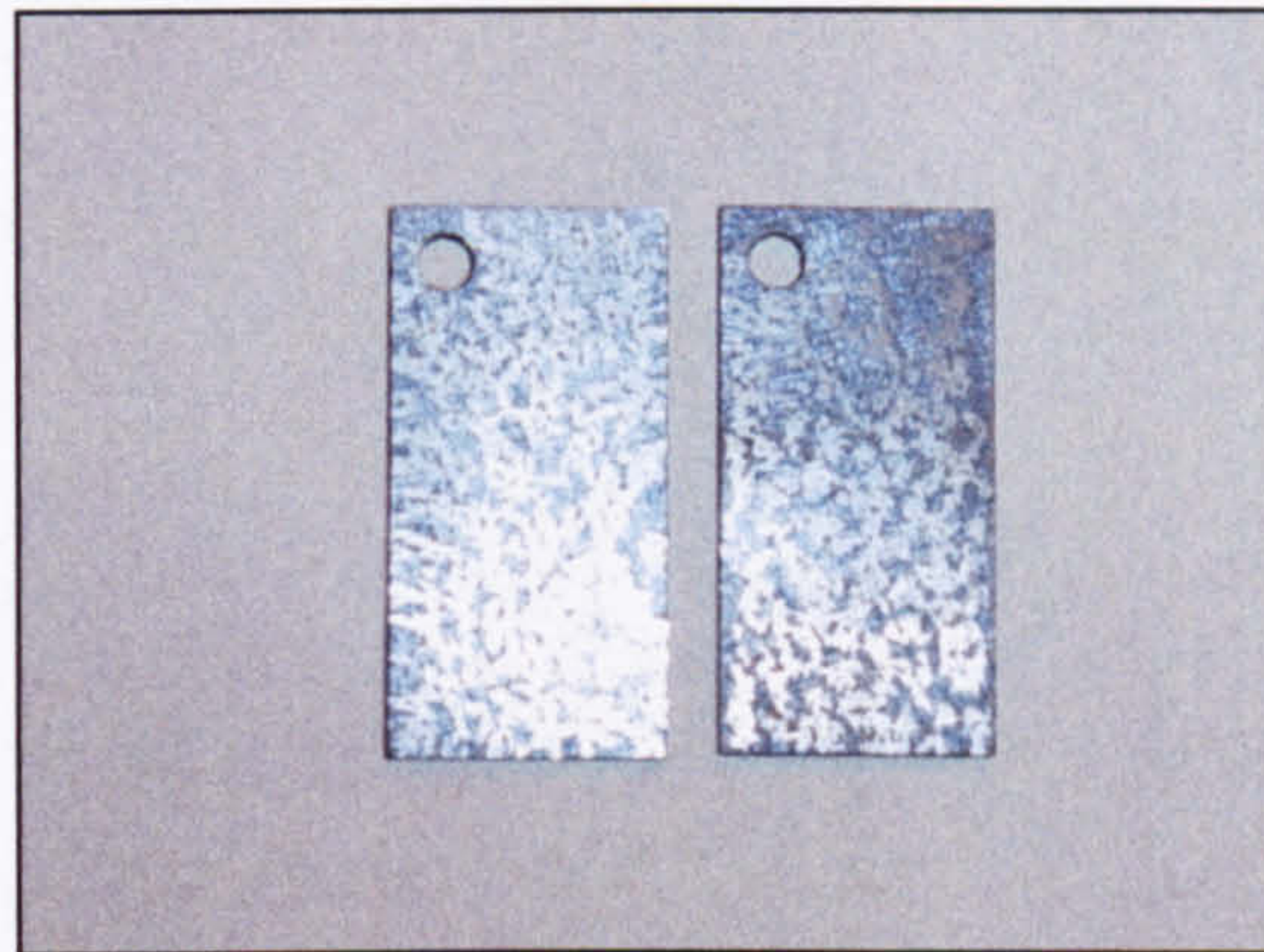
Figure 101-Cast iron corrosion test coupon immersed in plain water, 40°C and 600 rpm.
