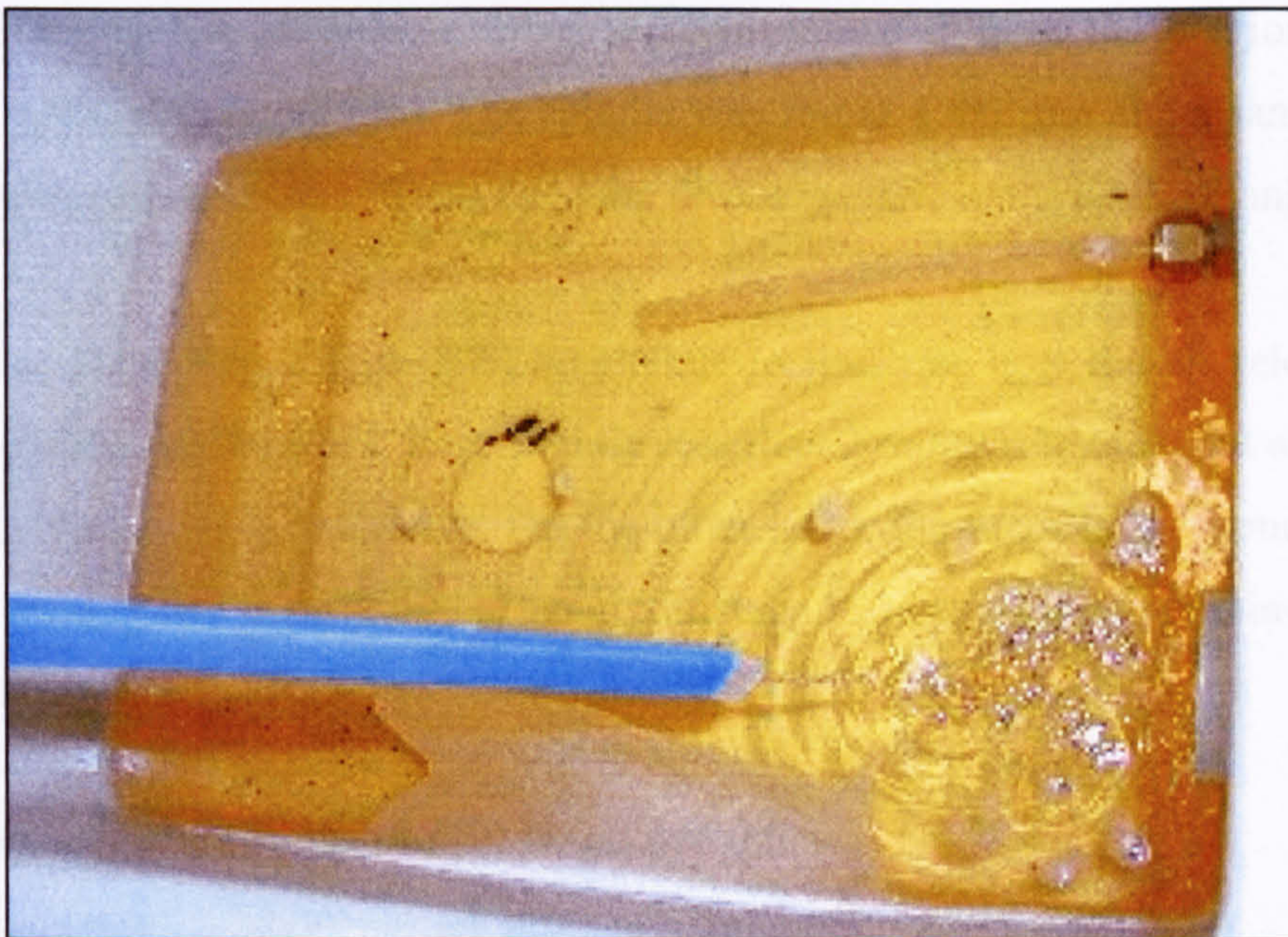
Figure 107- Settling tank after 3h operation at 3500 rpm, without air flowing to the seals.
