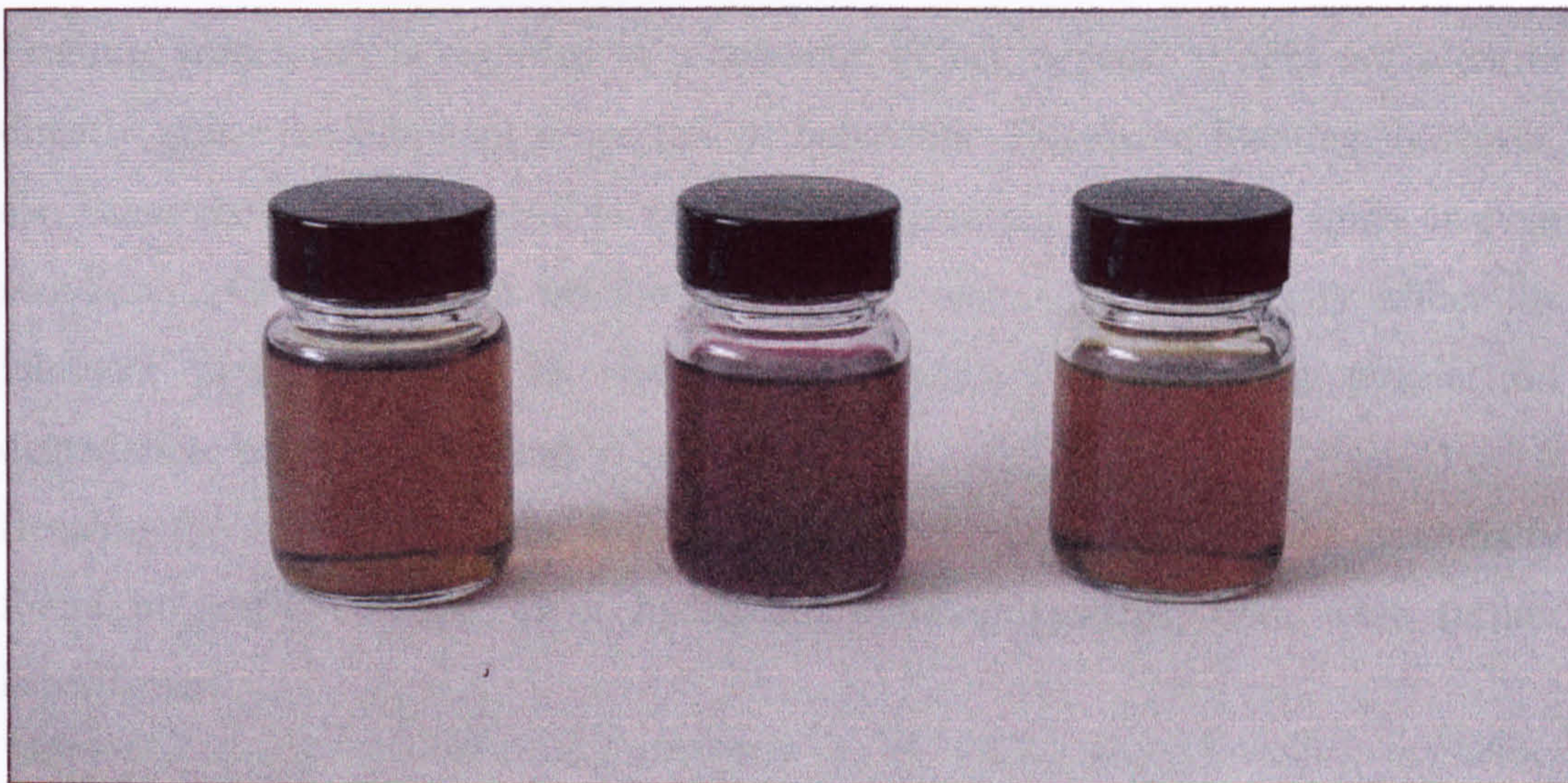
Figure 30-Inhibitors used for the corrosion testing. From left to right: Dowell, Nalco 2536 and Thaumakool.
