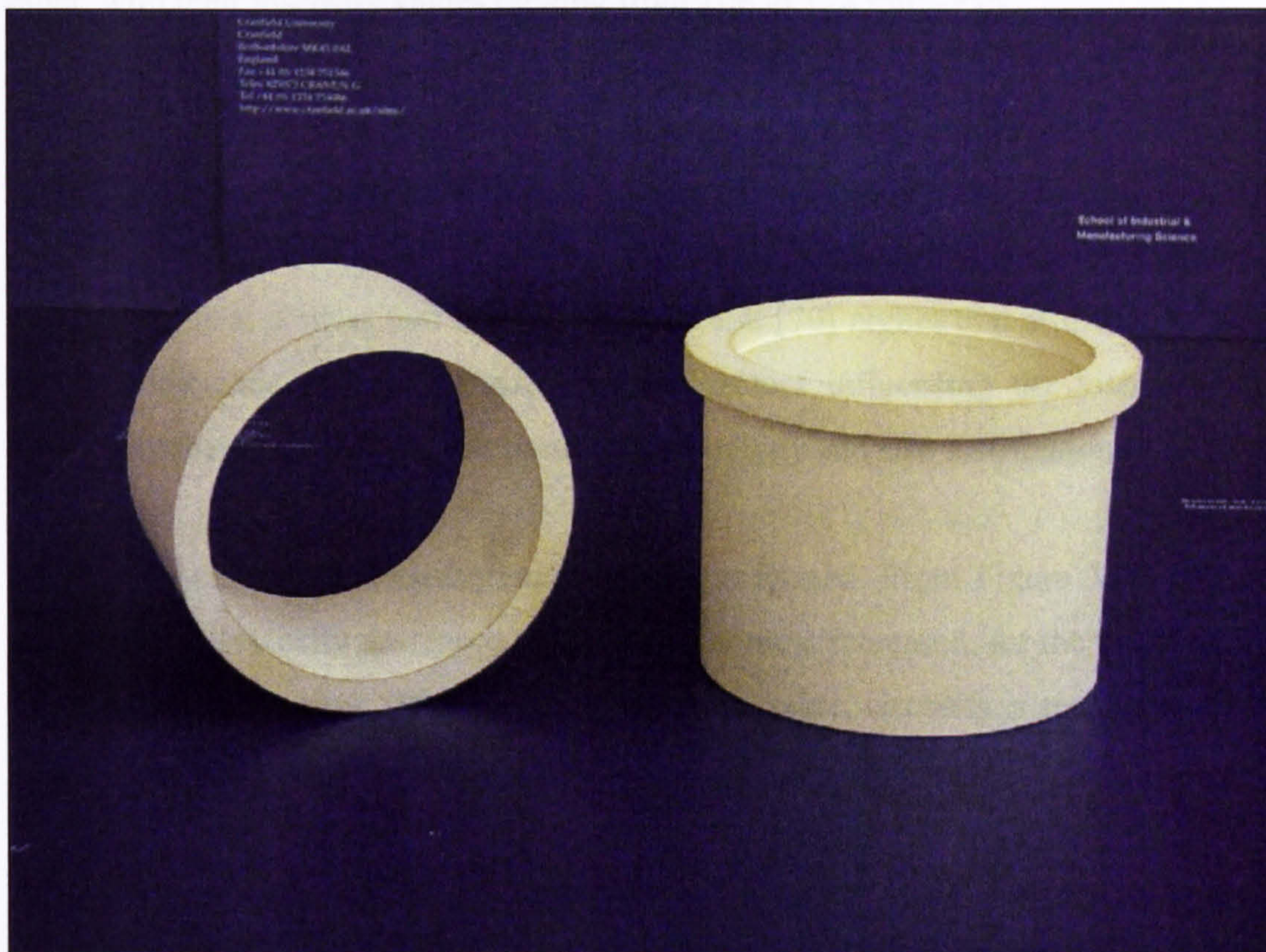
Figure 36- Larger bearings manufactured via the SC technique. Journal to the left dimensions: ID of 80 mm, OD of 96 mm and 62 mm long. Journal to the right dimensions: 85 mm ID, a 101mm OD and 82 mm long.
