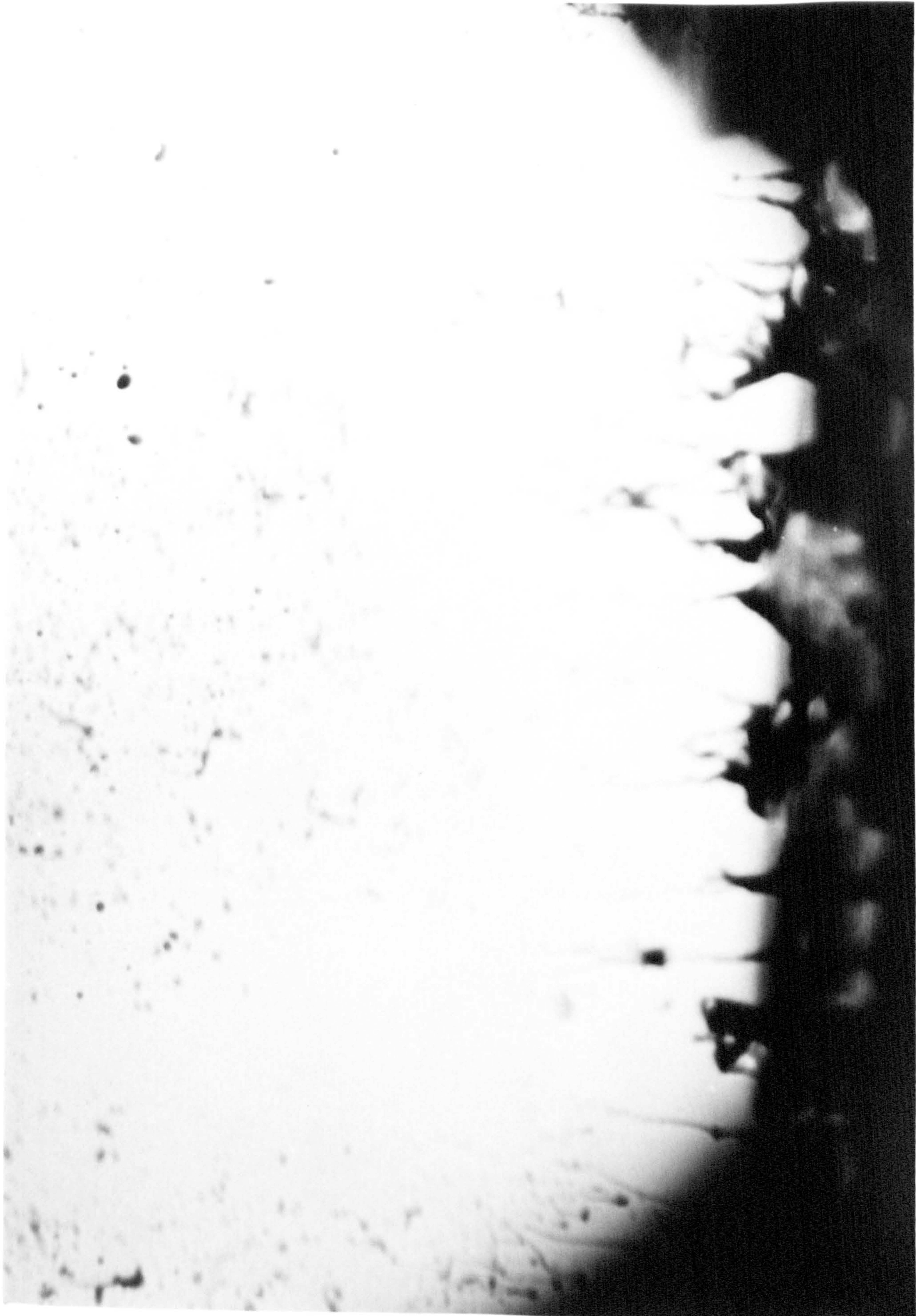
KEROSINE AIR VELOCITY = 54.9 m/s , LIQUID FLOW RATE = 4.5 gr/s
