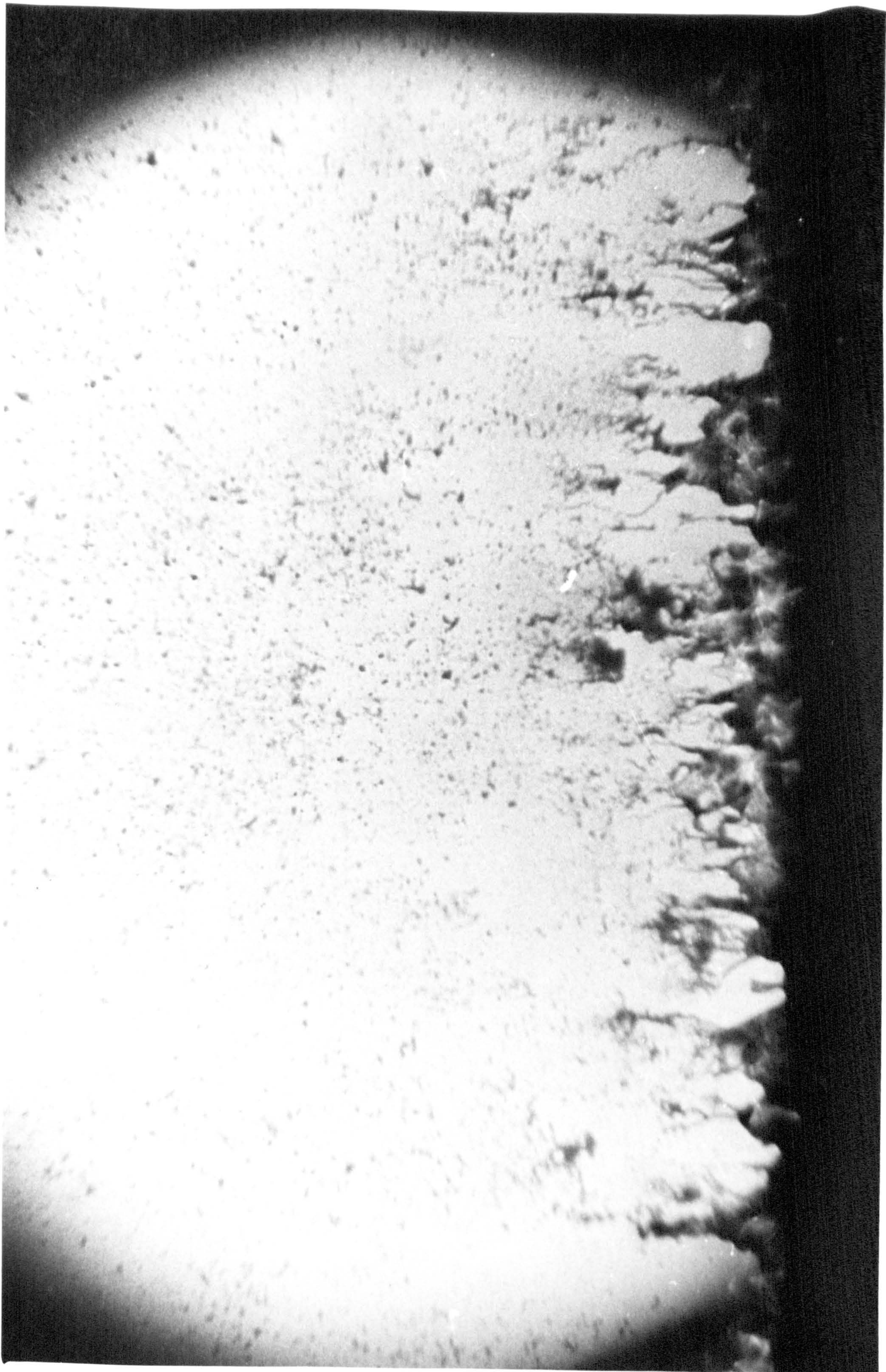
WATER AIR VELOCITY = 120 m/s , LIQUID FLOW RATE = 13.6 gr/s
