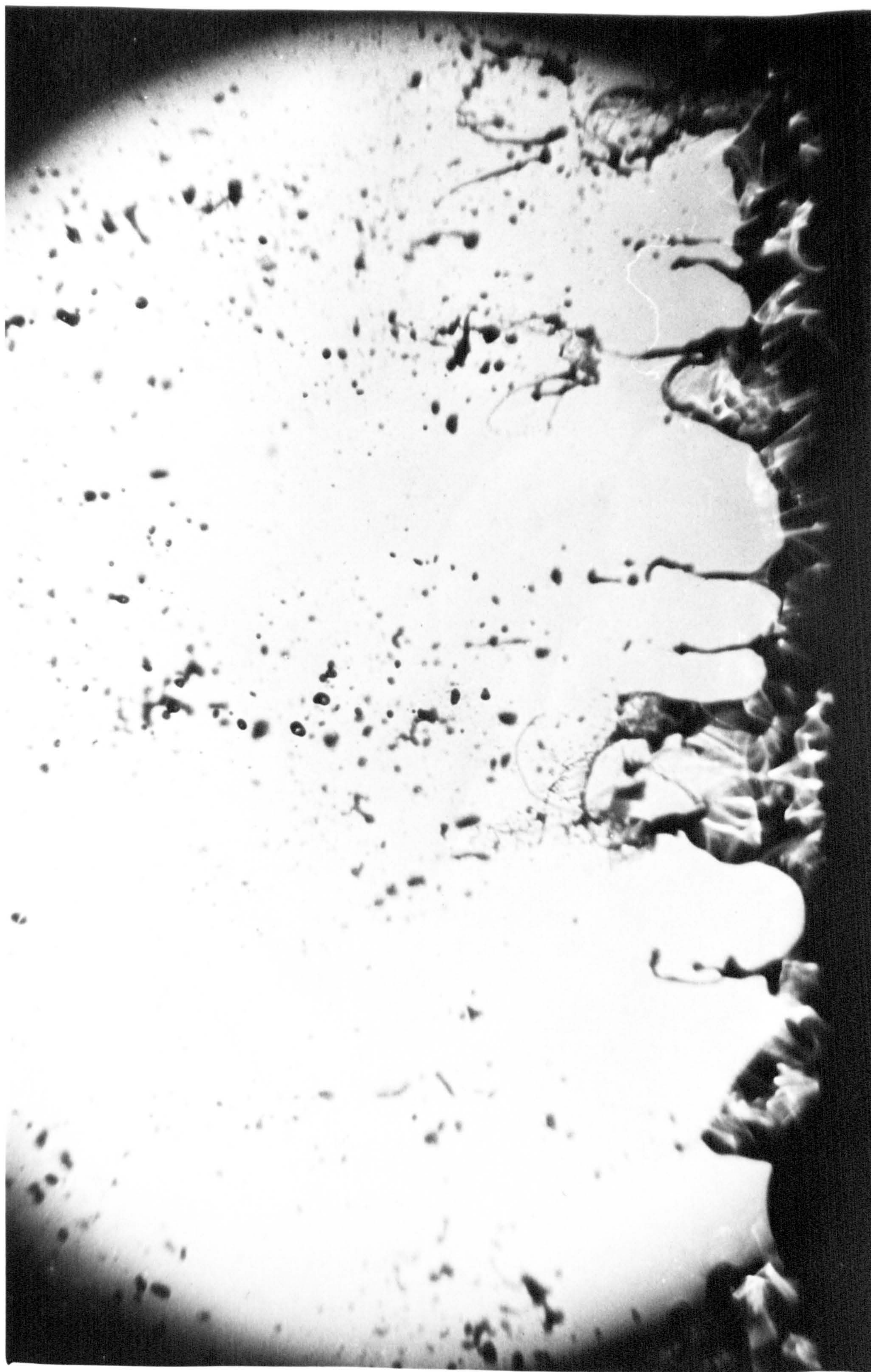
WATER AIR VELOCITY = 54.9 m/s , LIQUID FLOW RATE = 9 gr/s
