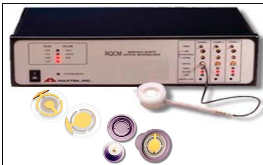
Fig 3.7 RQM Real-Time Crystal Frequency, Mass and Conductance Measurement Analyser, research crystals and crystal holder.
