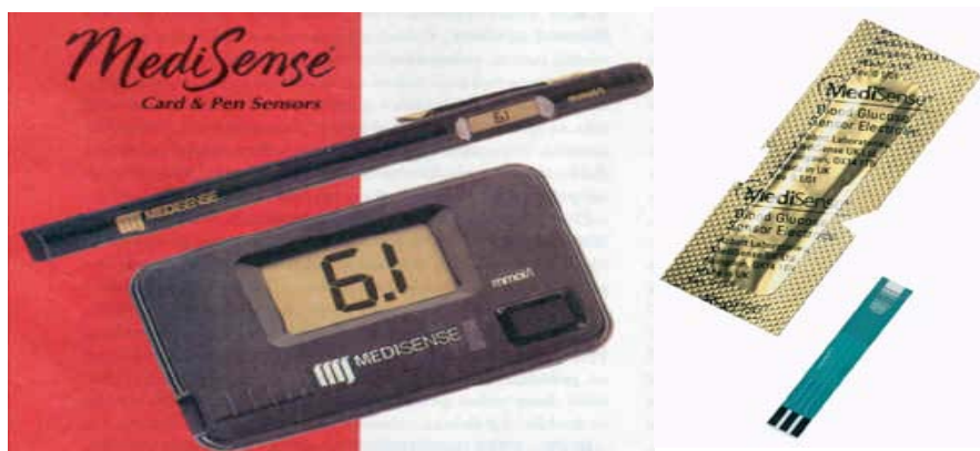
Fig 2.3 MediSense pen and credit card shaped glucose meters along with the disposable strips.
