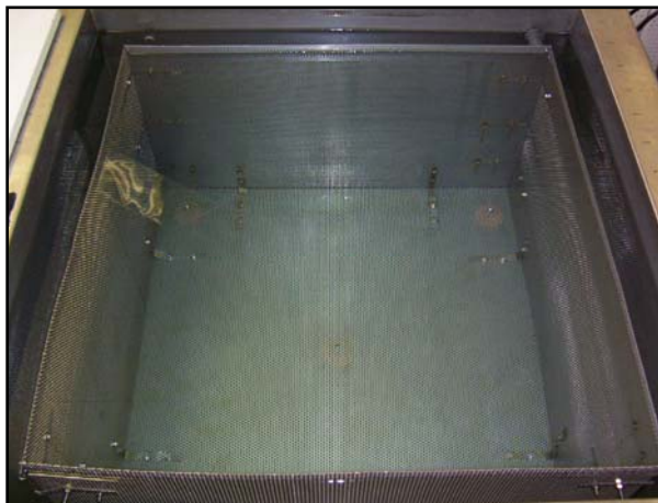
Fig 3.6 Sonication tank baffling.
