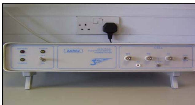
Fig 3.2 Sycopel Scientific AEW2-10 Potentiostat.
