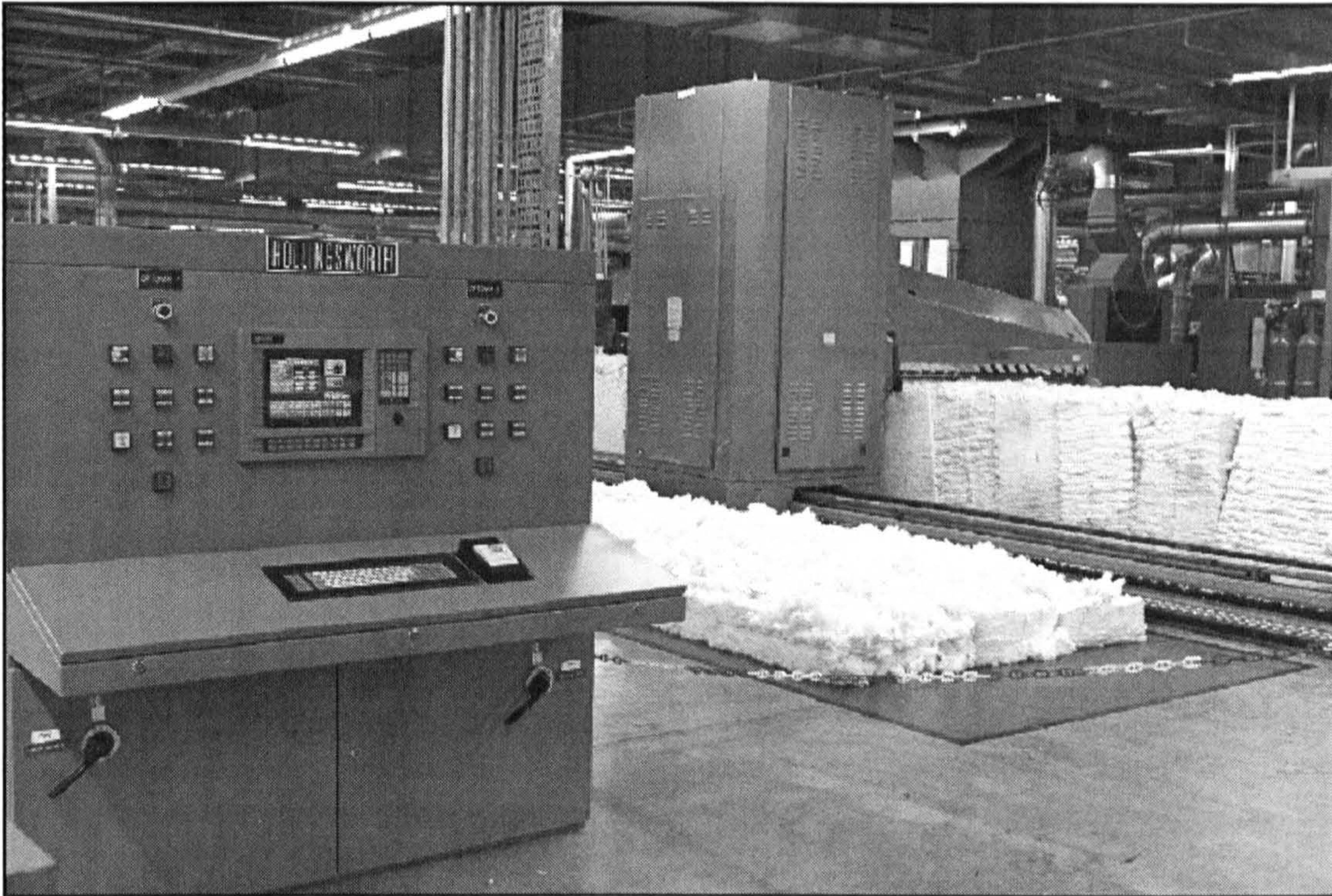
Figure 1.3: The first stage in the manufacturing process, the cleaning of cotton fibre.
