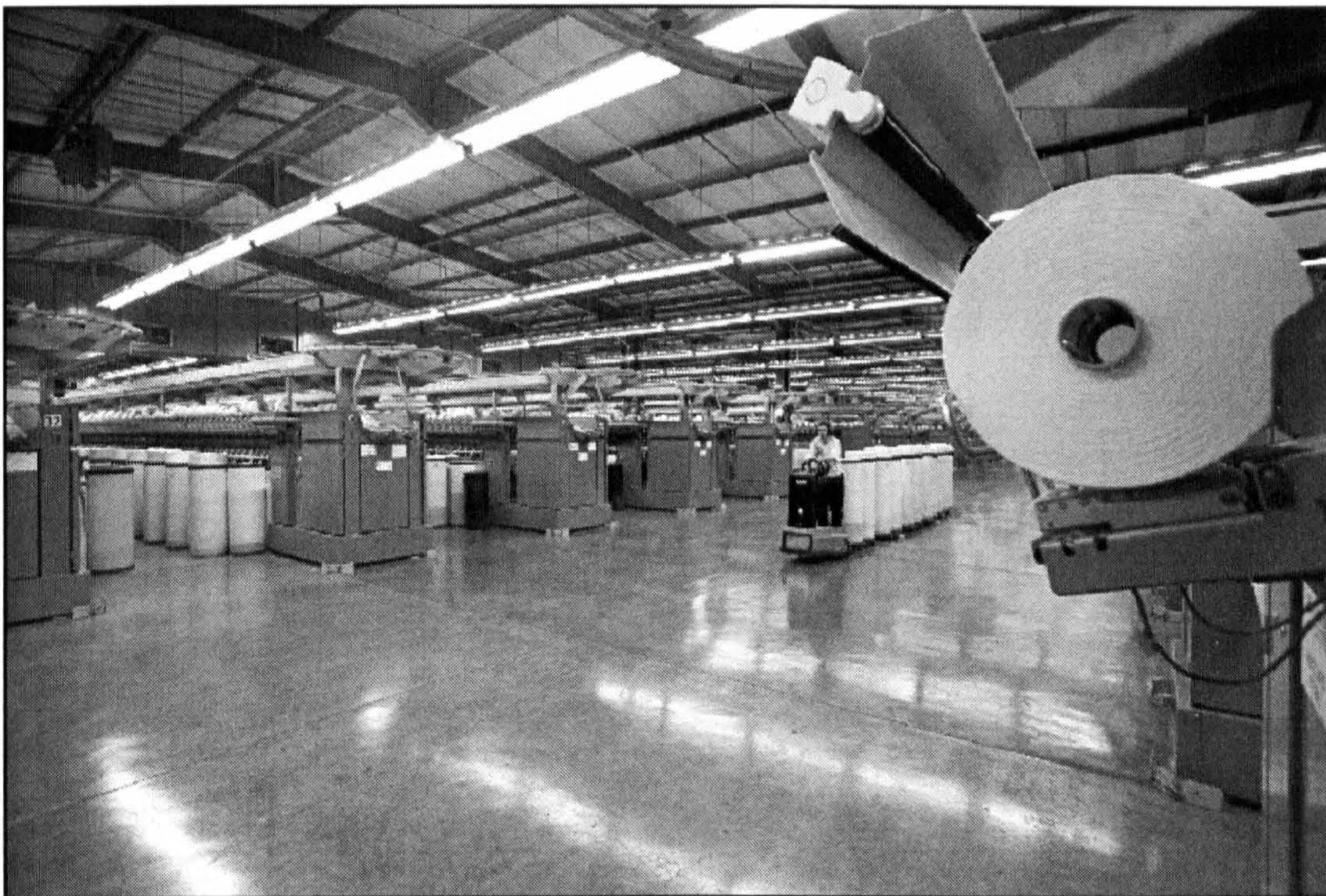
Figure 1.4: Some of the 51 spinning machines used to form yarn at the Campsie Mill in N.Ireland.
