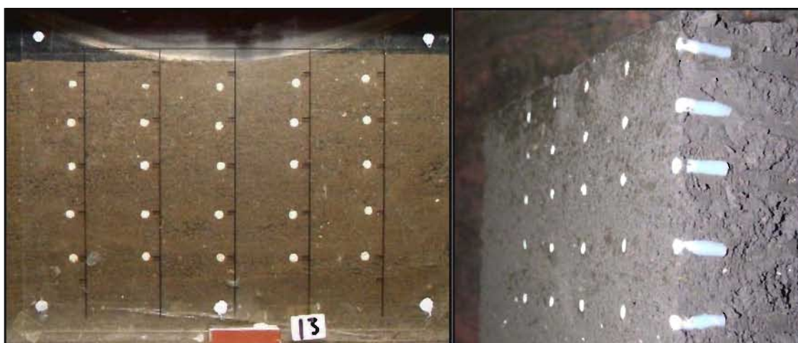
Figure 7.5 Rolling simulator side viewing window (left) showing grid of 25 markers embedded in OL soil. 5 mm diameter plastic markers, 20 mm long were inserted into the soil during preparation of the profile. Right hand picture was taken after a rolling experiment and shows no change in horizontal orientation of the marker after compaction despite vertical displacement.
