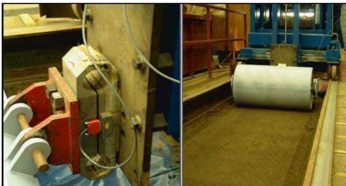
Figure 4.6 Roller mounted on a strain gauge (left) to measure force and being towed in the soil bin at Cranfield University, Silsoe by the soil bin processor (right).
