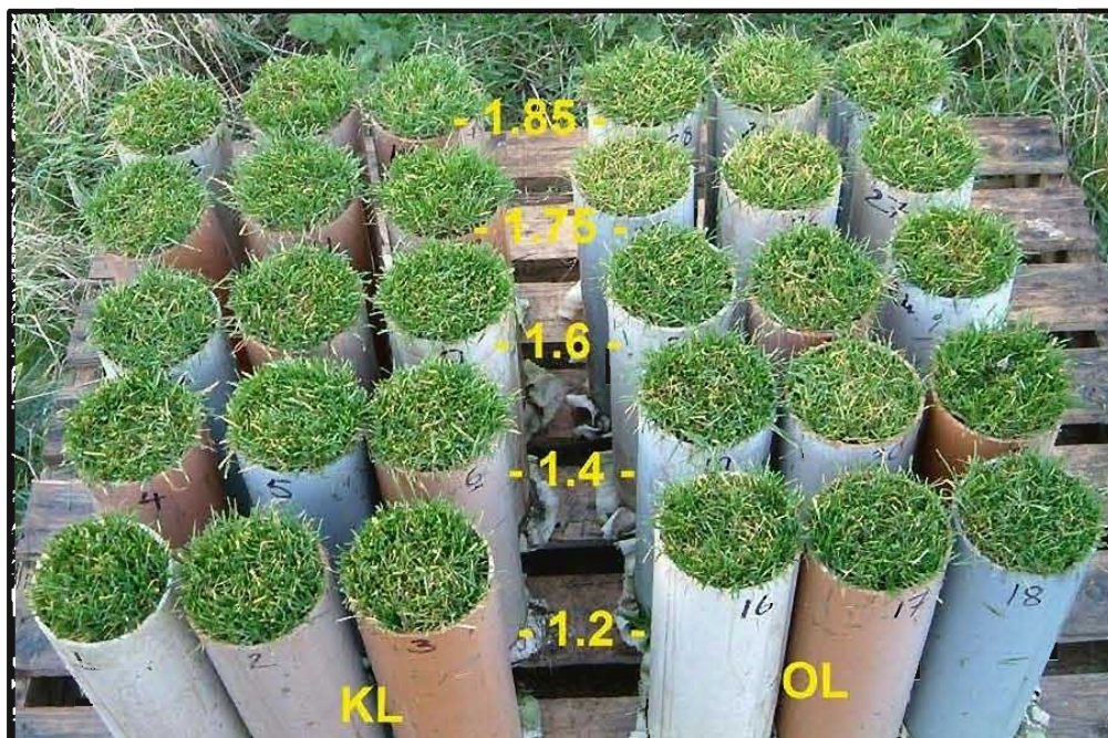
Figure 6.15 A range of root experiment treatments with KL (left) and OL (right) March 2007. OL soil showed visual signs of stressed grass growth compared to KL particularly with the higher dry bulk density treatments.
