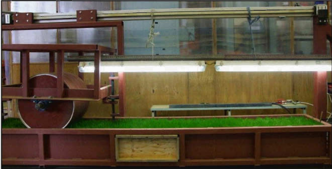
Figure 7.3 Cricket rolling simulator with grass growing in the soil bin. The grass was initially grown outside from September 2007 until experimental work was undertaken in May 2008. Growth was maintained whilst inside using 'daylight' florescent tubes to ensure grass plant health whilst target experimental moisture content was achieved (25%). Note that the wooden panel was replaced with a glass window and that grass height was reduced to 5 mm during testing.
