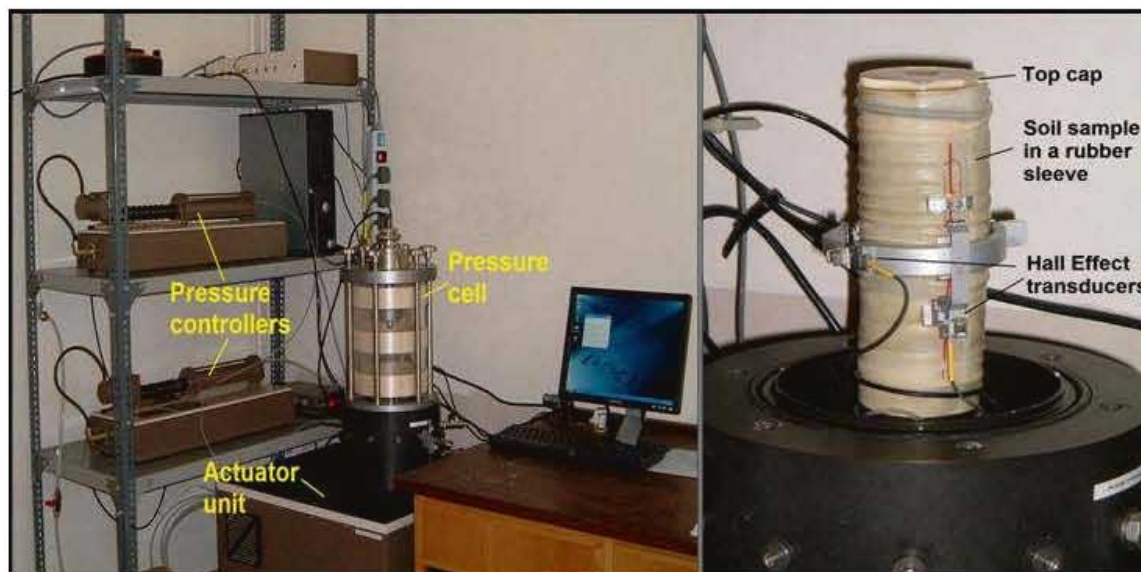
Figure 4.2 GDS Minidyn 2Hz DYNTTS equipment (left) Prepared sample for dynamic testing with Hall Effect local strain transducers measuring radial and lateral movement.
