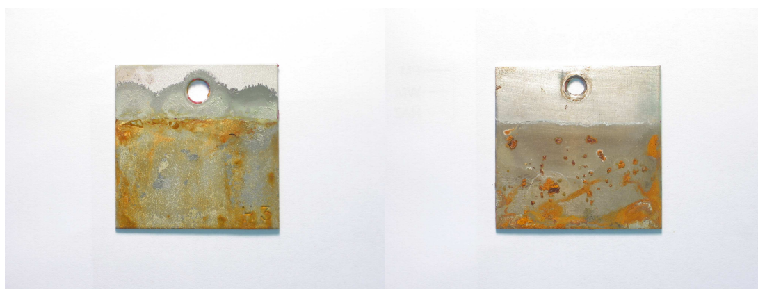
Figure 53 Appearance of 984 and steel panels after ten days of testing. Coated panel on the left and steel panel on the right
