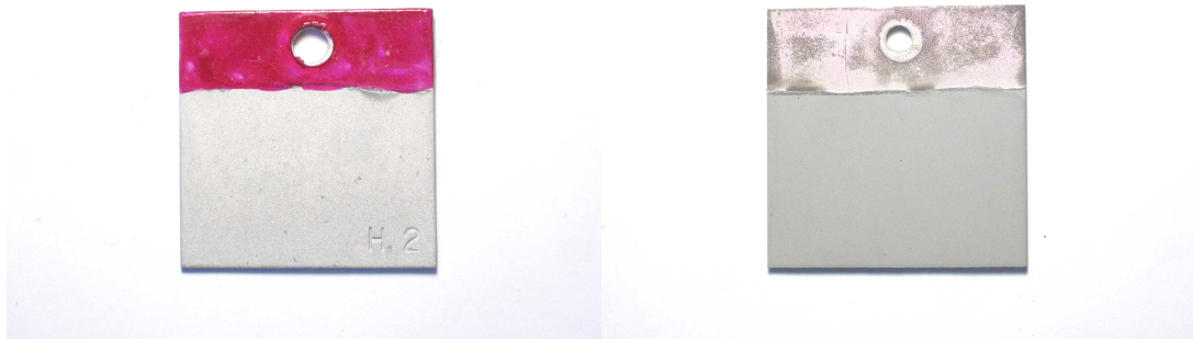
Figure 14. Appearance of unmodified 984 on the left and Cd electroplated on the right. Tested for ten days in naturally aerated 3.5% NaCl solution
