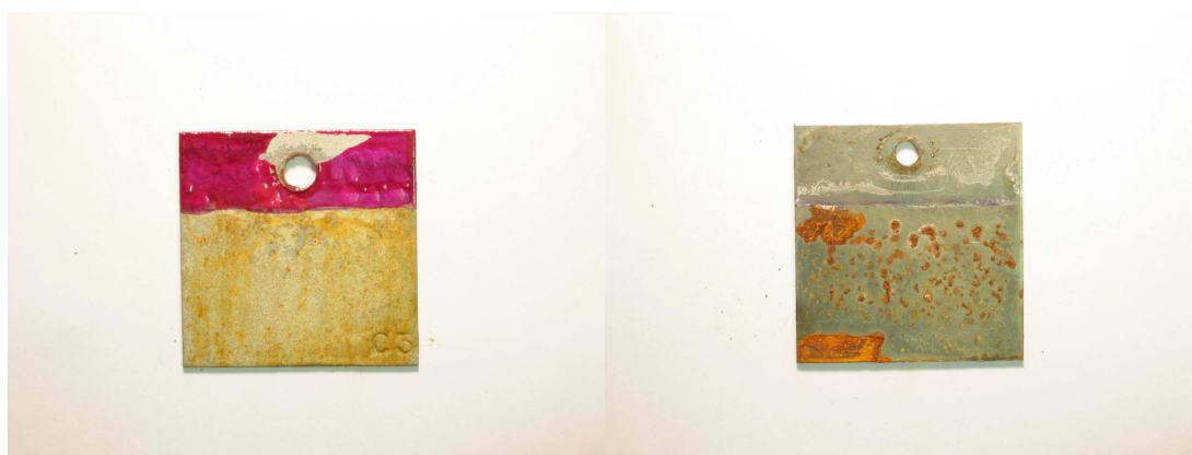
Figure 38. Appearance of 3% Zn 984 and steel panel after ten days of testing. Coated panel on the left and steel panel on the right
