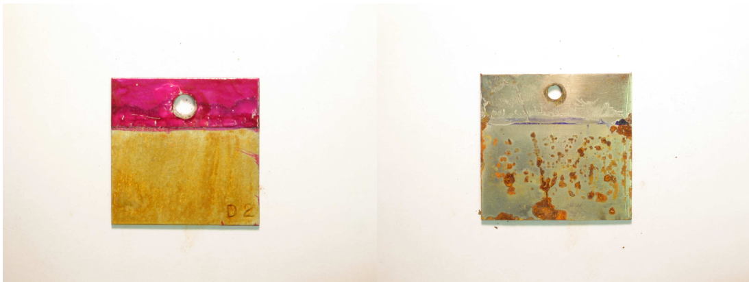
Figure 41. Appearance of 0.5% Zn 984 and steel panels after ten days of testing. Coated panel on the left and steel panel on the right
