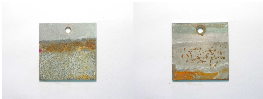
Figure 62 Appearance of IVD2 and steel panels after ten days of testing. Coated panel on the left and steel panel on the right
