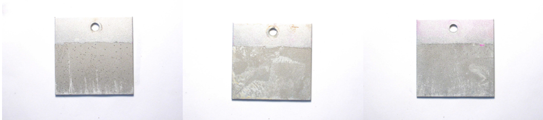
Figure 29. Appearance pure aluminium IVD1 on the left, IVD2 in the middle and IVD3 on the right. Tested for ten days in naturally aerated 3.5% NaCl solution
