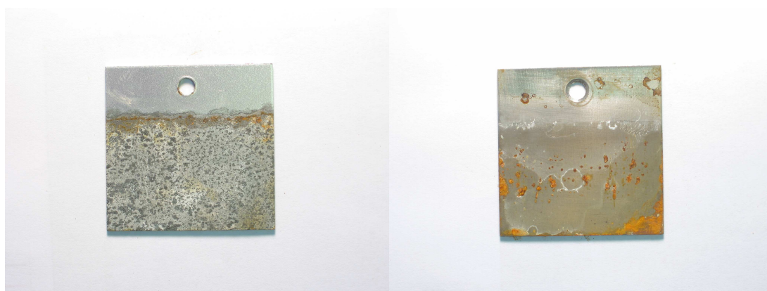
Figure 59 Appearance of IVD1 and steel panels after ten days of testing. Coated panel on the left and steel panel on the right
