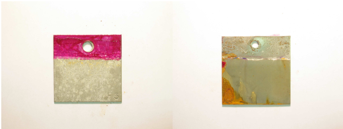
Figure 47. Appearance of 30% Mg 984 and steel panels after ten days of testing. Coated panel on the left and steel panel on the right
