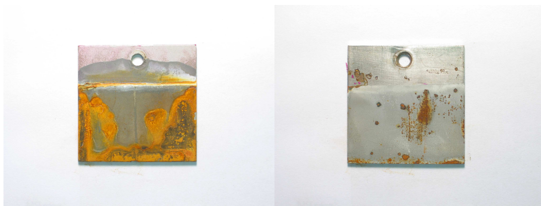
Figure 68 Appearance of Cd and steel panels after ten days of testing. Coated panel on the left and steel panel on the right
