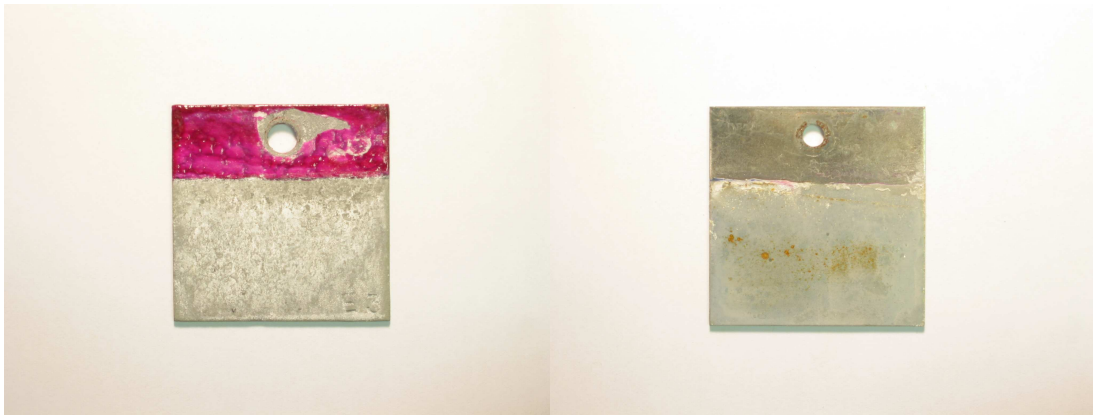
Figure 44. Appearance of 50% Mg 984 and steel panels after ten days of testing. Coated panel on the left and steel panel on the right
