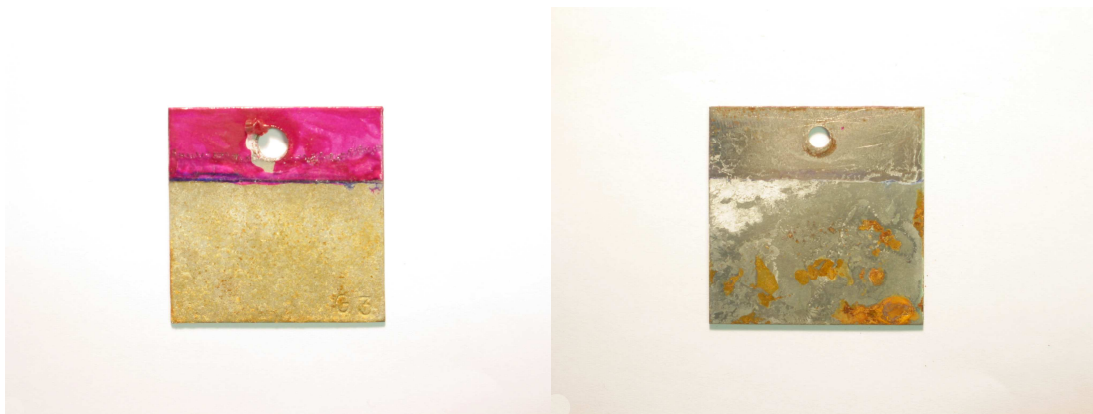
Figure 50. Appearance of 7075 and steel panels after ten days of testing. Coated panel on the left and steel panel on the right
