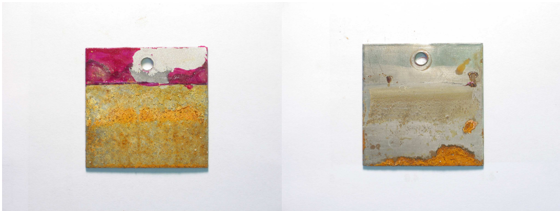
Figure 56. Appearance of 1725 and steel panels after ten days of testing. Coated panel on the left and steel panel on the right
