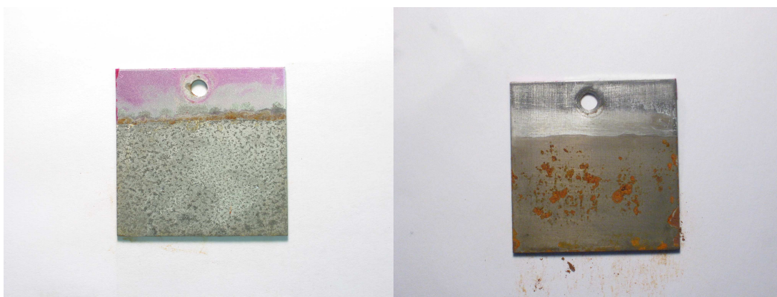
Figure 65 Appearance of IVD3 and steel panels after ten days of testing. Coated panel on the left and steel panel on the right
