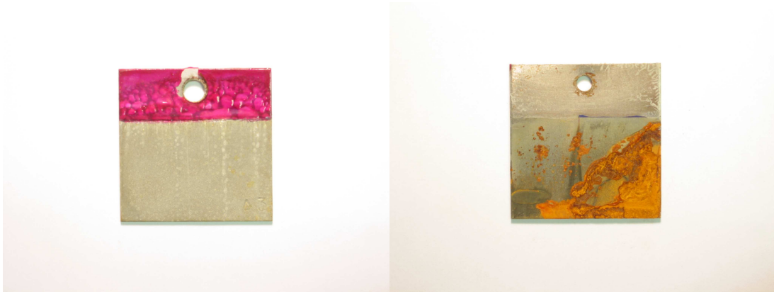
Figure 32. Appearance of 50% Zn 984 and steel panels after ten days of testing. Coated panel on the left and steel panel on the right.
