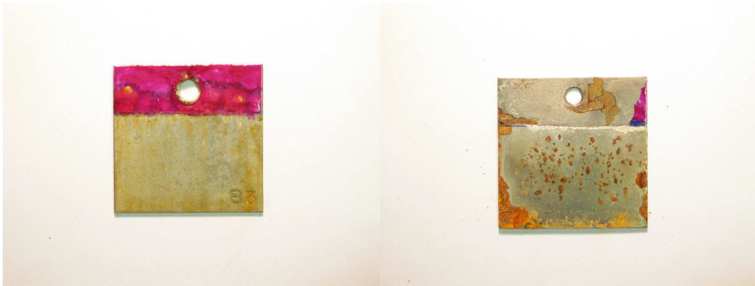
Figure 35. Appearance of 10% Zn 984 and steel panels after ten days of testing. Coated panel on the left and steel panel on the right.
